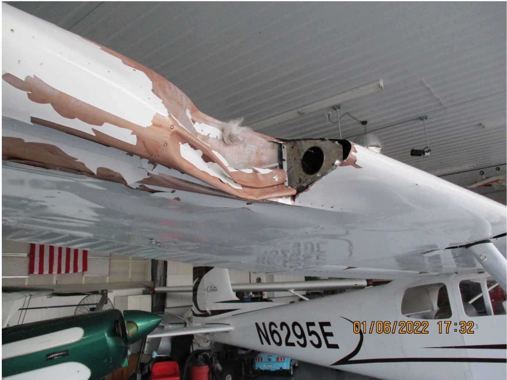
Photo 1 – Right Wing Damage (Photo Courtesy of FAA)
