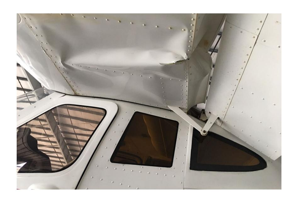
Photo 3 – Close-up View of Left Wing Damage (Photo Courtesy of FAA)
