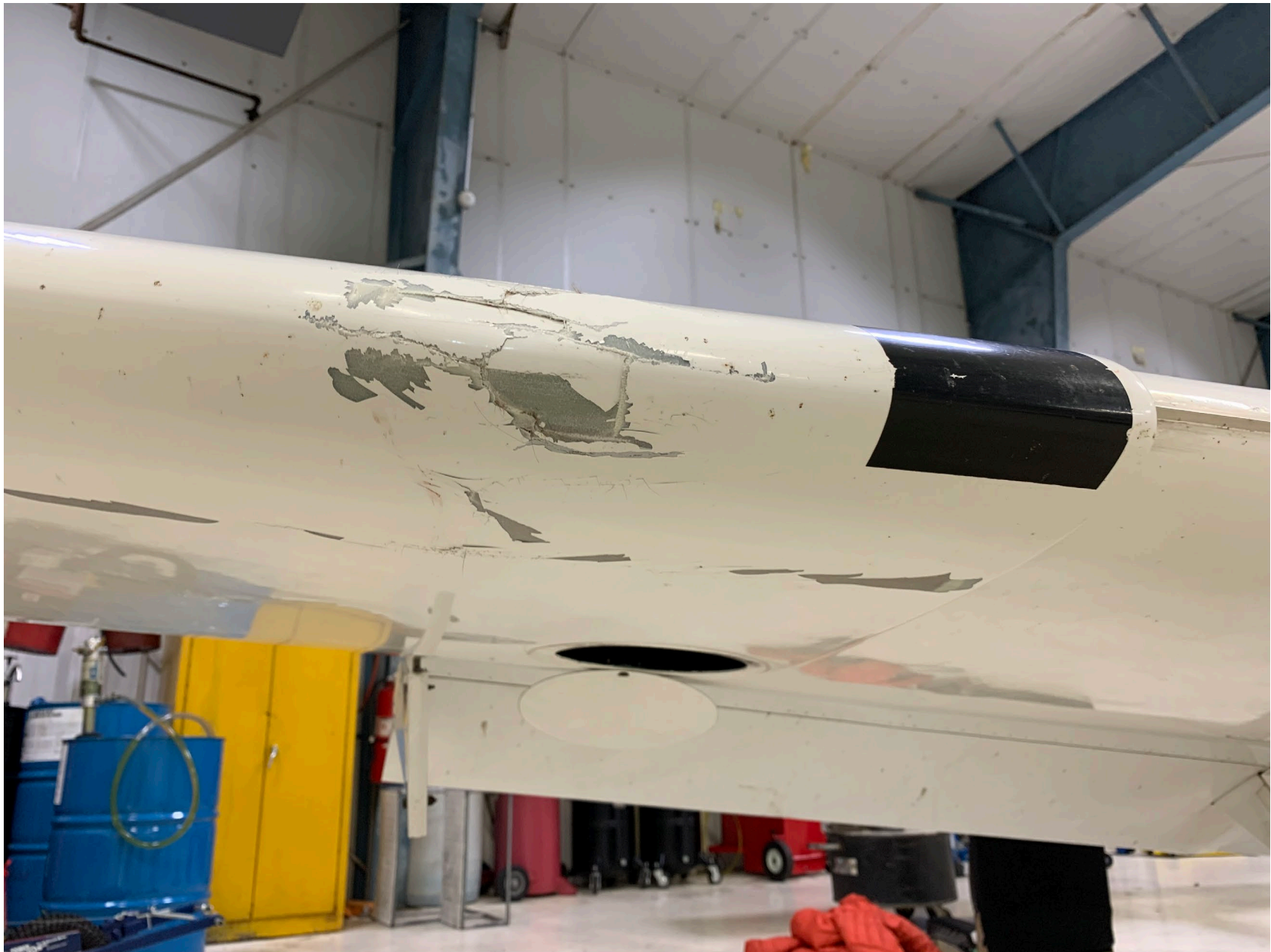
Photo 2 – Right wing and leading edge damage (photo provided by FAA)
