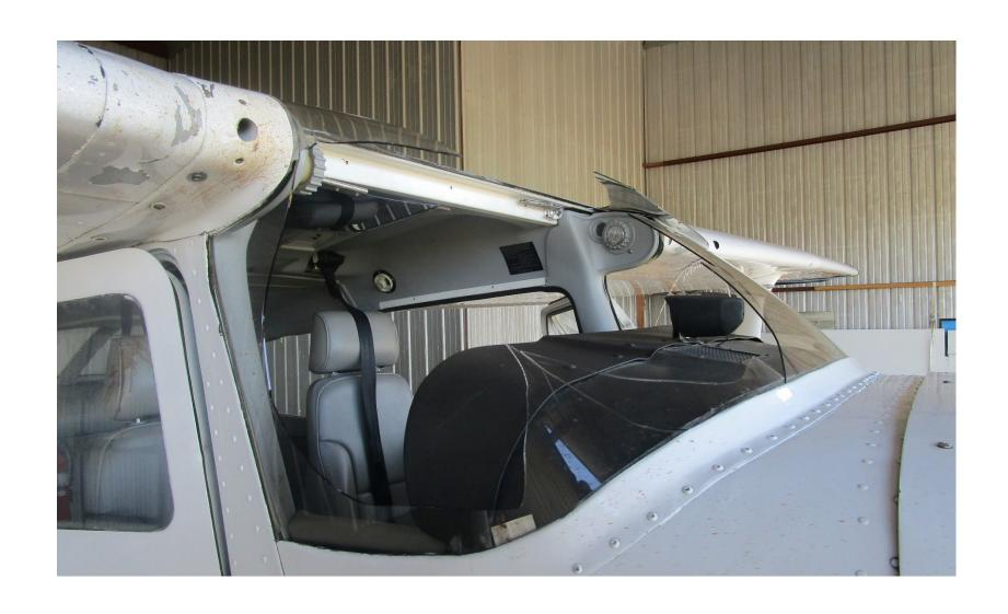
Photo 2 – View of Broken Windscreen (Photo Courtesy of FAA)
