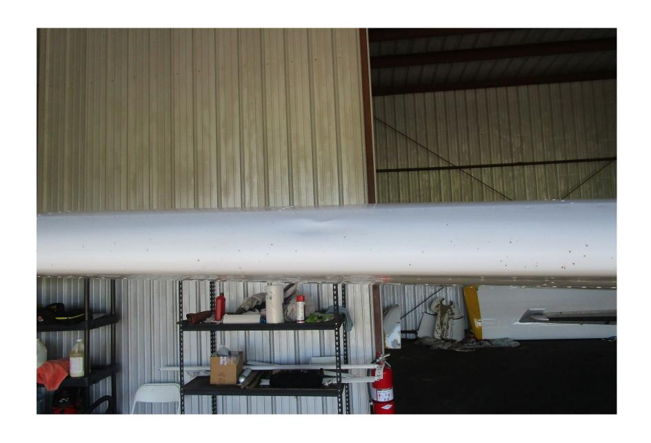
Photo 3 – View of Additional Bird Impact Damage on Right Wing (Photo Courtesy of FAA)
