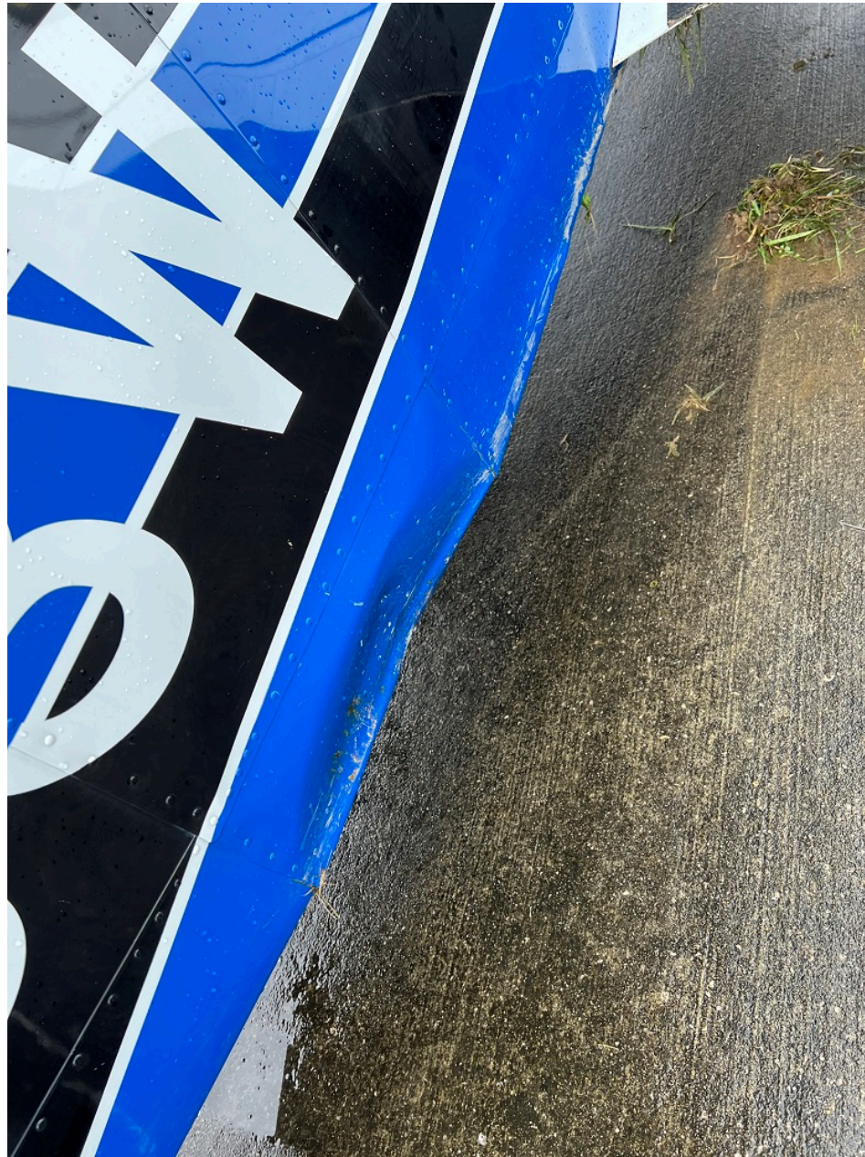
Photo 3 – Right Fuselage Damage (Photo Courtesy of FAA)
