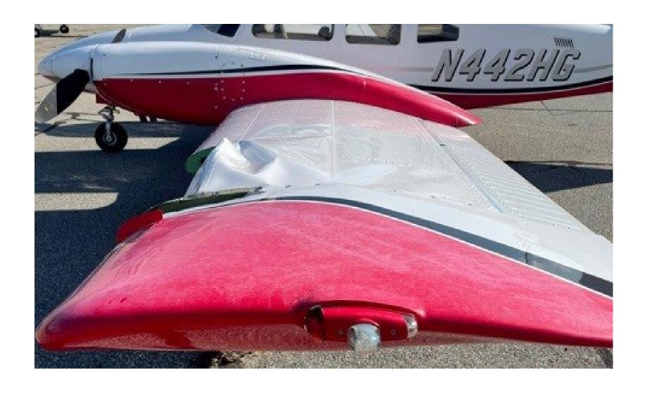
**Photo 2 – View of Wing Damage from Left Wingtip (Photo Courtesy of Pilot)**
