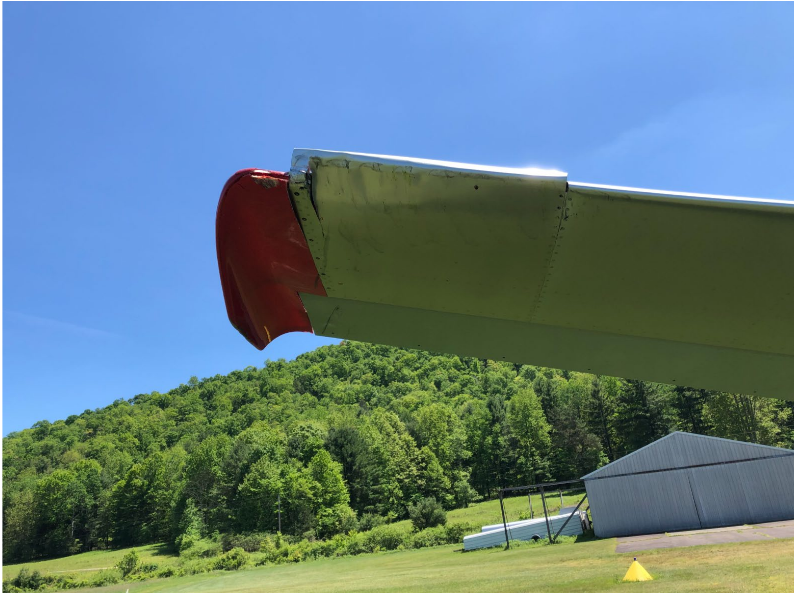
Photo 4 – Damage to Right Wingtip – Courtesy of Brokenstraw Soaring Club
