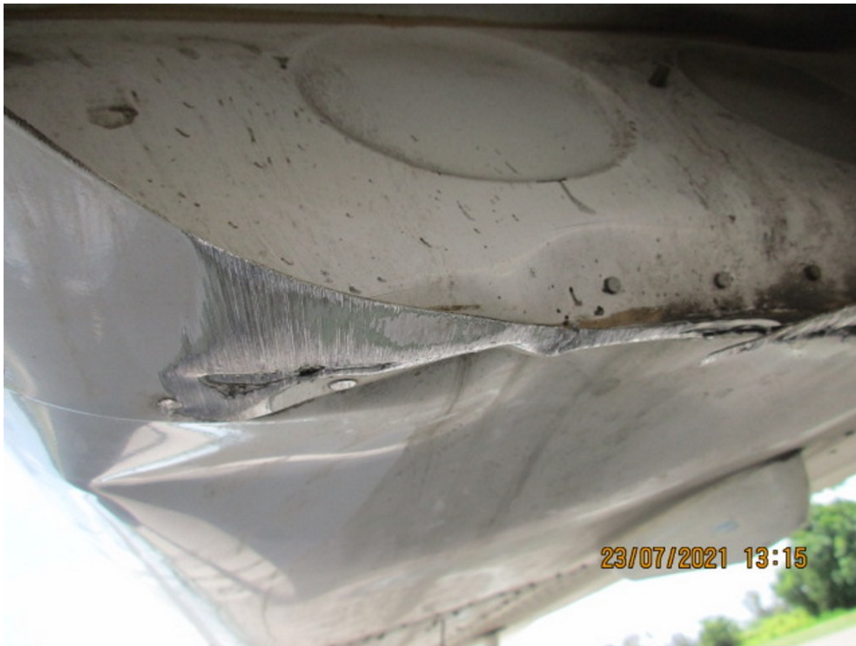
Photo 2 – Deformation of Bulkhead (courtesy FAA)
