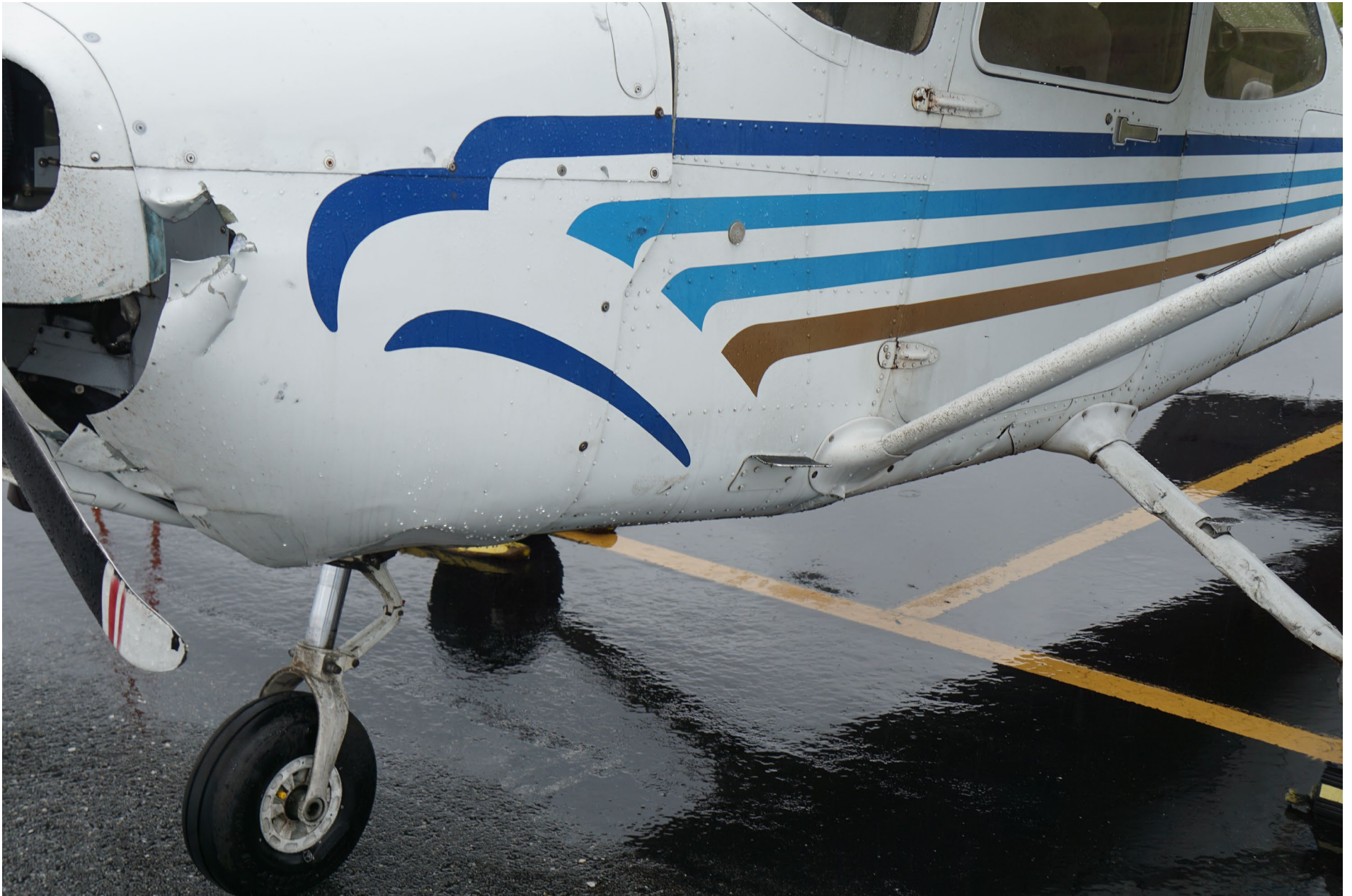
Photo 4 – Forward Fuselage Damage (FAA Photo)
