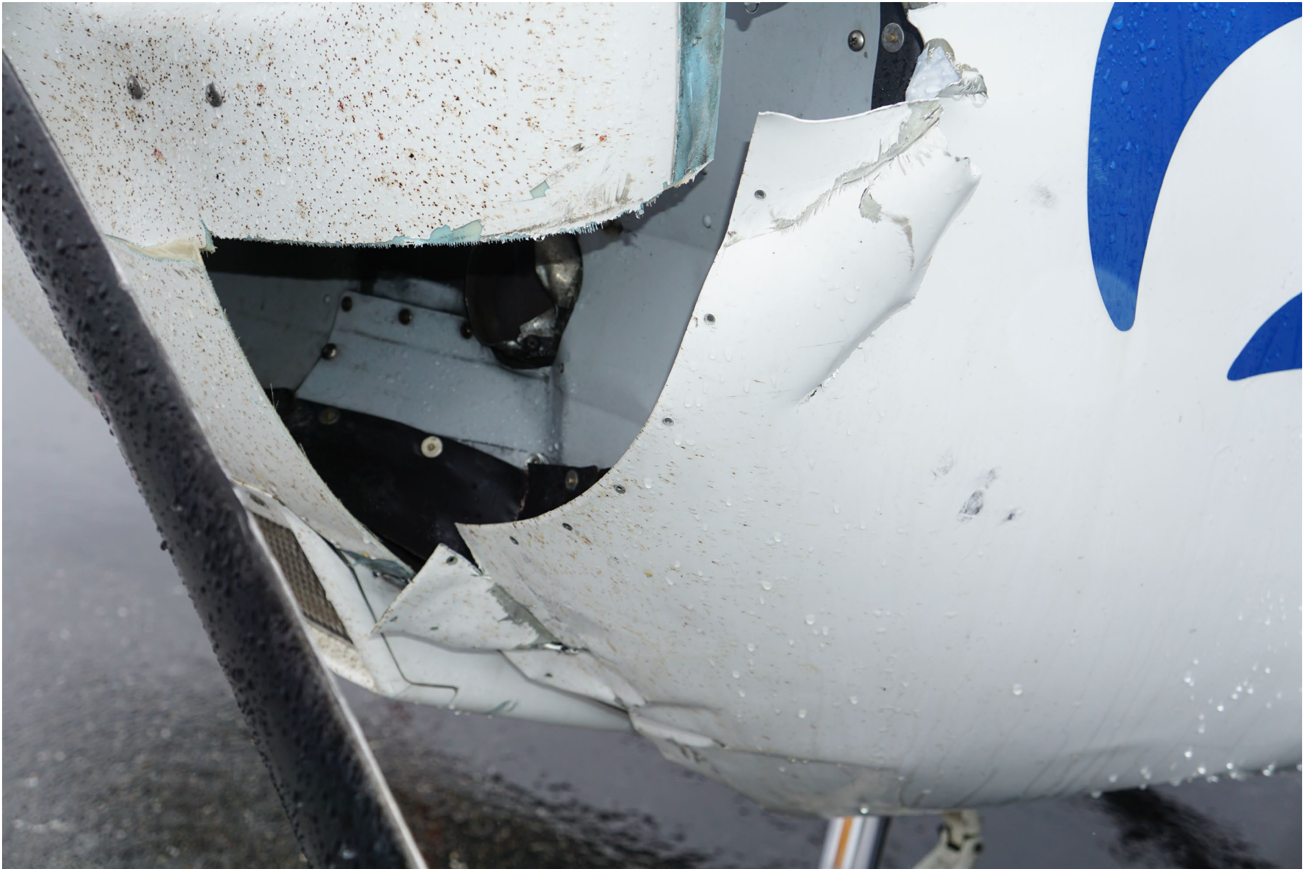
Photo 5 – Forward Fuselage Damage (FAA Photo)
