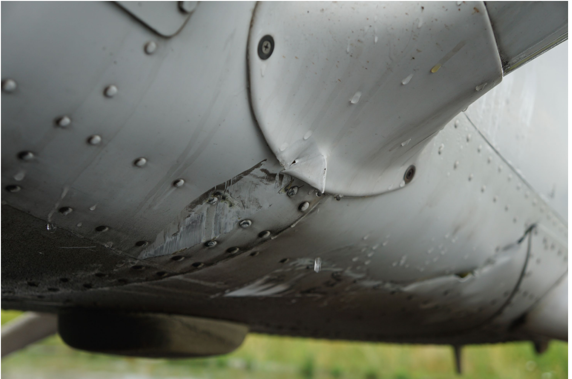
Photo 3 – Lower Fuselage Damage (FAA Photo)
