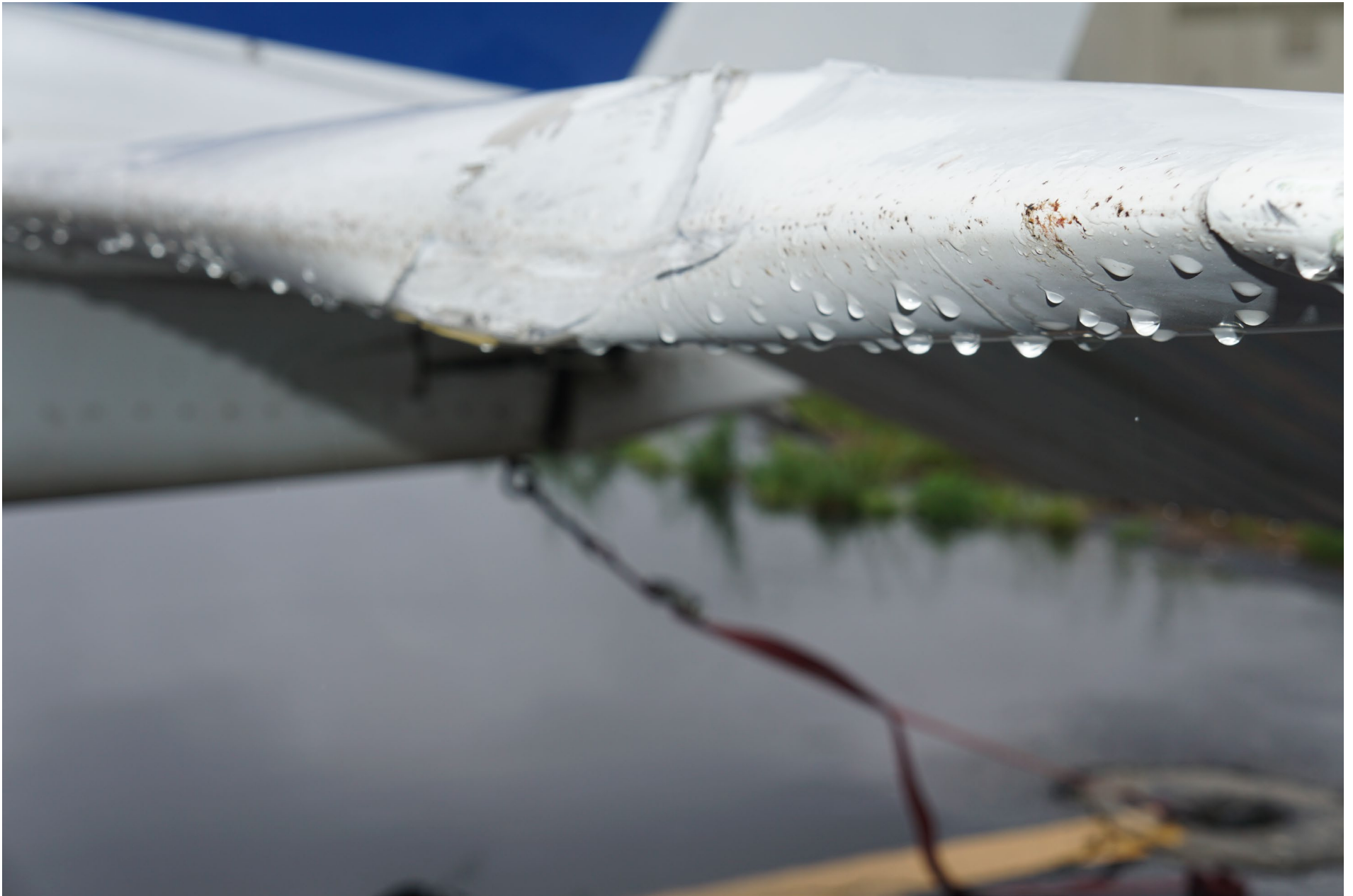
Photo 1 – Horizontal Stabilizer Damage (FAA Photo)
