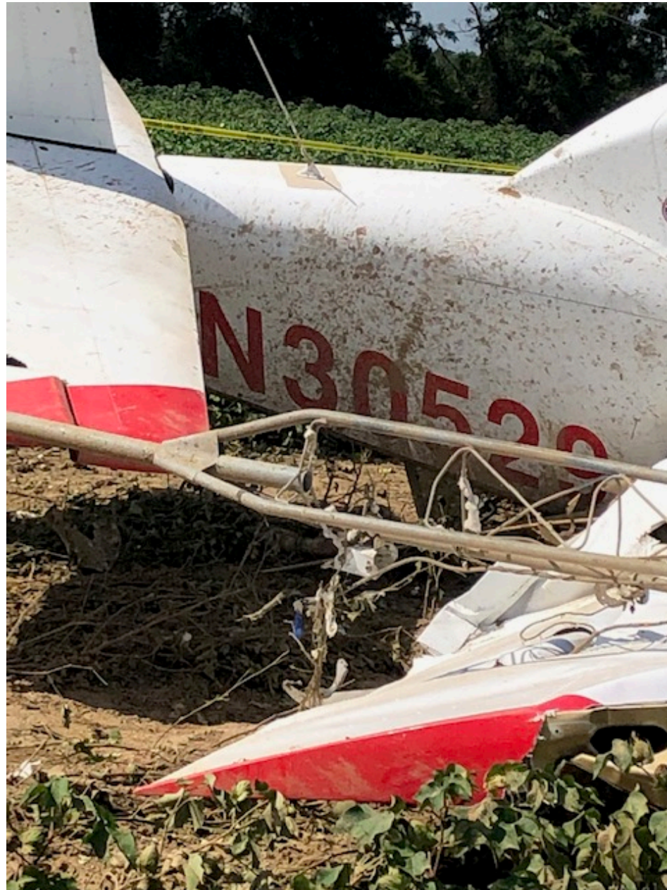
Photo 8 – Close Up of Portion of Antenna Tower Embedded in Right Wing – Courtesy of AIG
