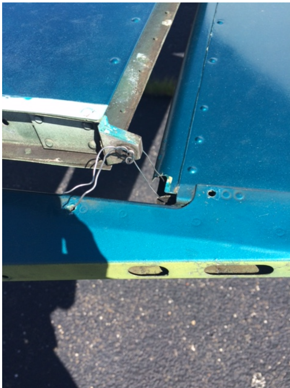
Photo 4 – Close Up of Left Elevator Hinge
