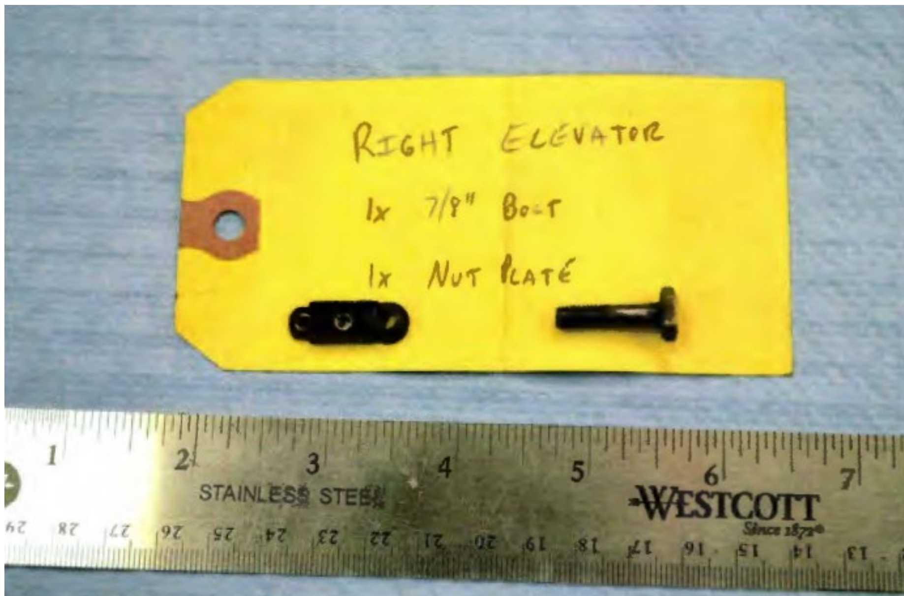
Photo 7 – Right Elevator Bolt and Nut Plate – Courtesy of FAA
