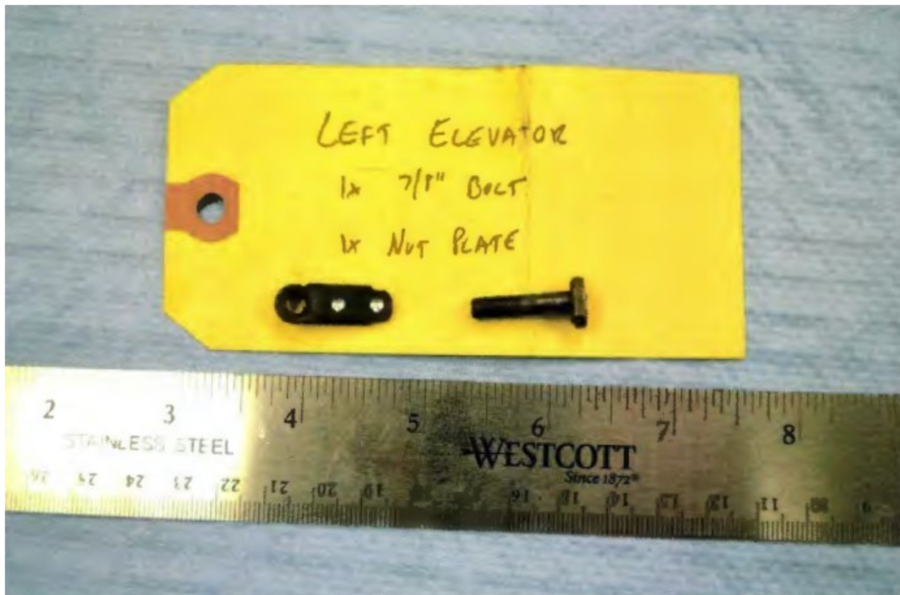
Photo 6 – Left Elevator Bolt and Nut Plate – Courtesy of FAA
