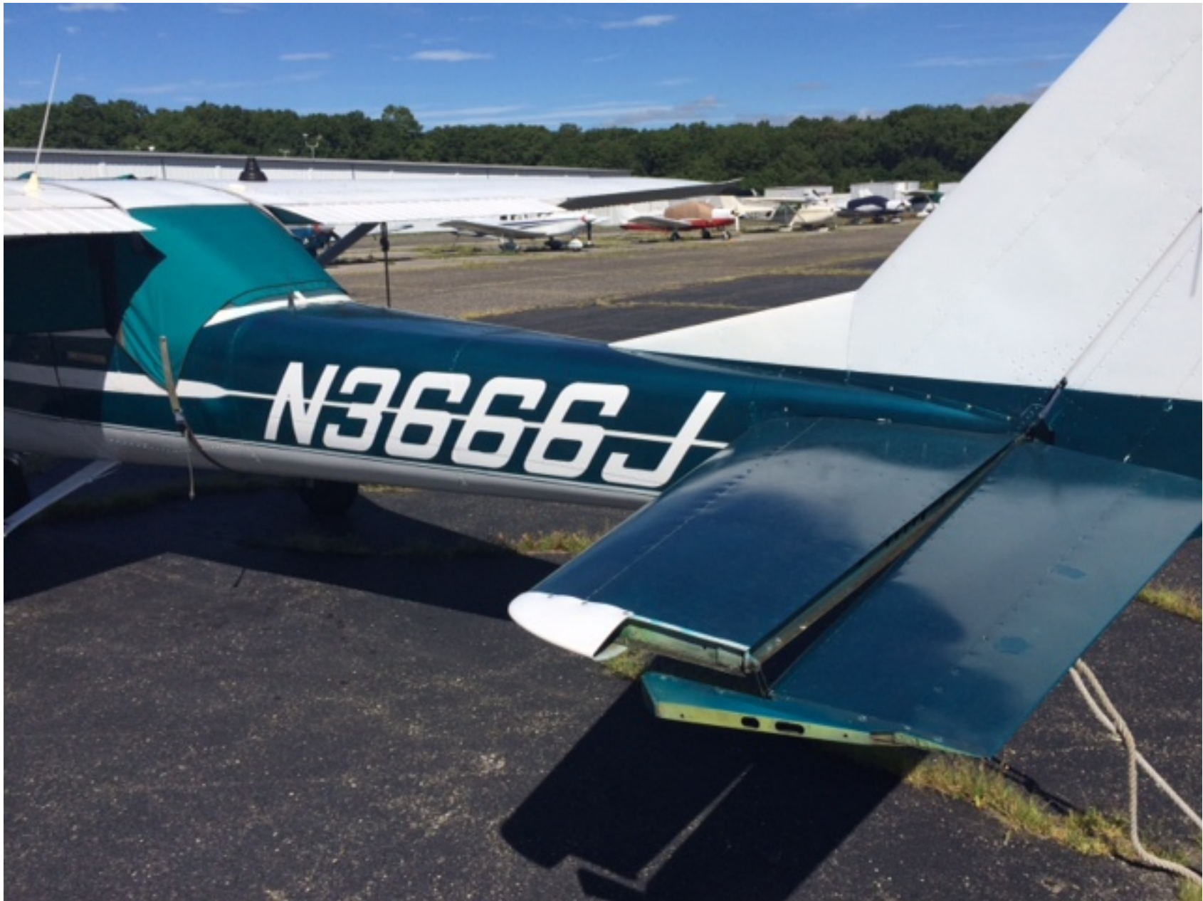
Photo 1 – Left Horizontal Stabilizer and Elevator – Courtesy of FAA
