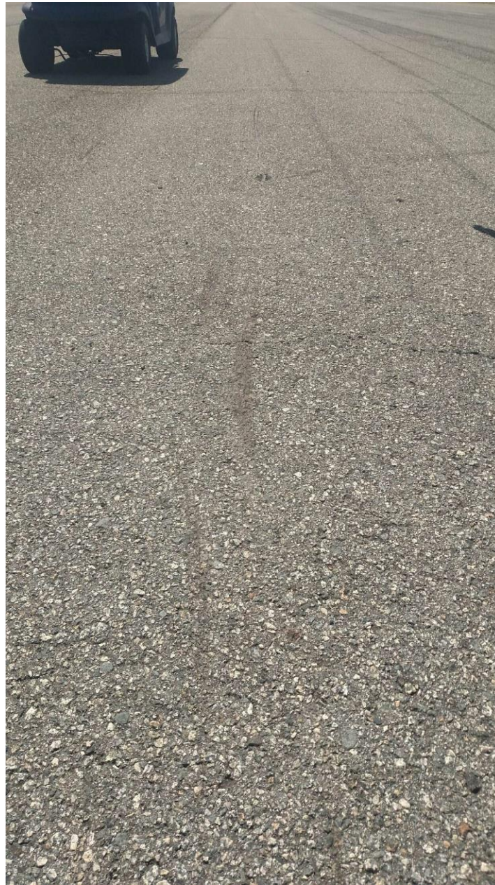
Photo 2 – Accident site, runway impact marks.
