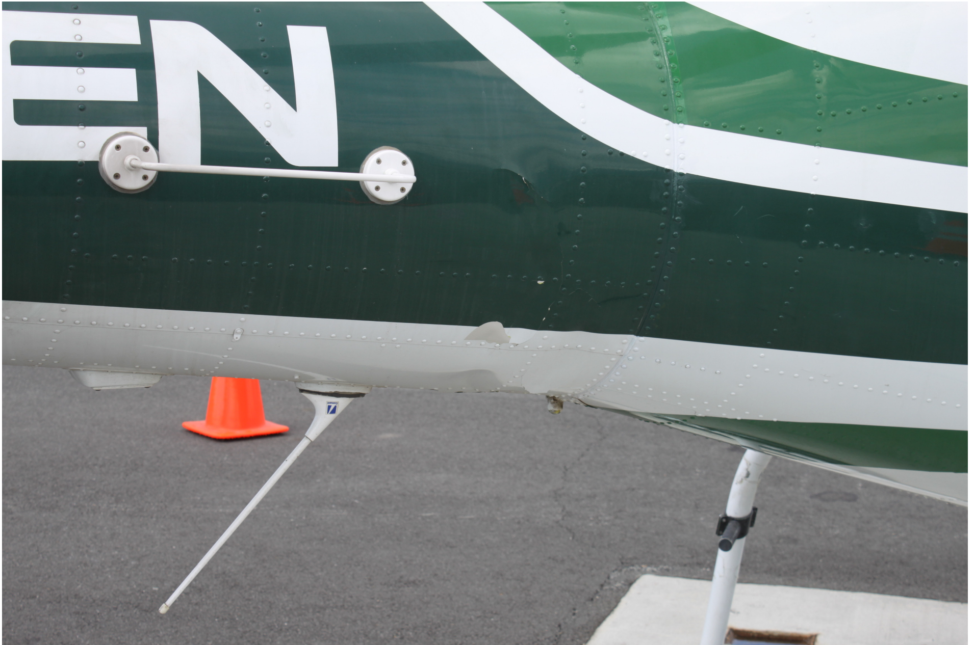
Photo 2 – Damage to Right Tail Boom Assembly
