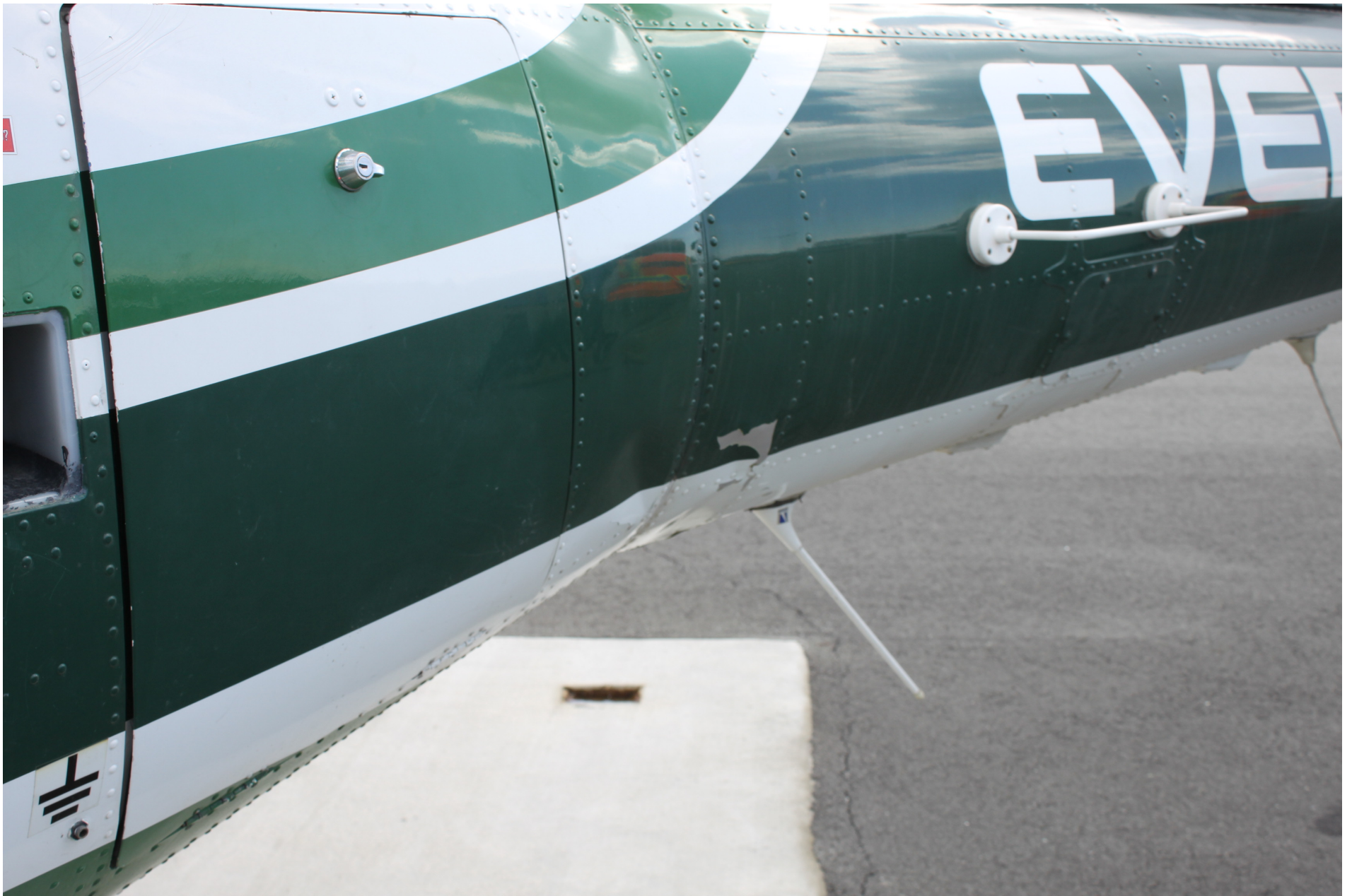
Photo 1 – Damage to Left Tail Boom Assembly
