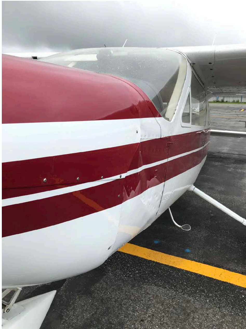
Photo 7 – Close Up of Left Side Forward Fuselage Wrinkle - Courtesy of Pittsfield Municipal Airport
