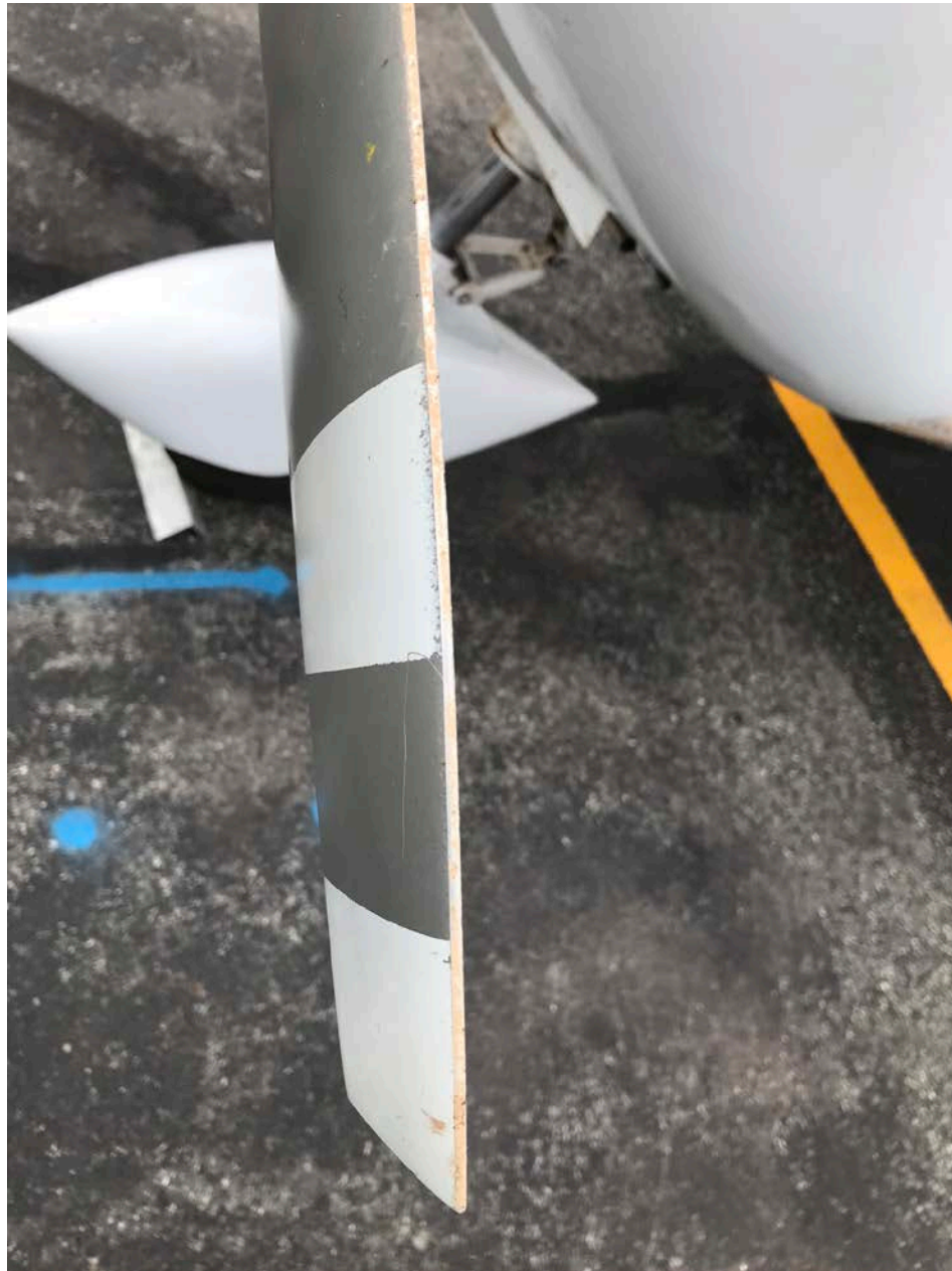
Photo 5 – Propeller Blade Showing Dirt from Ground Contact and Yellow Paint Transfer - Courtesy of Pittsfield Municipal Airport
