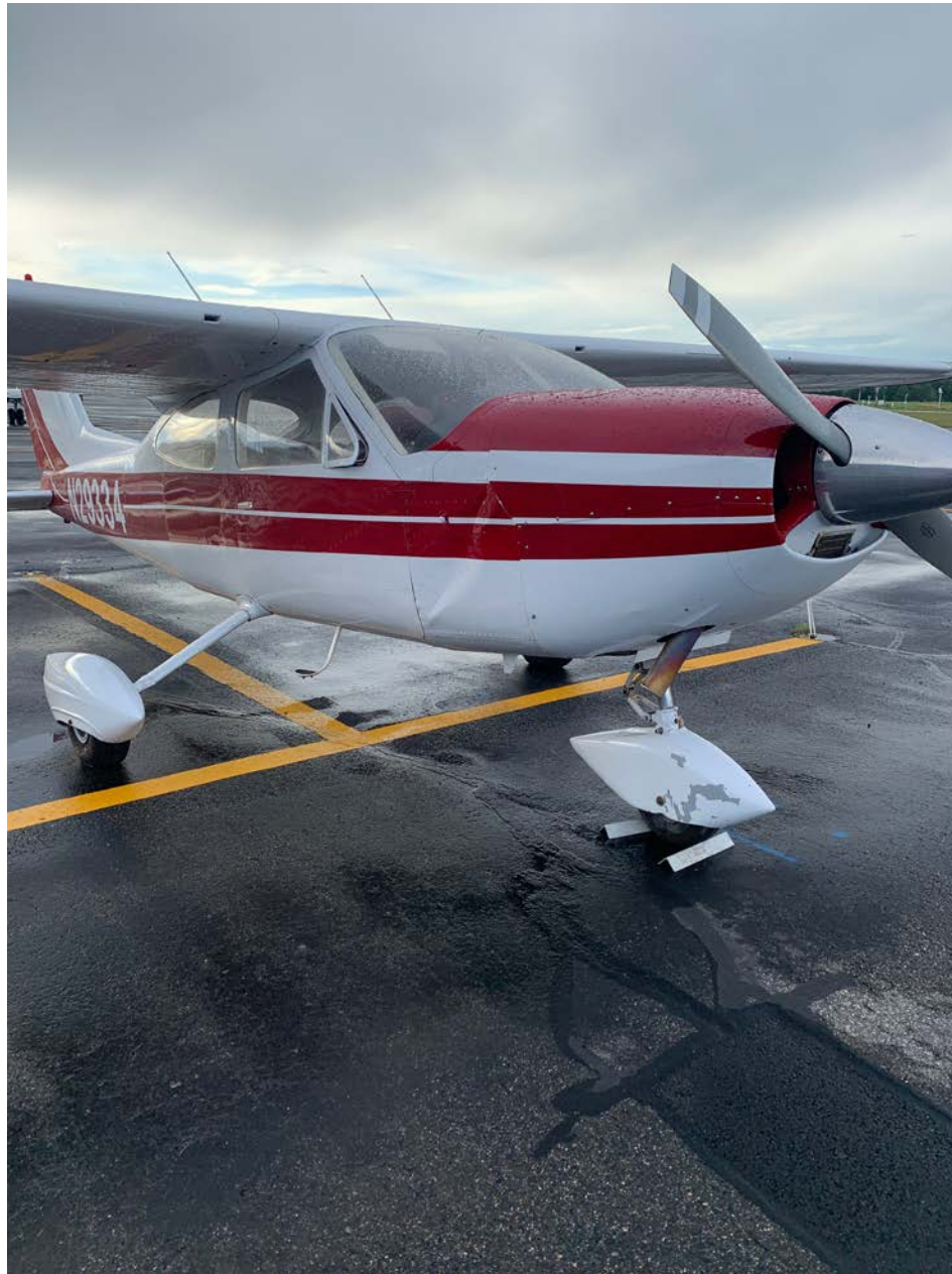
Photo 9 – Right Side of Airplane Showing Fuselage Wrinkle and Missing Paint on Nose Wheel Landing Gear Paint - Courtesy of Pittsfield Municipal Airport
