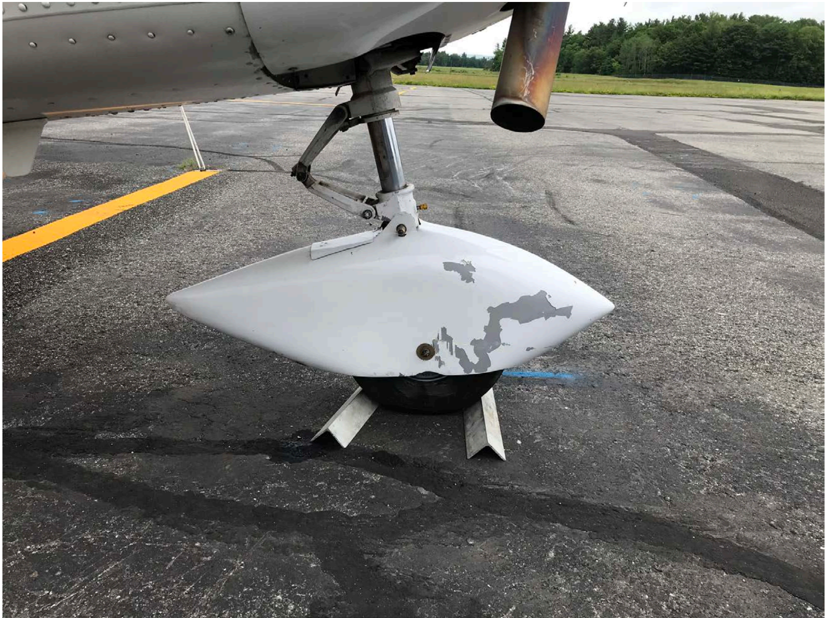
Photo 4 – Nose Wheel Landing Gear Pant Showing Missing Paint - Courtesy of Pittsfield Municipal Airport
