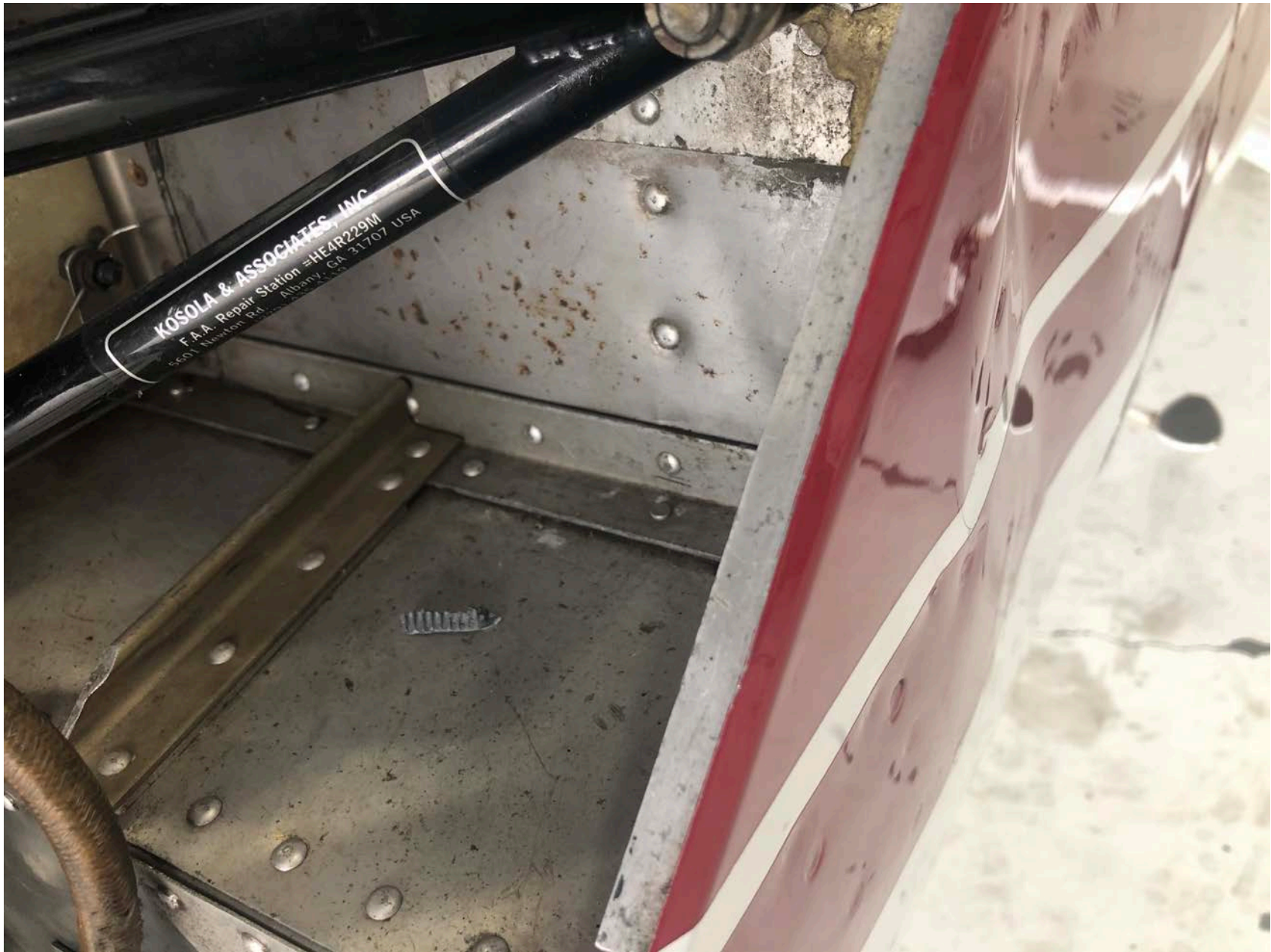
Photo 8 – Left Side Firewall and Fuselage Wrinkles - Courtesy of Pittsfield Municipal Airport
