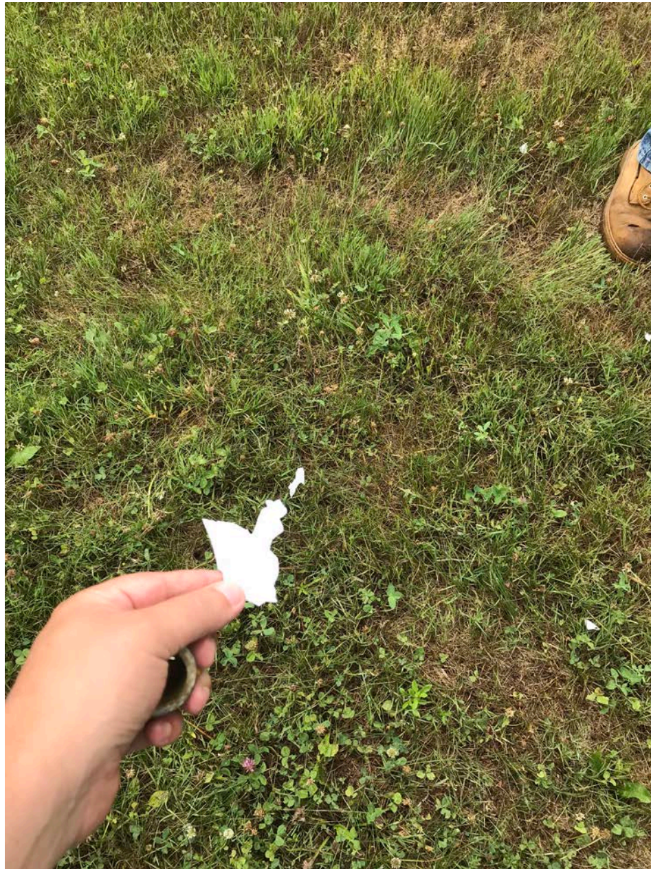
Photo 3 – Paint Chips from Nose Wheel Landing Gear Pant – Courtesy of Pittsfield Municipal Airport
