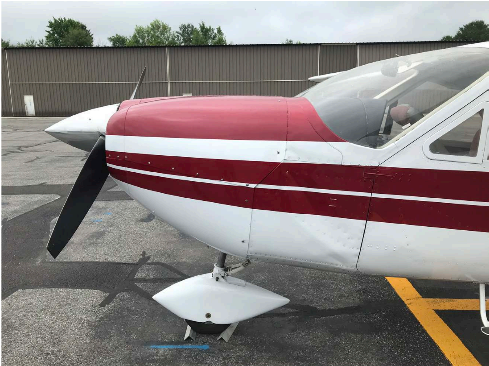
Photo 6 – Left Side Forward Fuselage Wrinkle - Courtesy of Pittsfield Municipal Airport
