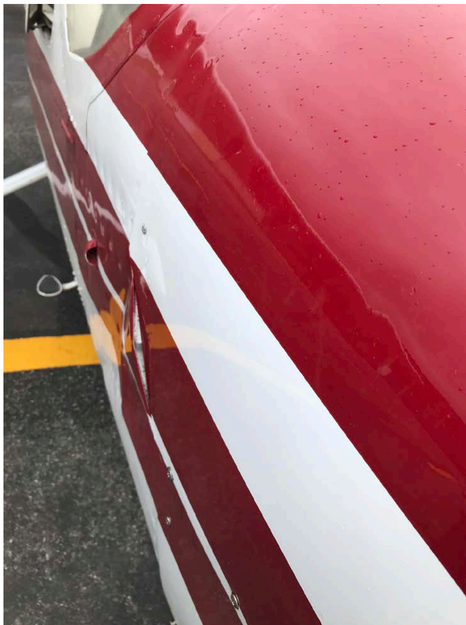
Photo 11 – Close Up of Right Side Forward Fuselage Wrinkle - Courtesy of Pittsfield Municipal Airport
