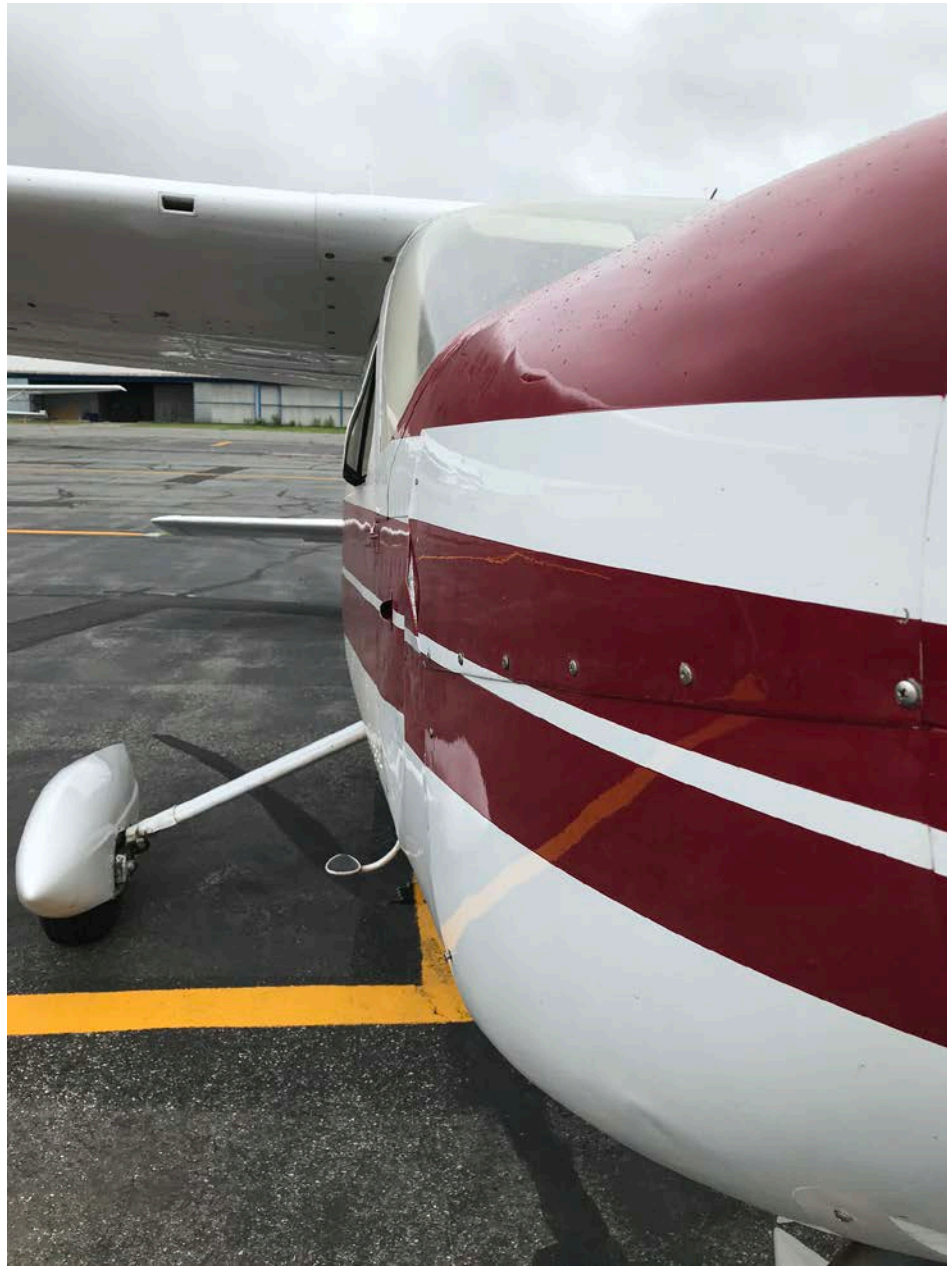
Photo 10 – Right Side Forward Fuselage Wrinkle - Courtesy of Pittsfield Municipal Airport
