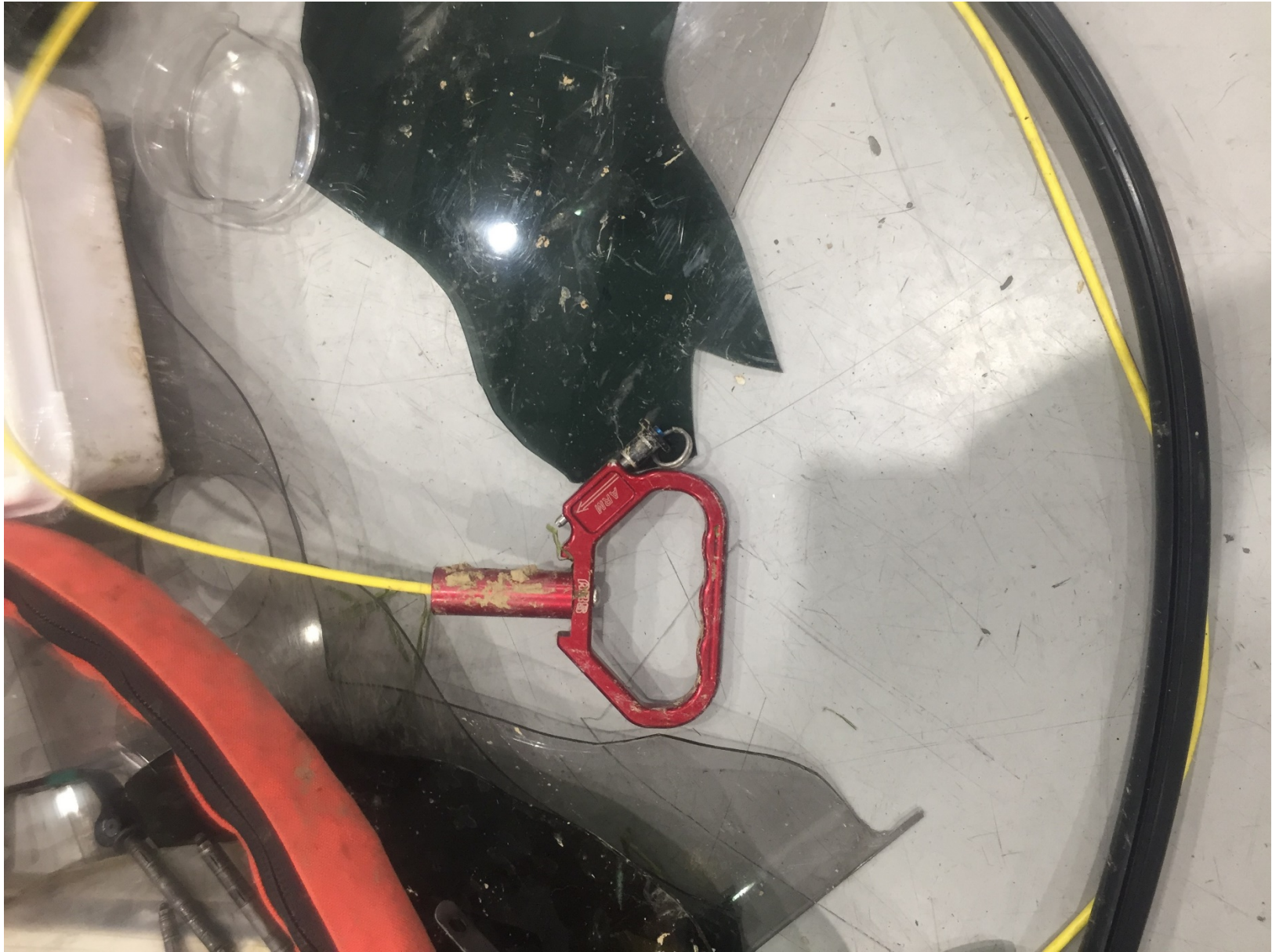
Photo 6 – View of the pulled belly band release handle postaccident (Photo Courtesy of Haverfield Aviation)
