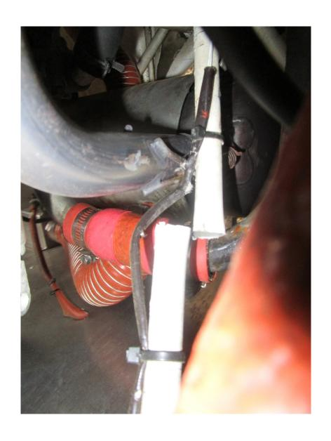
Photo 2 - View of the fractured engine mount (Photo Courtesy of FAA)
