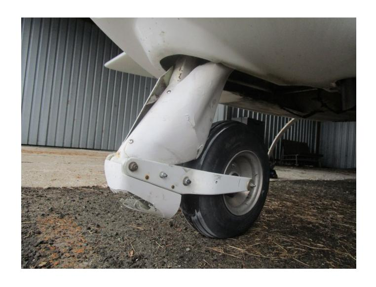
Photo 1 – View of the collapsed nose landing gear (Photo Courtesy of FAA)
