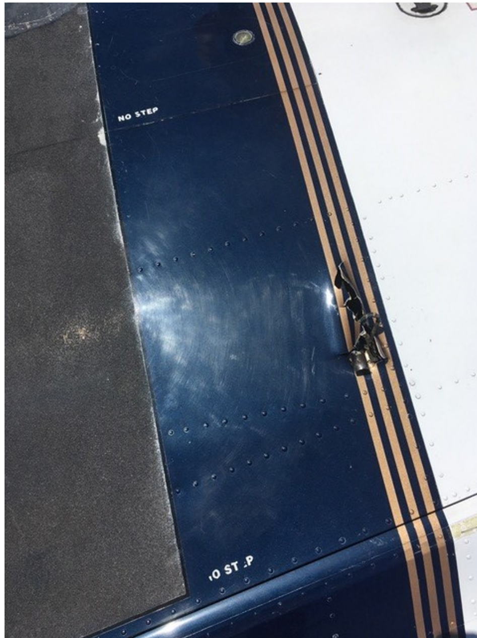
Photo 4 – Right Main Landing Gear Pushed Up Through Right Wing
