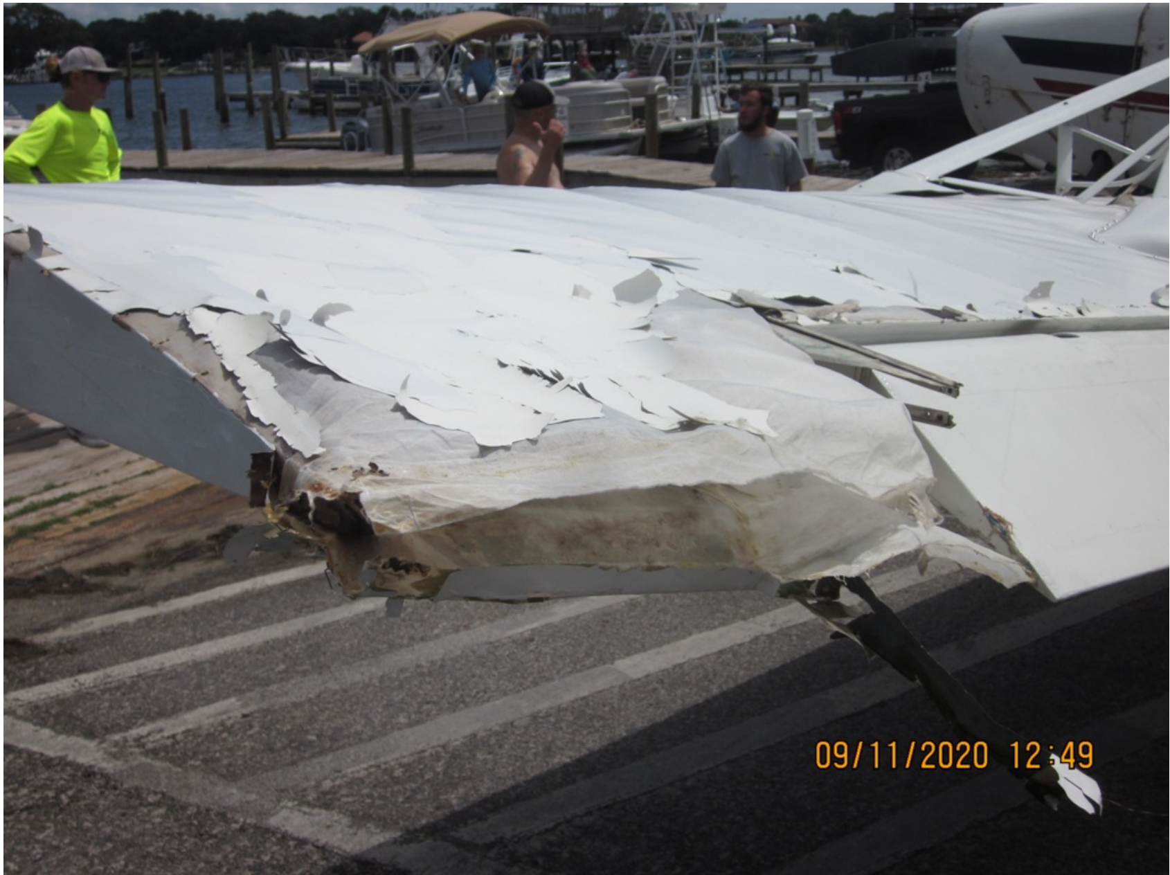
Photo 5 – Damage to the Left-Wing Tip Area (Photo Courtesy of FAA)
