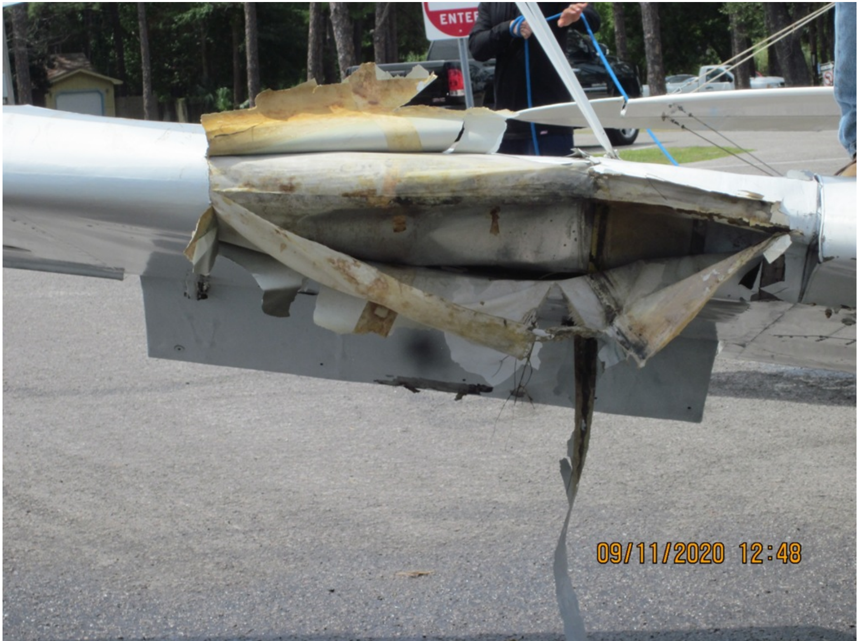
Photo 3 – Leading Edge Damage of Right-Wing (Photo Courtesy of FAA)
