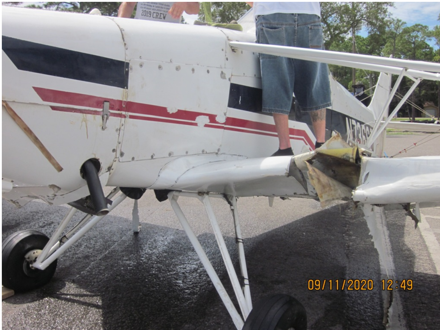
Photo 4 - Leading Edge Damage to Left-Wing (Photo Courtesy of FAA)
