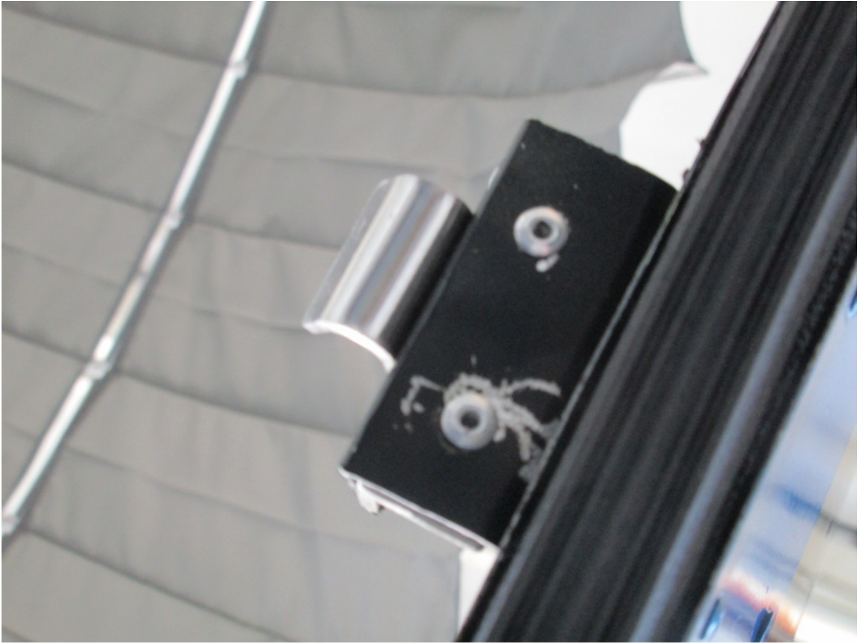
Photo 4 - Secondary Latching System Installed By Pilot/Builder (Photo Courtesy of FAA)
