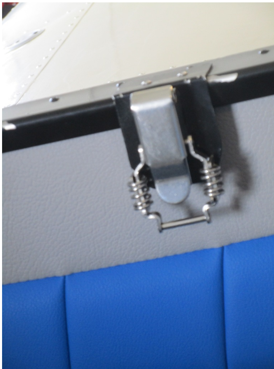
Photo 3 – Secondary Latching System Installed By Pilot/Builder (Photo Courtesy of FAA)
