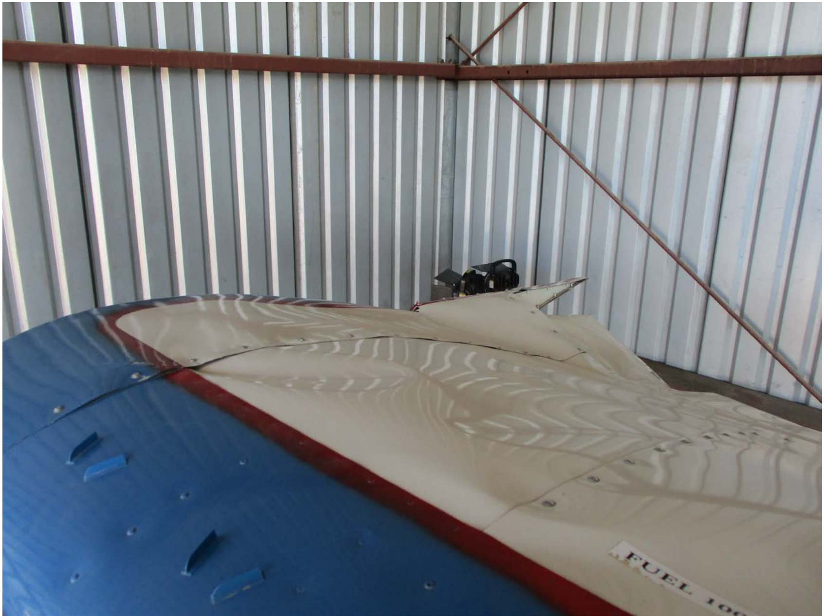
Photo 1 – Right Wing Damage
