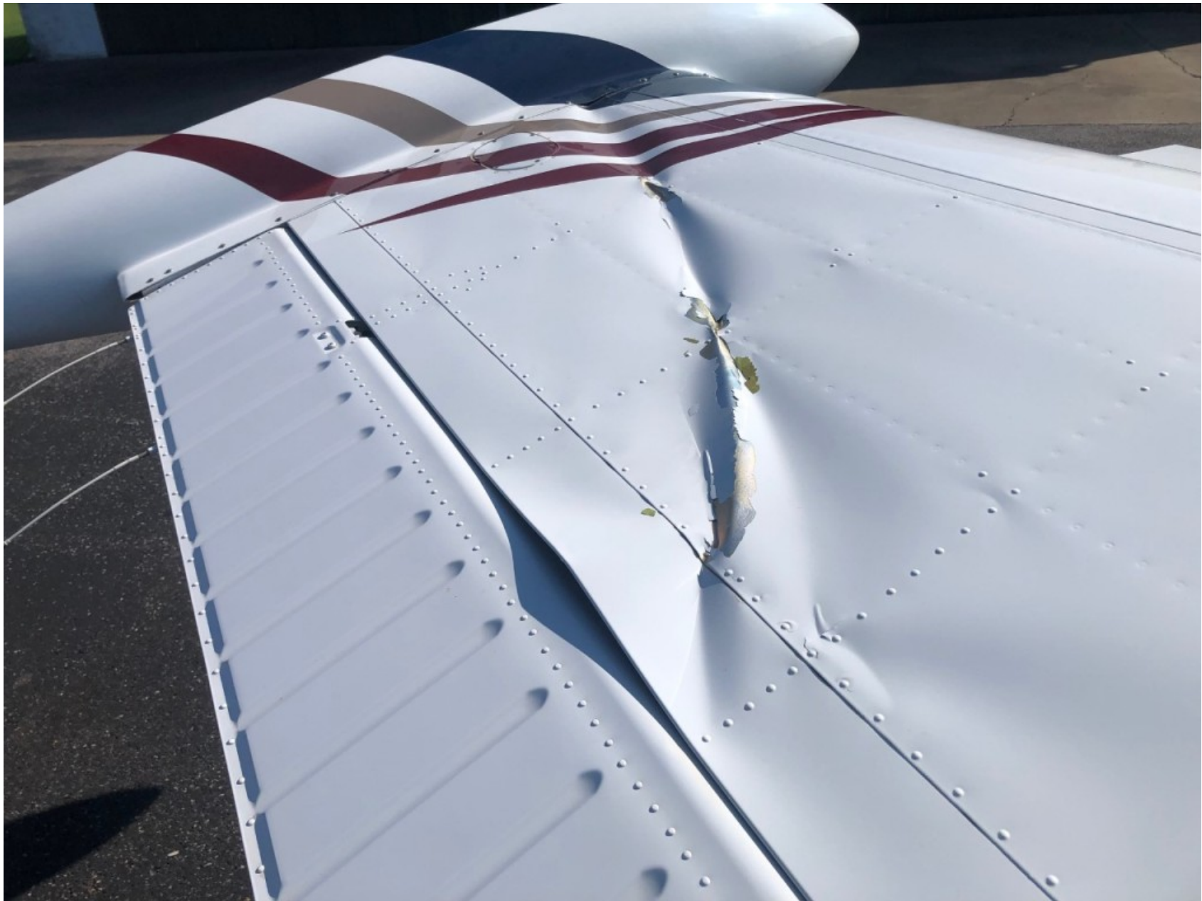
Photo 2 – Damage to Left Wing (Courtesy of FAA)
