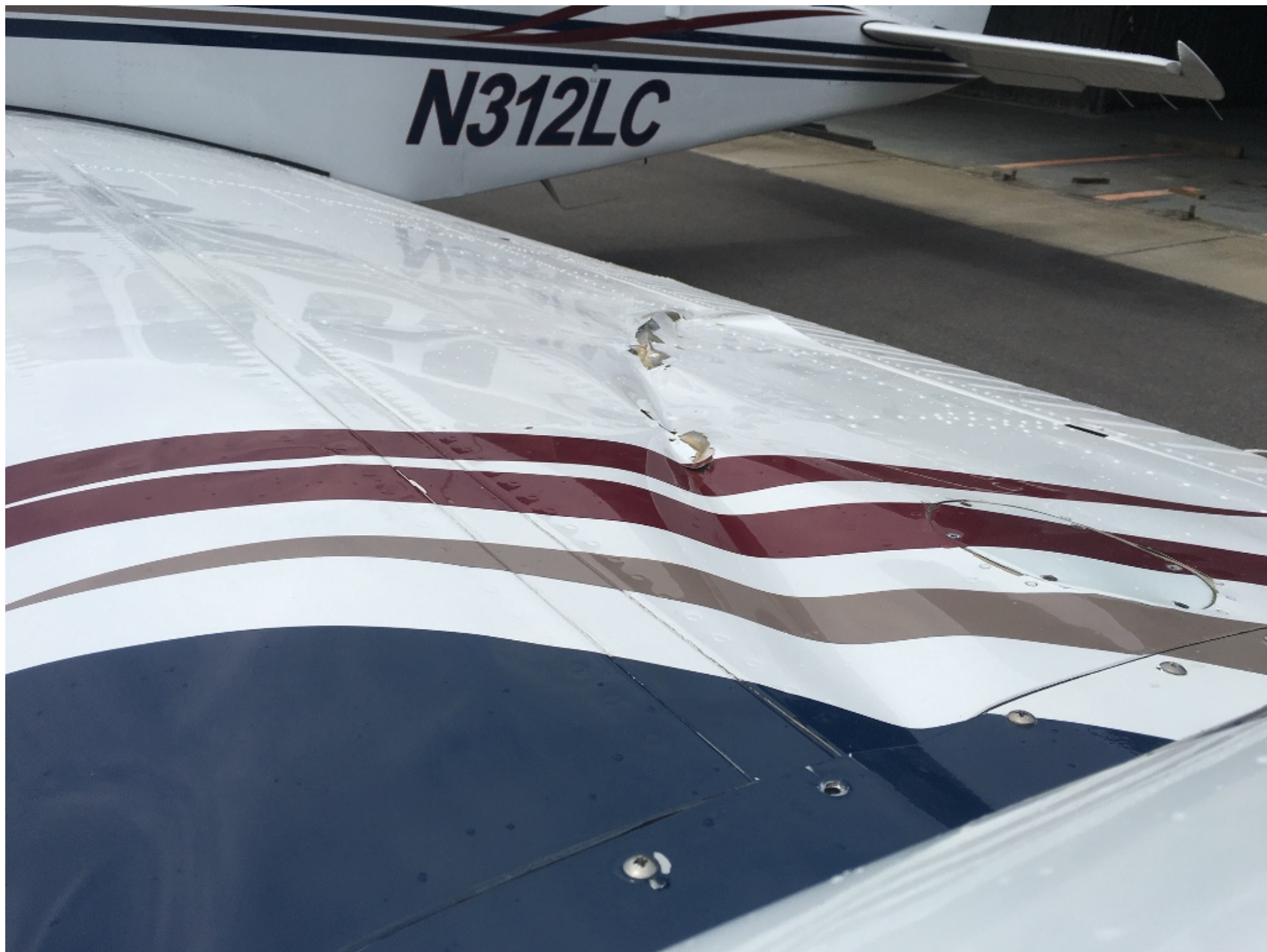
Photo 3 - Damage to Left Wing (Courtesy of FAA)
