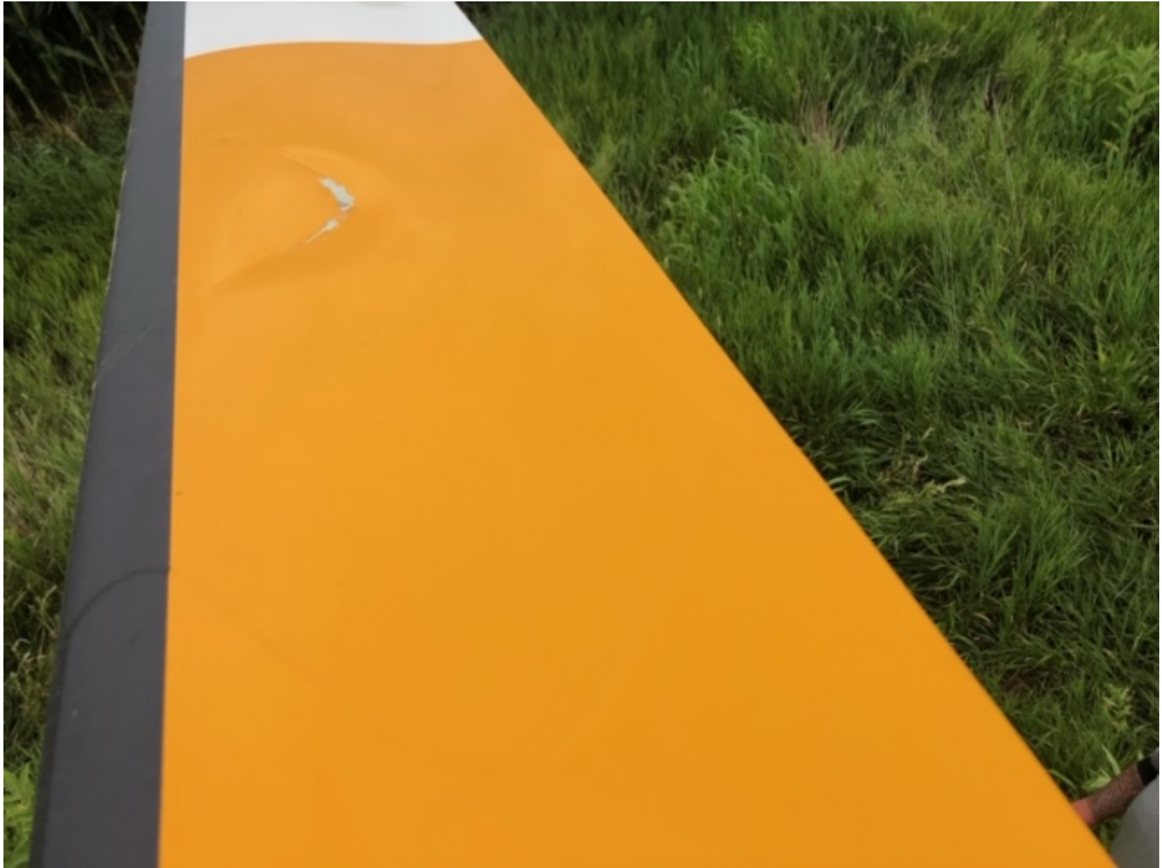
Photo 1 – Damage to main rotor blade
