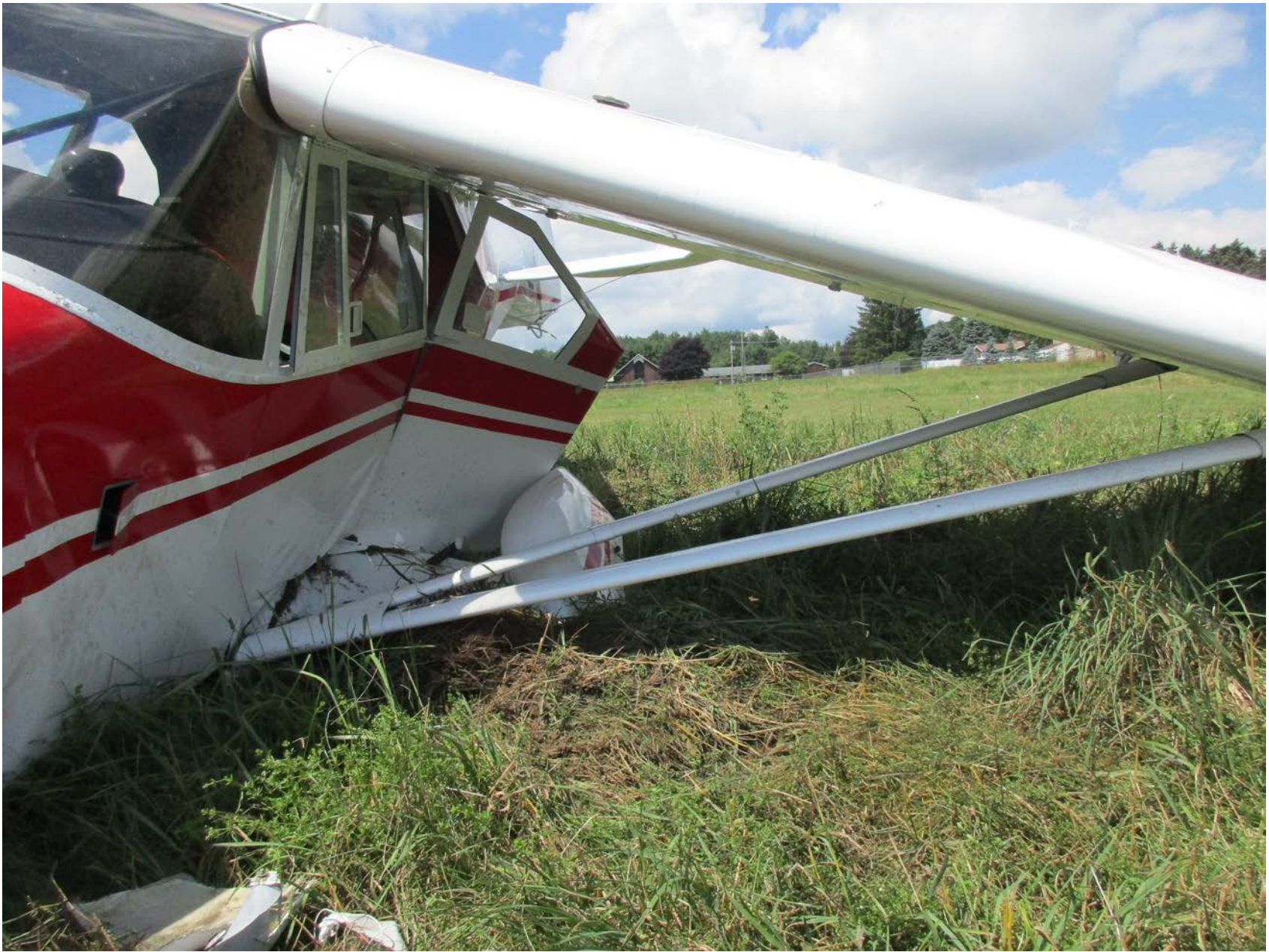
Photo 2 – View of the damage on the left side of the airplane. (Photo courtesy of the FAA)
