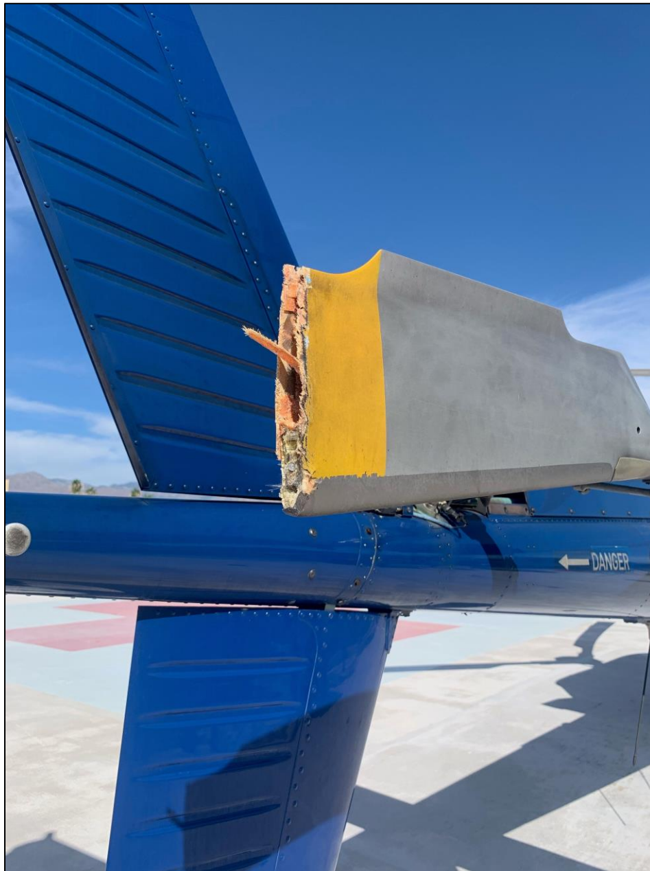
Photo 2 – Accident site, tail rotor blade. (Courtesy of the helicopter operator)
