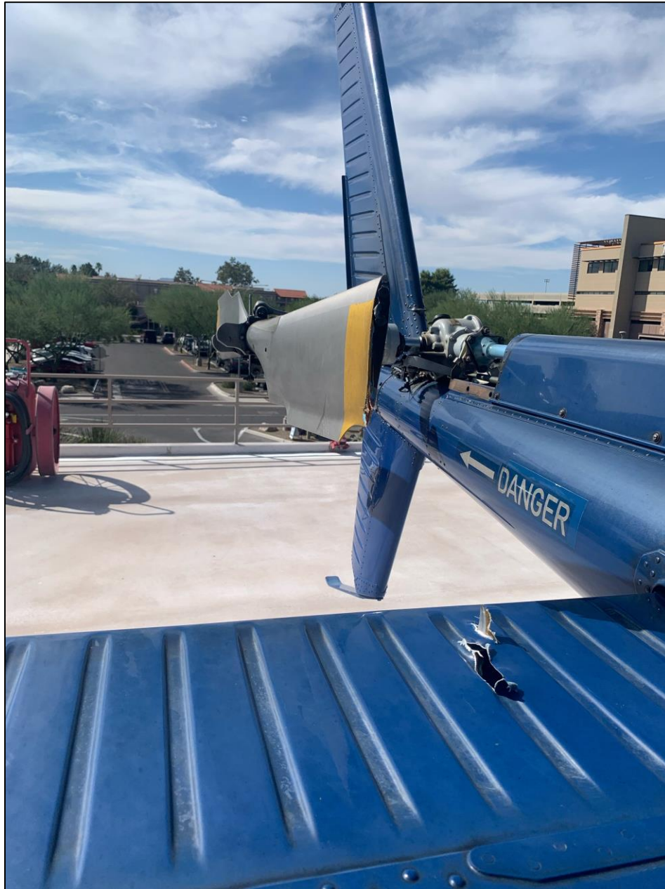
Photo 1 – Accident site, stabilizer, and tail rotor blade damage. (Courtesy of the helicopter operator)
