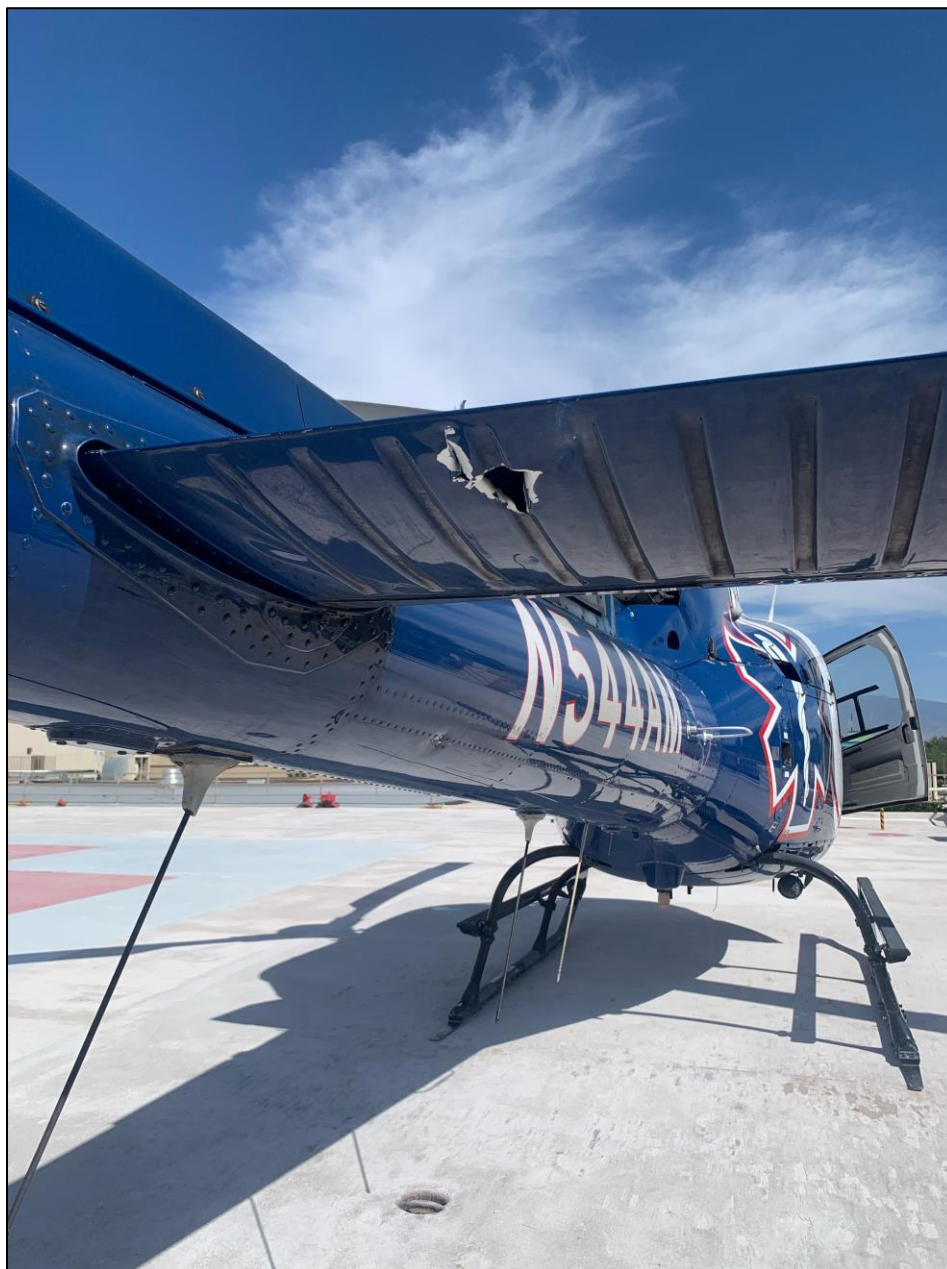
Photo 4 – Accident site, horizontal stabilizer damage. (Courtesy of the helicopter operator)
