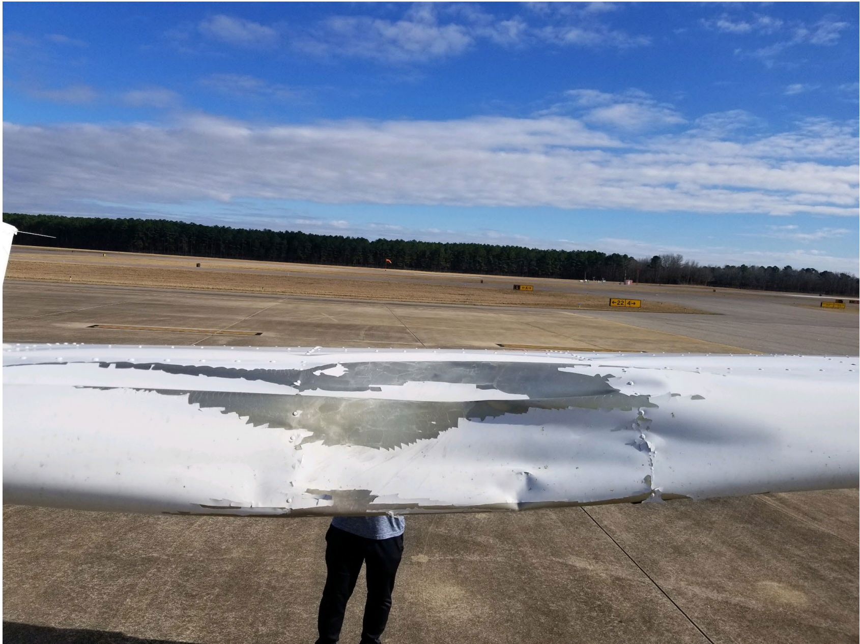
Photo 1 – Front View of Left Wing Damage – Courtesy of FAA
