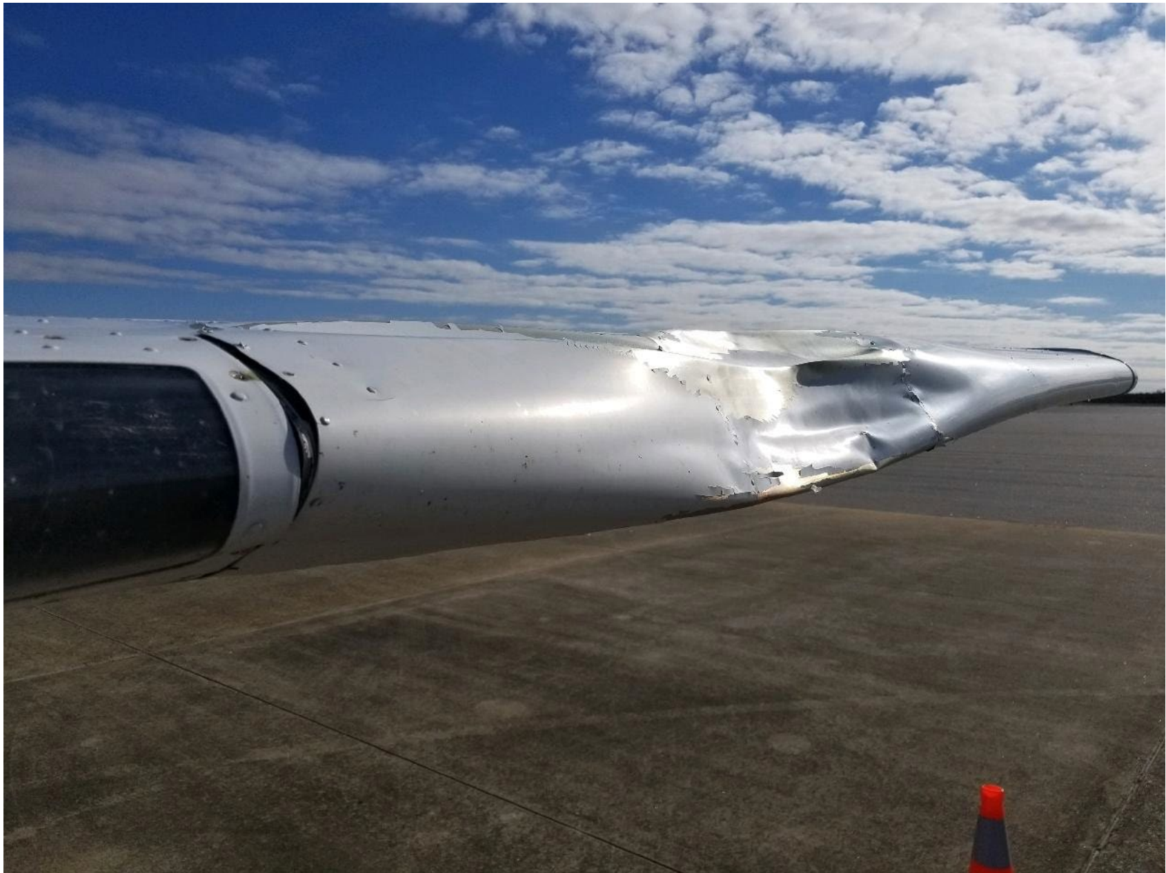
Photo 3 – Side View of Left Wing Damage – Courtesy of FAA
