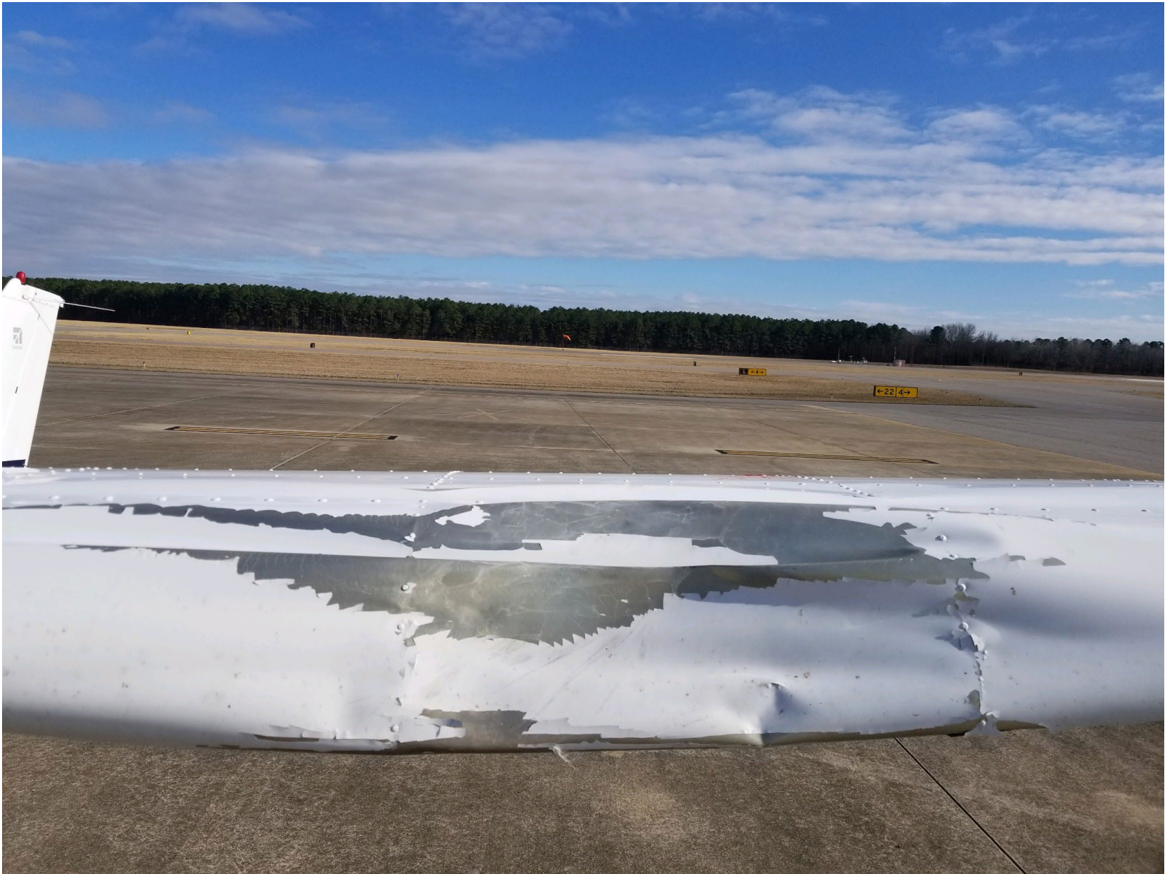
Photo 2 – Close Up of Left Wing Damage – Courtesy of FAA
