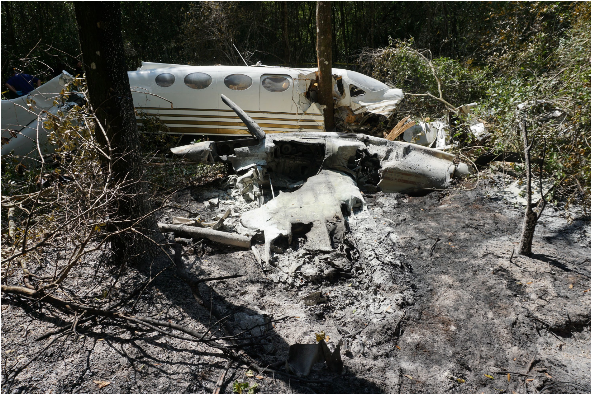
Photo 4 – View of right side of airplane showing post fire and structural damage.
