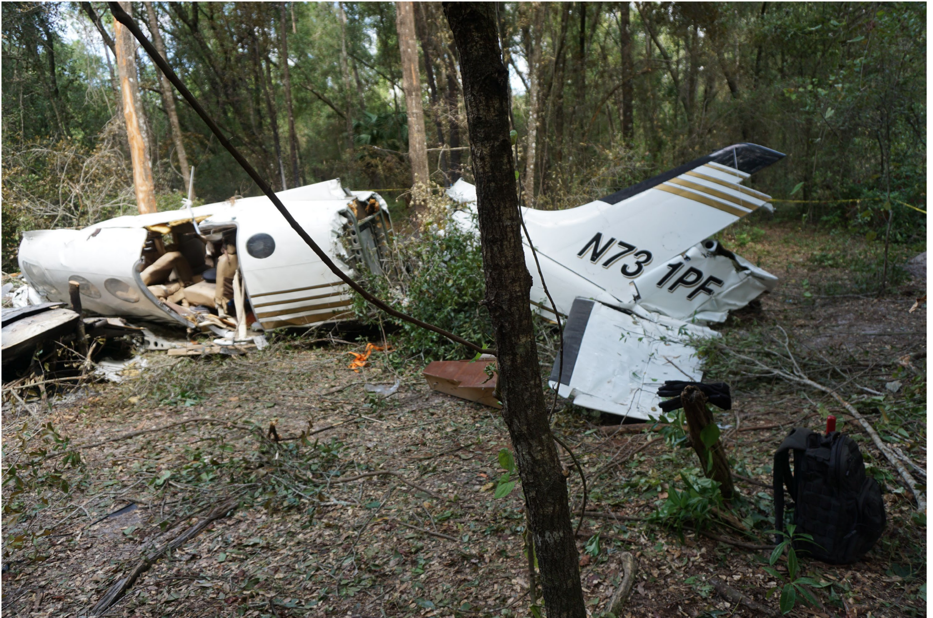
Photo 1 – View of left side of airplane showing structural damage
