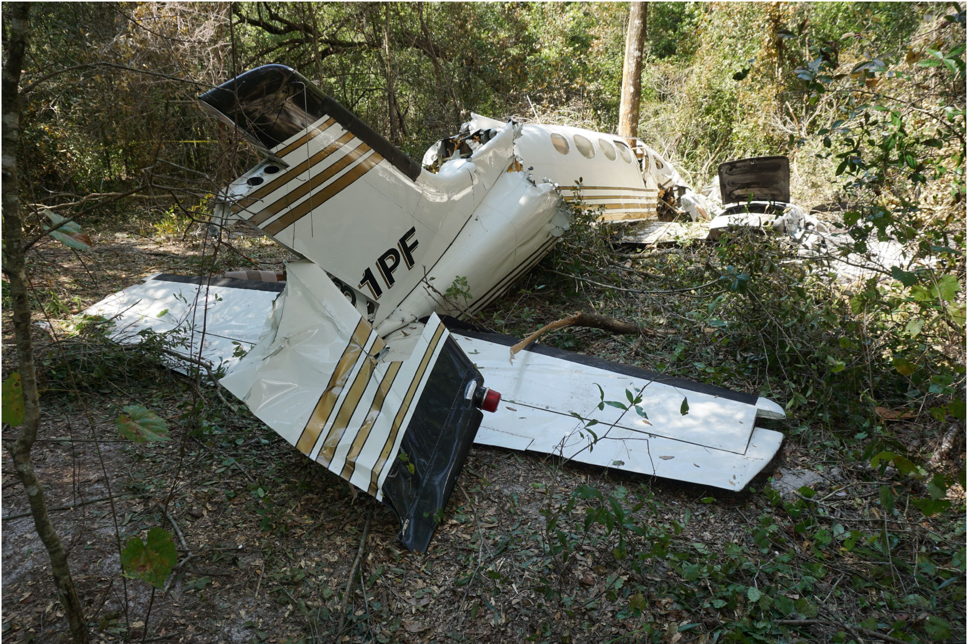
Photo 3 – View of right side of airplane showing structural damage
