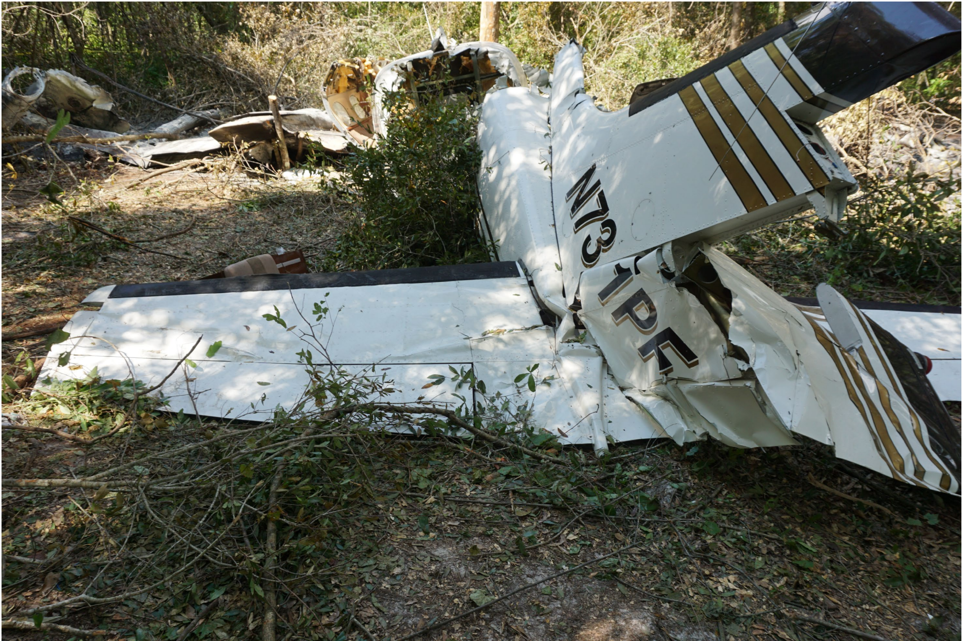
Photo 2 – View of aft of airplane showing structural damage
