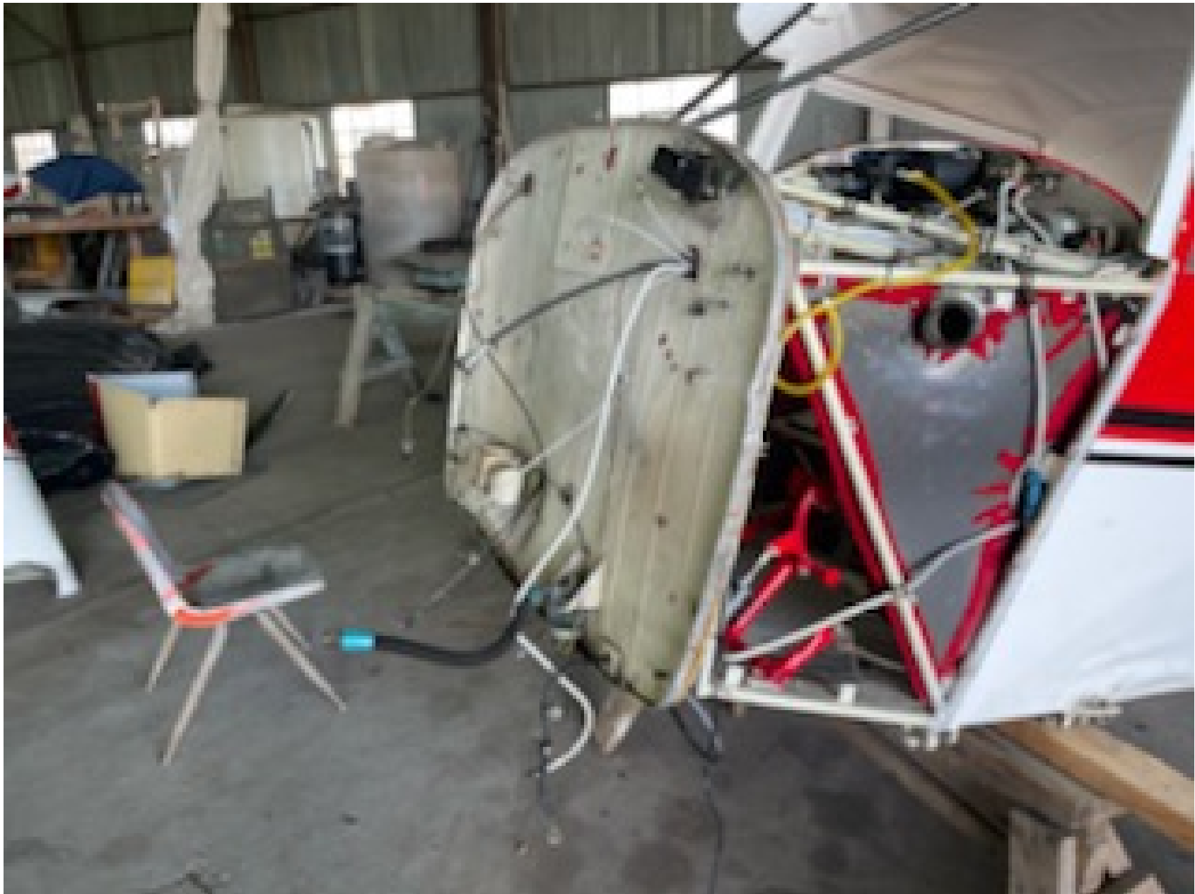
Photo 2 – View of damaged firewall
