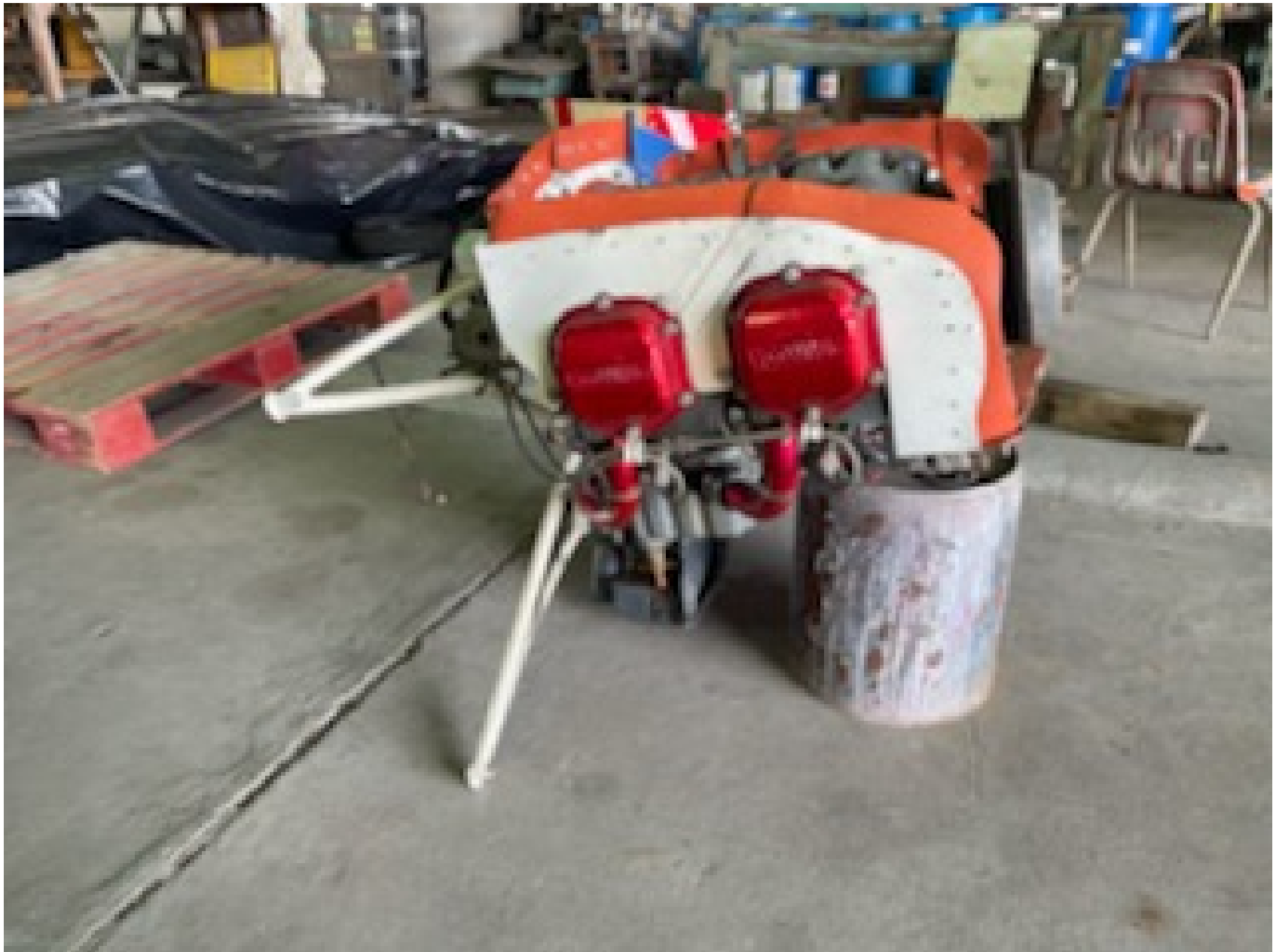
Photo 1 – View of motor mount showing a bend in the lower section.
