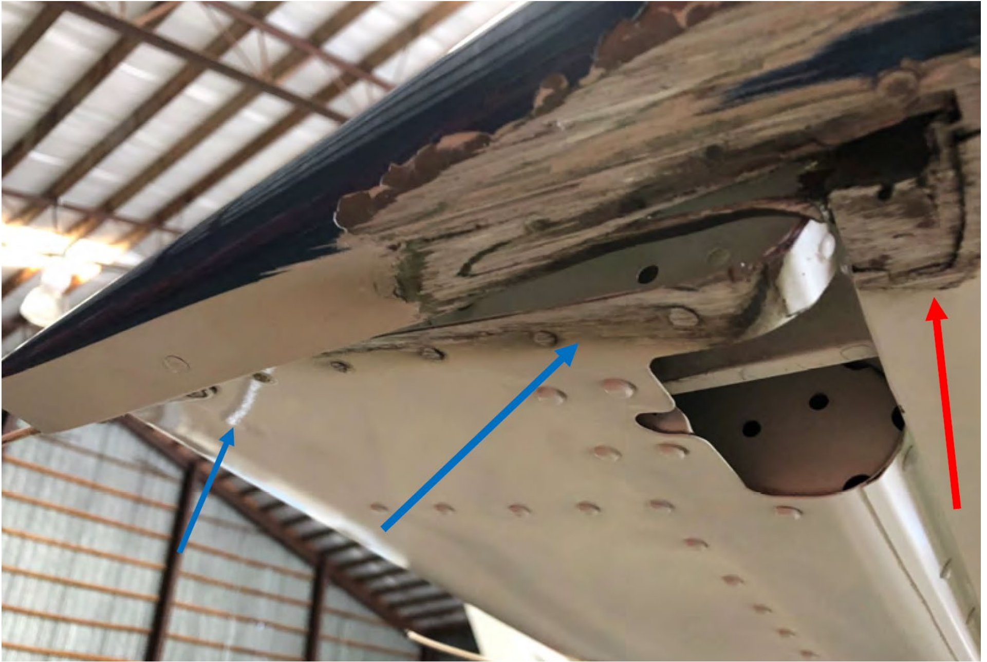
Photo 2 – View of left wing damage (Courtesy of Insurance Adjuster)
