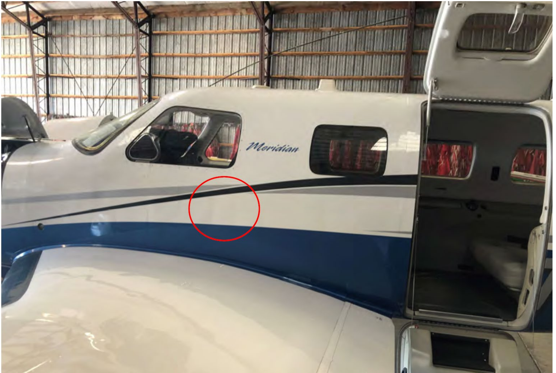
Photo 4 – View of fuselage. Circle notes a wrinkle that is difficult to see in photographs. (Courtesy of insurance adjuster)
