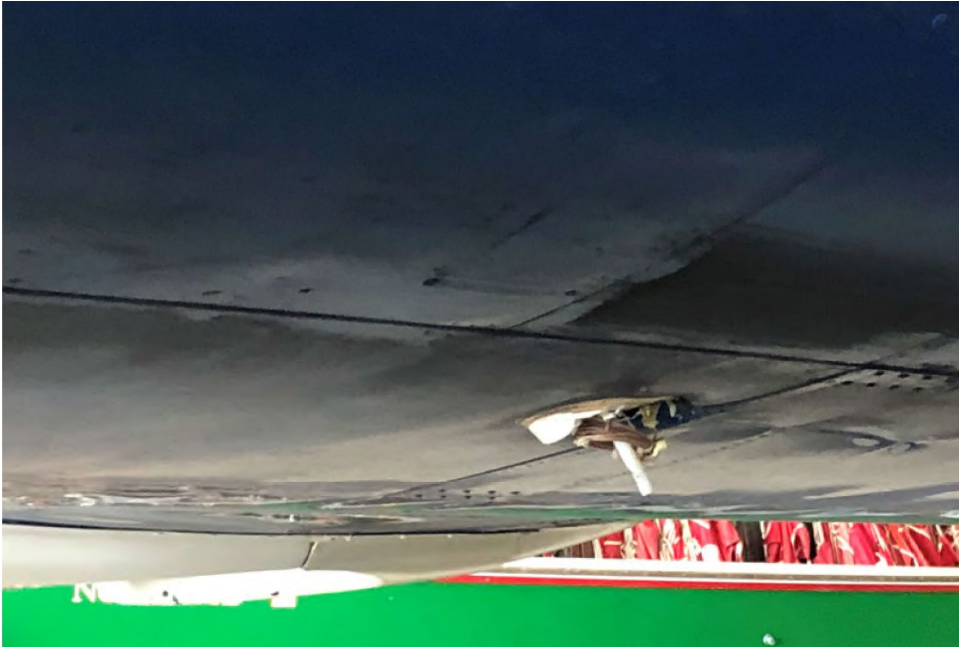
Photo 3 – Wrinkle on lower section of fuselage. (Courtesy of insurance adjuster)
