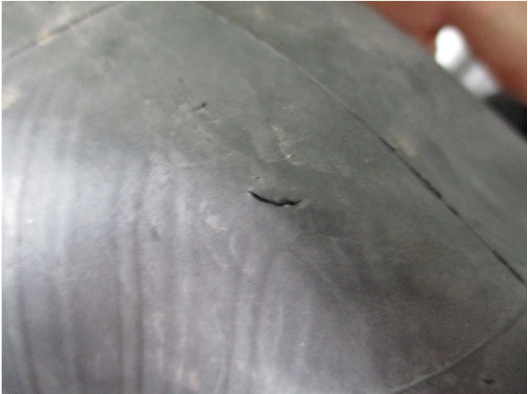
Photo 3 – View of punctured tire inner tube
