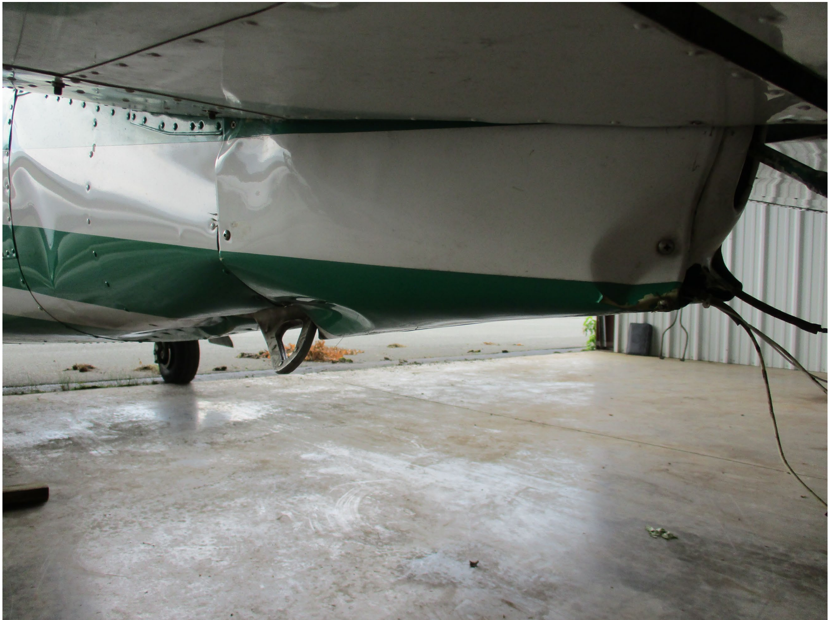
Photo 2 – View of bottom of fuselage (empennage) showing buckling
