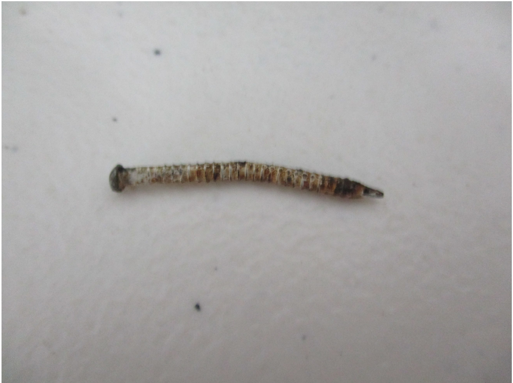
Photo 4 – View of nail found in punctured tire inner tube.
