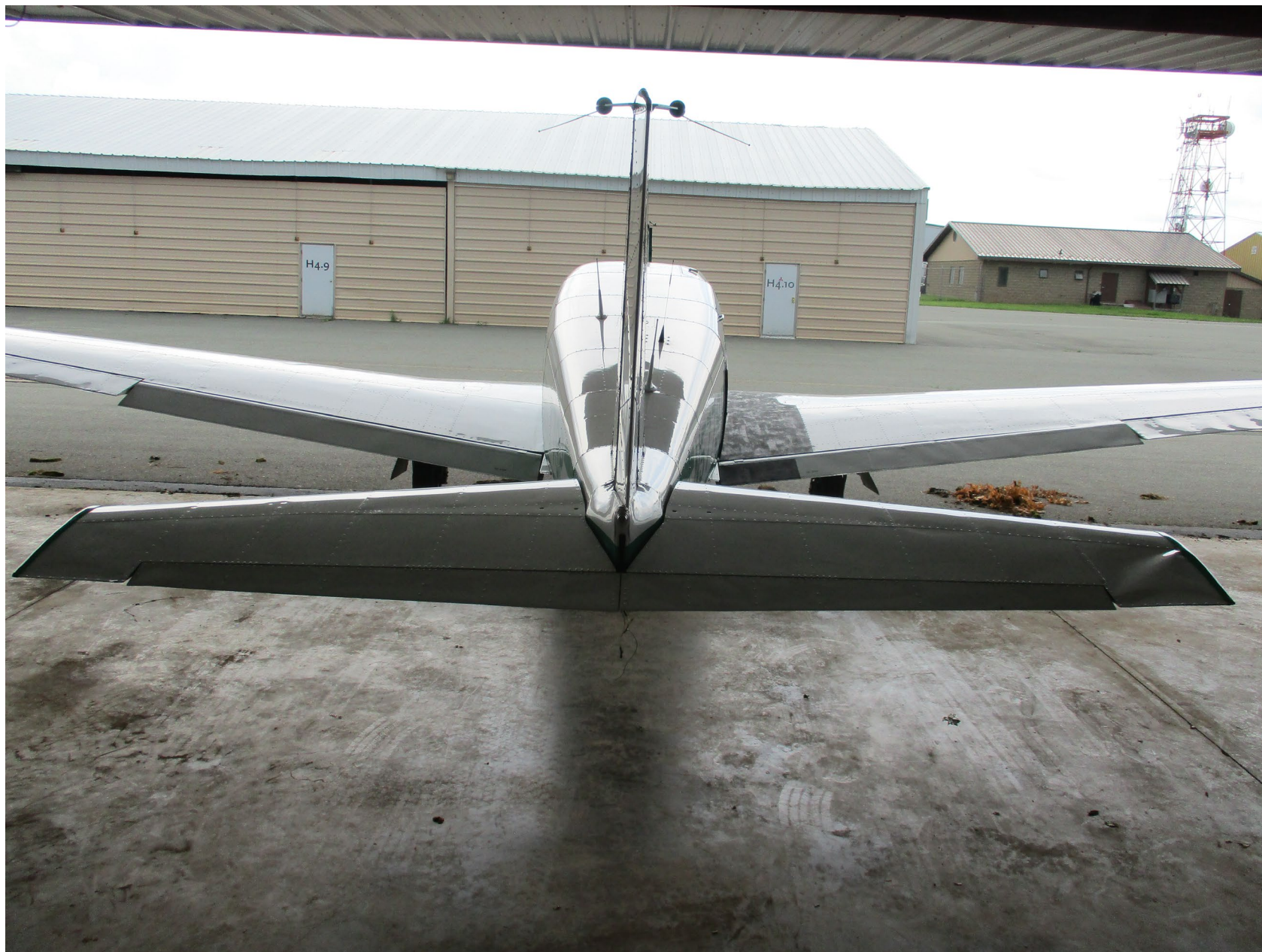
Photo 1 – Aft the view of airplane showing right horizontal stabilizer bent
