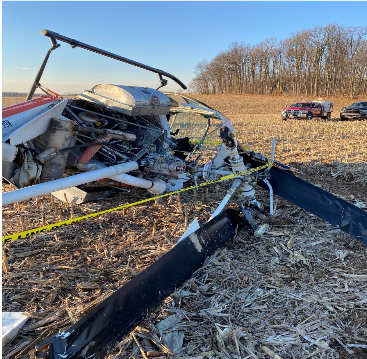
Photo 2 – View top view of helicopter showing damage to rotor blades fuselage.
