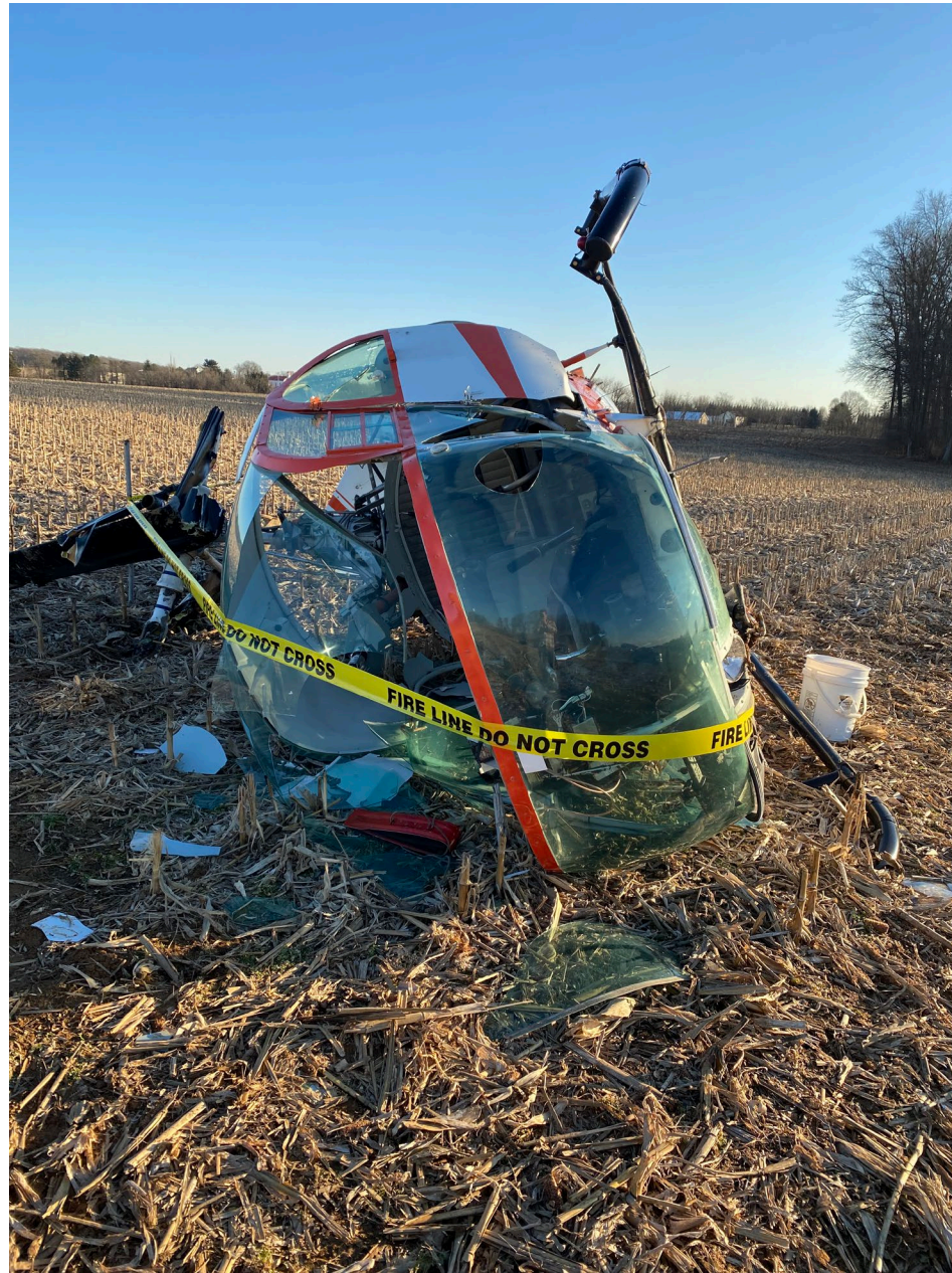
Photo 1 – View of helicopter showing airframe damage and resting on the left side.
