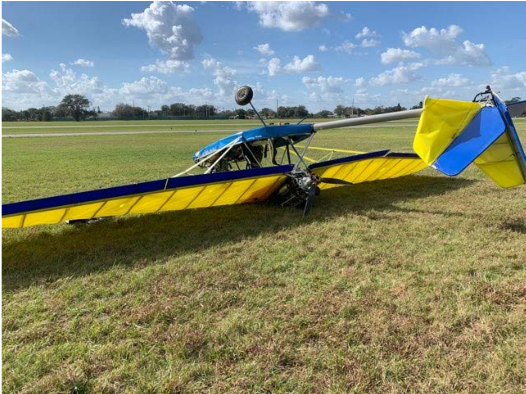
Photo 2 – View of right side of airplane inverted showing horizontal stabilizer and elevator buckling
