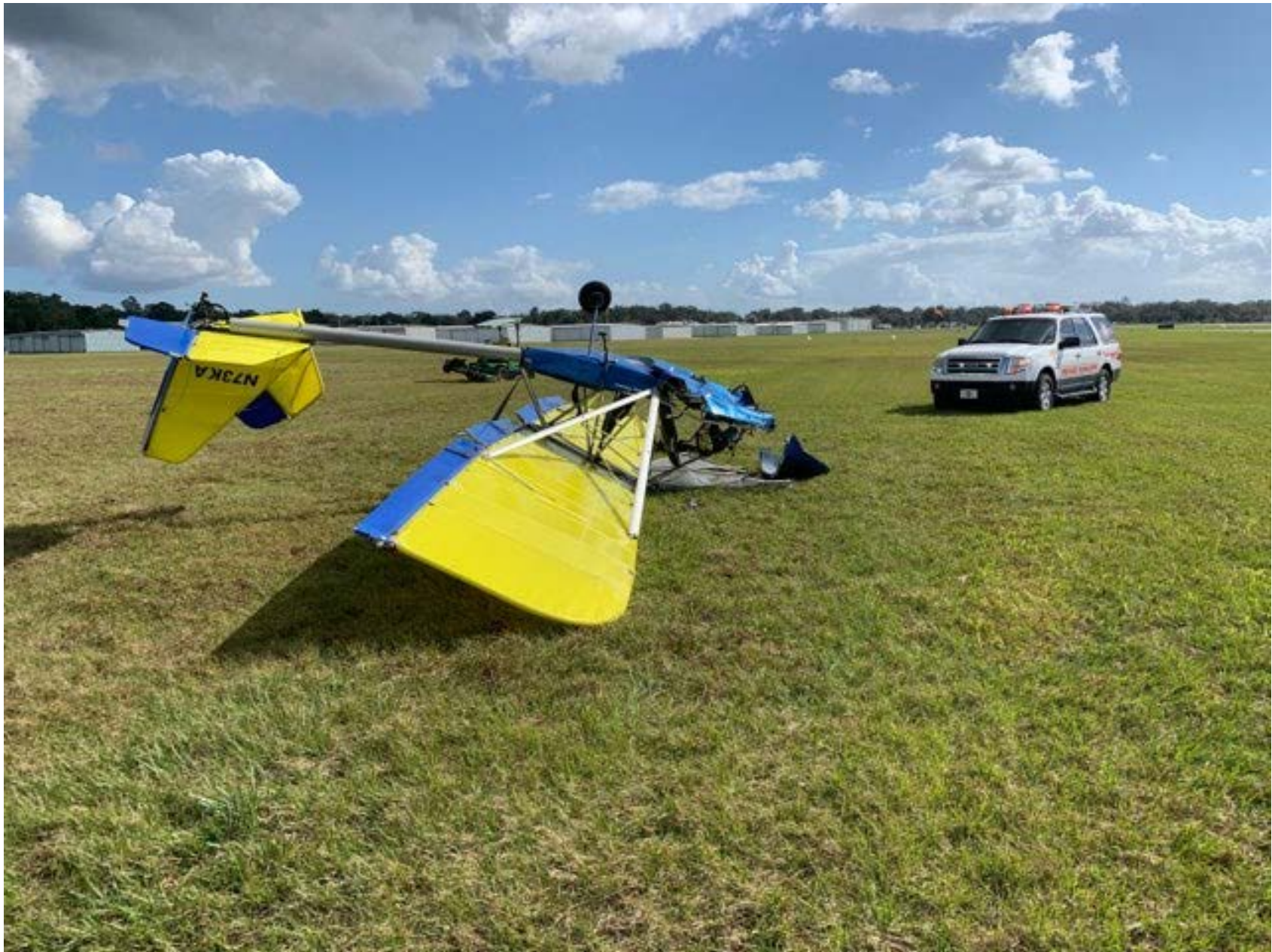
Photo 1 – View of left side of airplane inverted showing cockpit crushing
