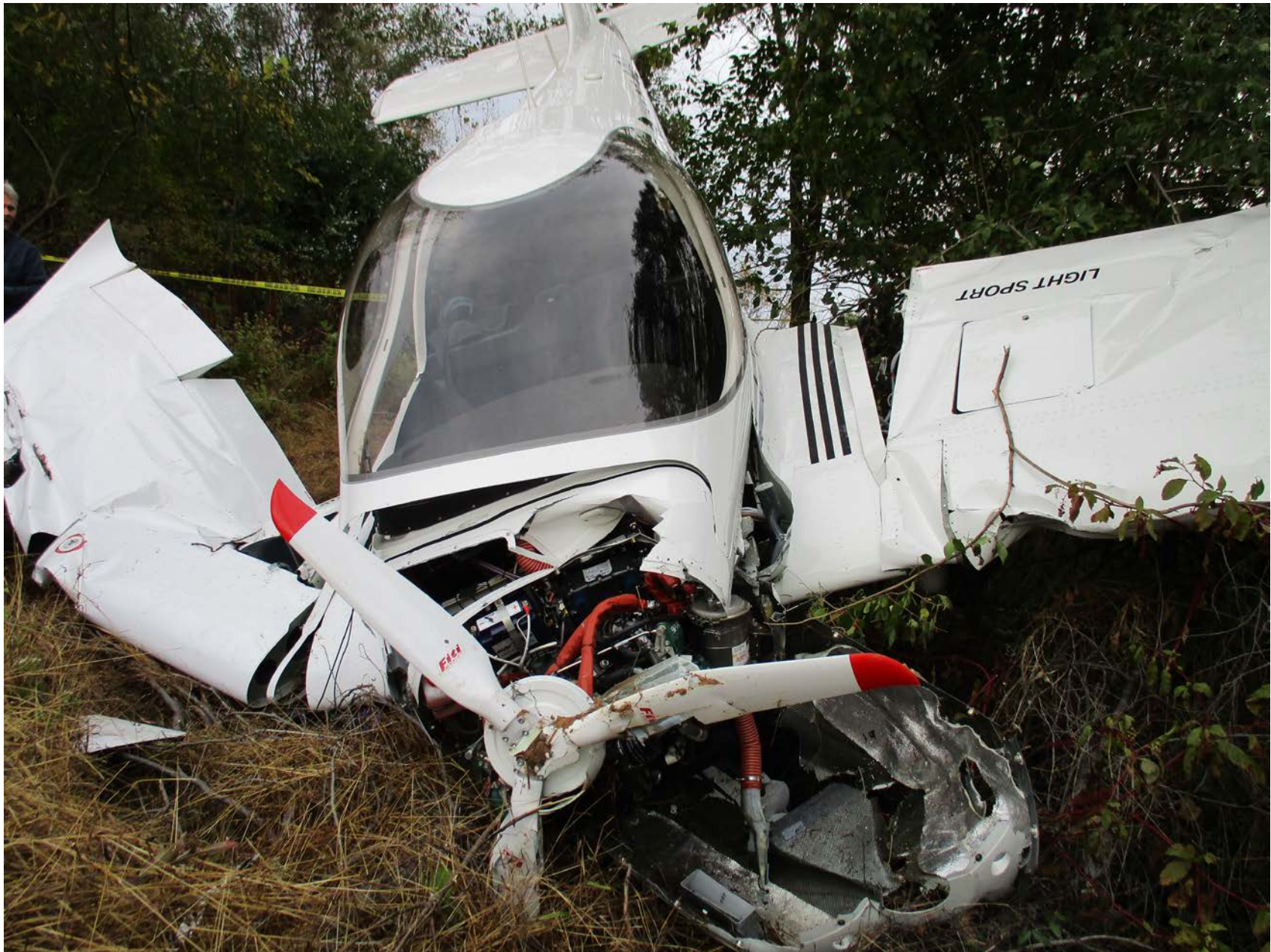
Photo 2 – View of airplane from the front showing forward crush damage
