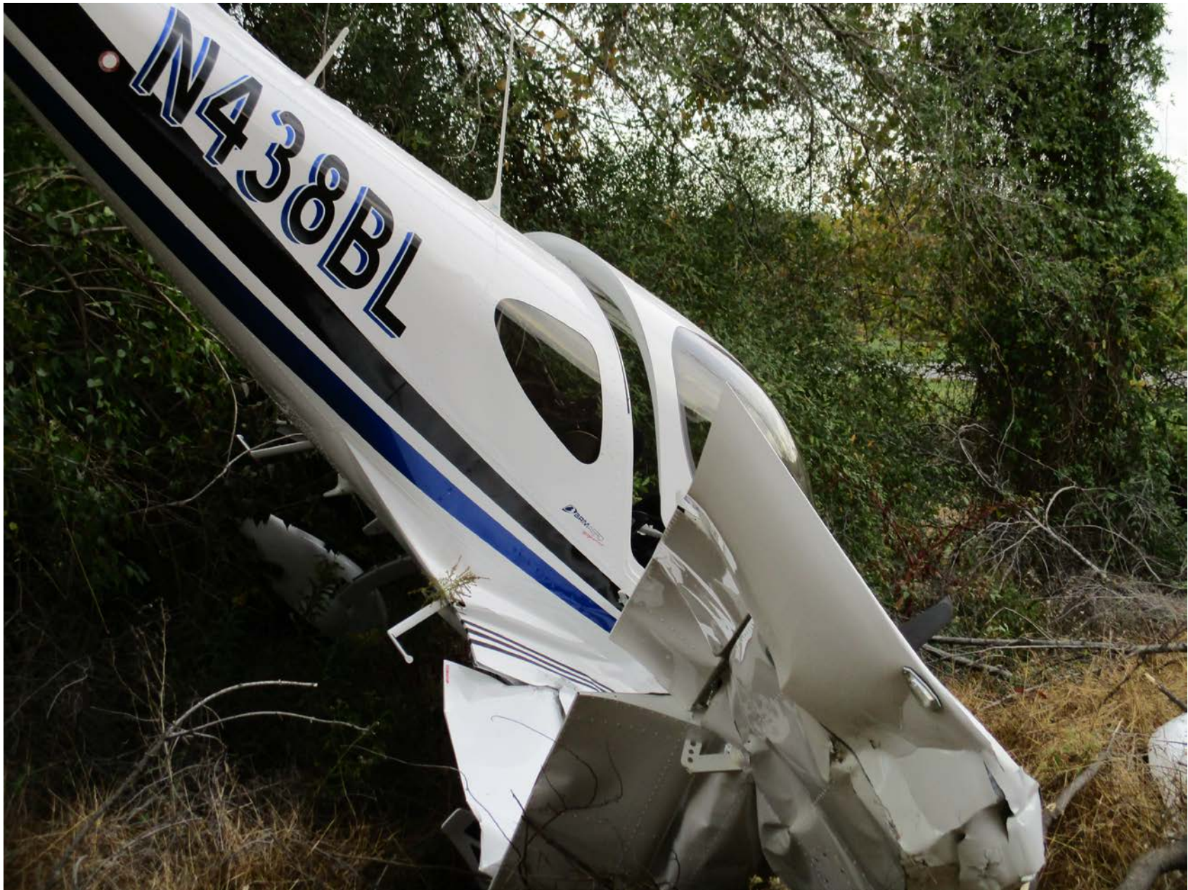
Photo 1 – View of airplane from the left side showing right wing damage
