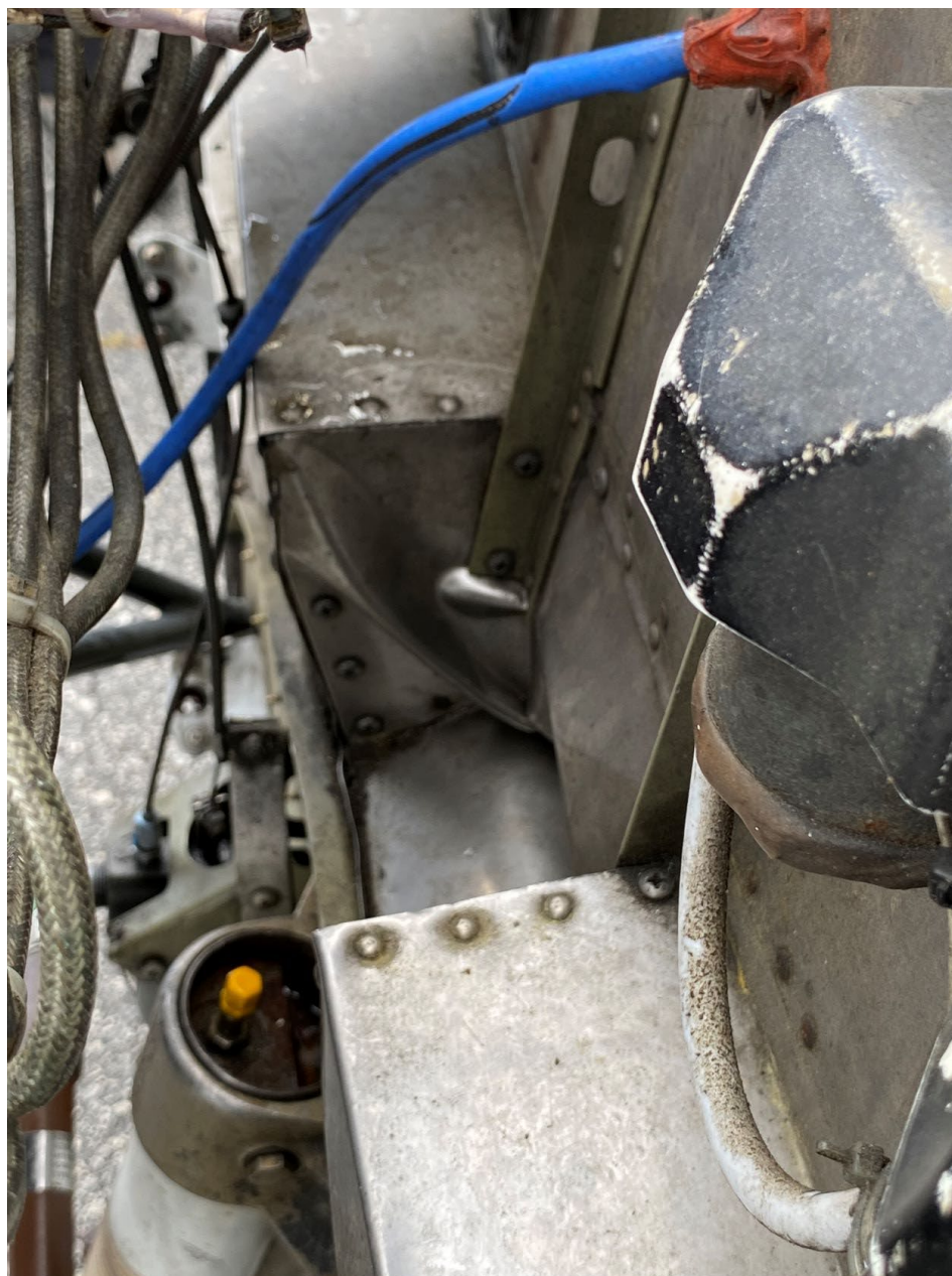
Photo 2 – View of Damage to Nose Landing Gear Support Structure (FAA)
