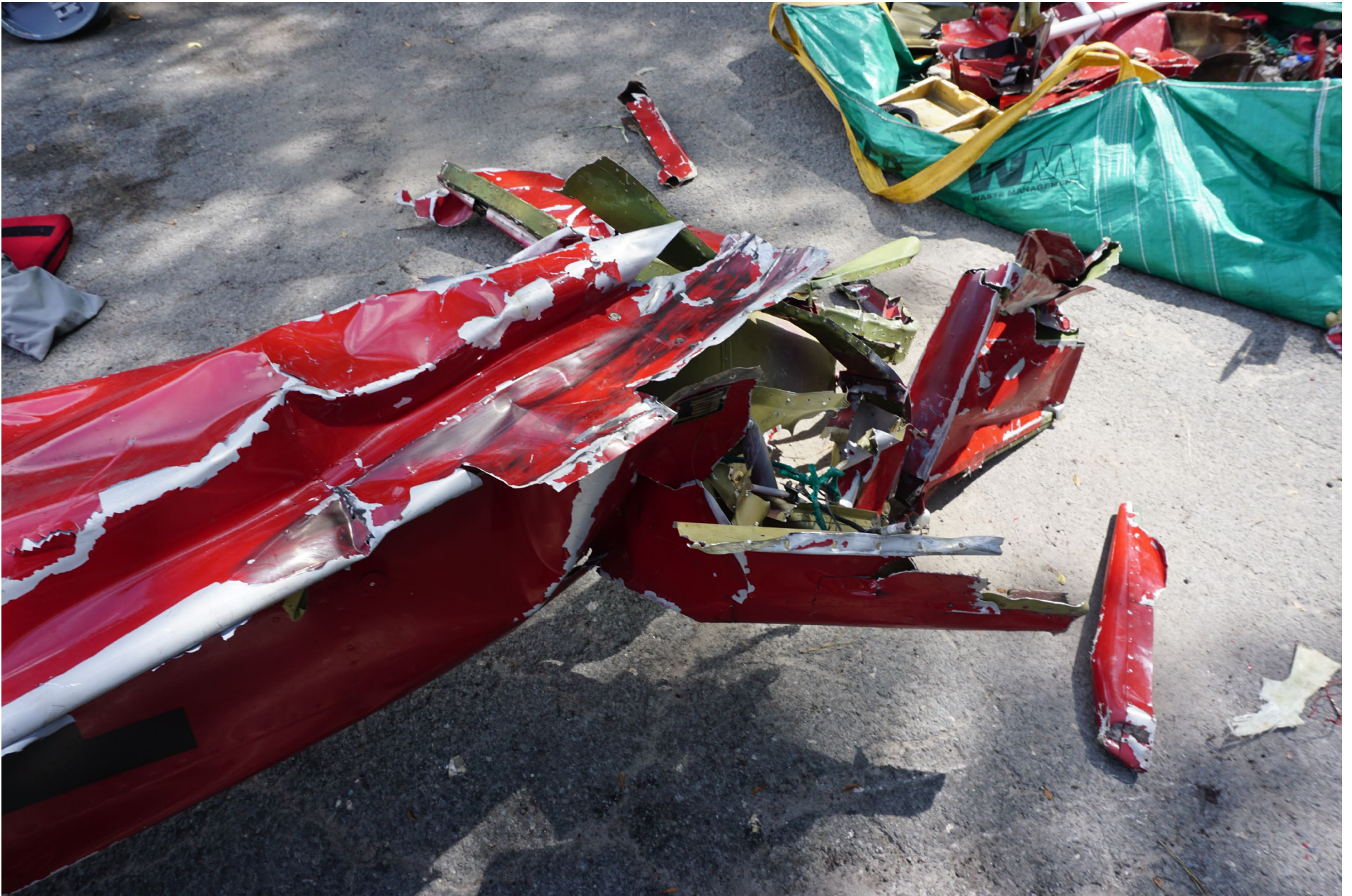
Photo 3 – View of empennage showing black tire skid mark.
