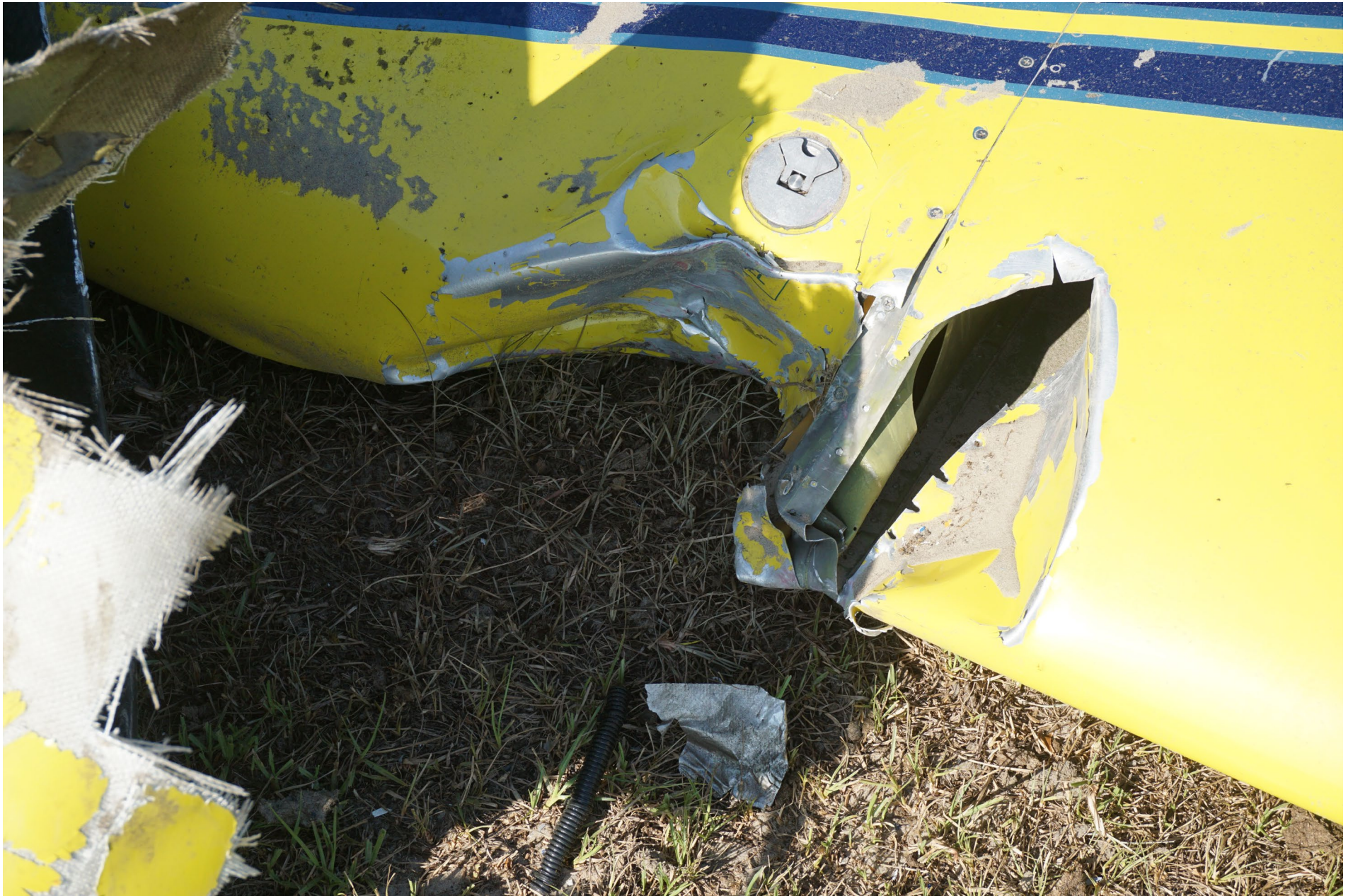
Photo 6 – View of semicircular damage on leading edge of left inboard wing.
