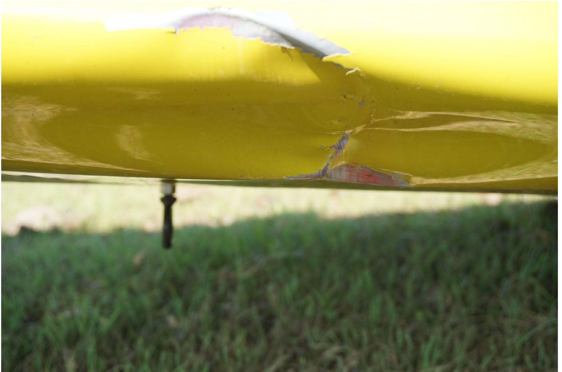
Photo 7 – View of red paint transfer on leading edge of right wing.
