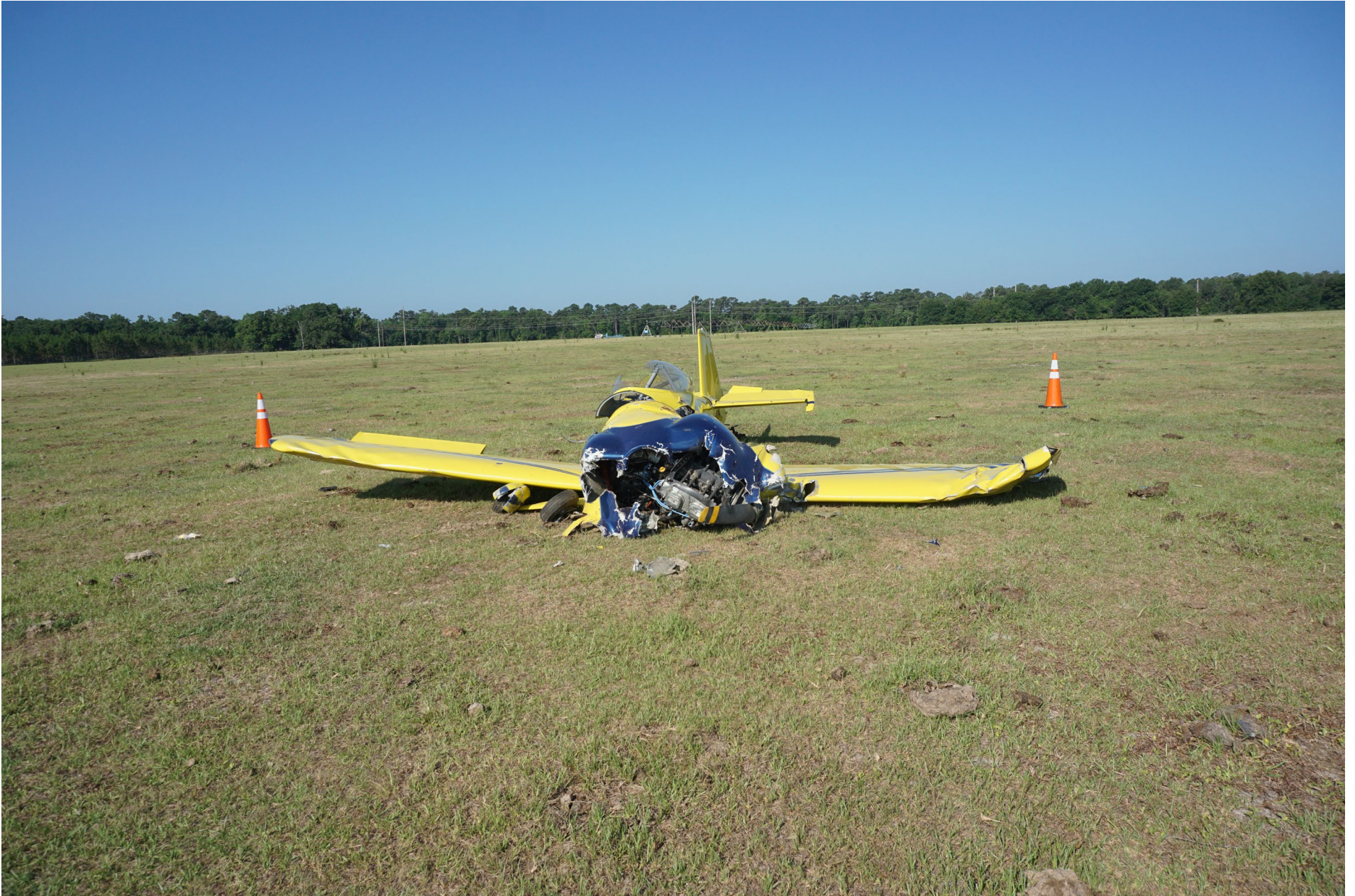
Photo 5 – View of N203DD in field showing structural damage throughout aircraft.
