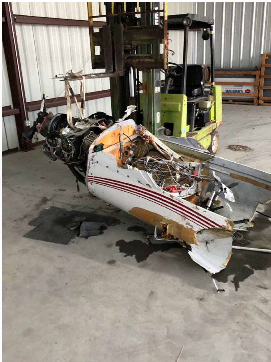
Photo 5 – View of the forward fuselage/cockpit with engine attached
