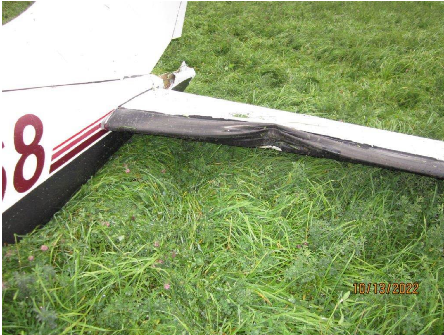
Photo 3: View of damage to the airplane's left horizontal stabilizer (Photo Courtesy of FAA)
