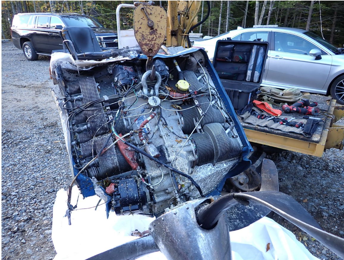
Photograph 5 - View of the top of the engine after recovery from the accident site.
