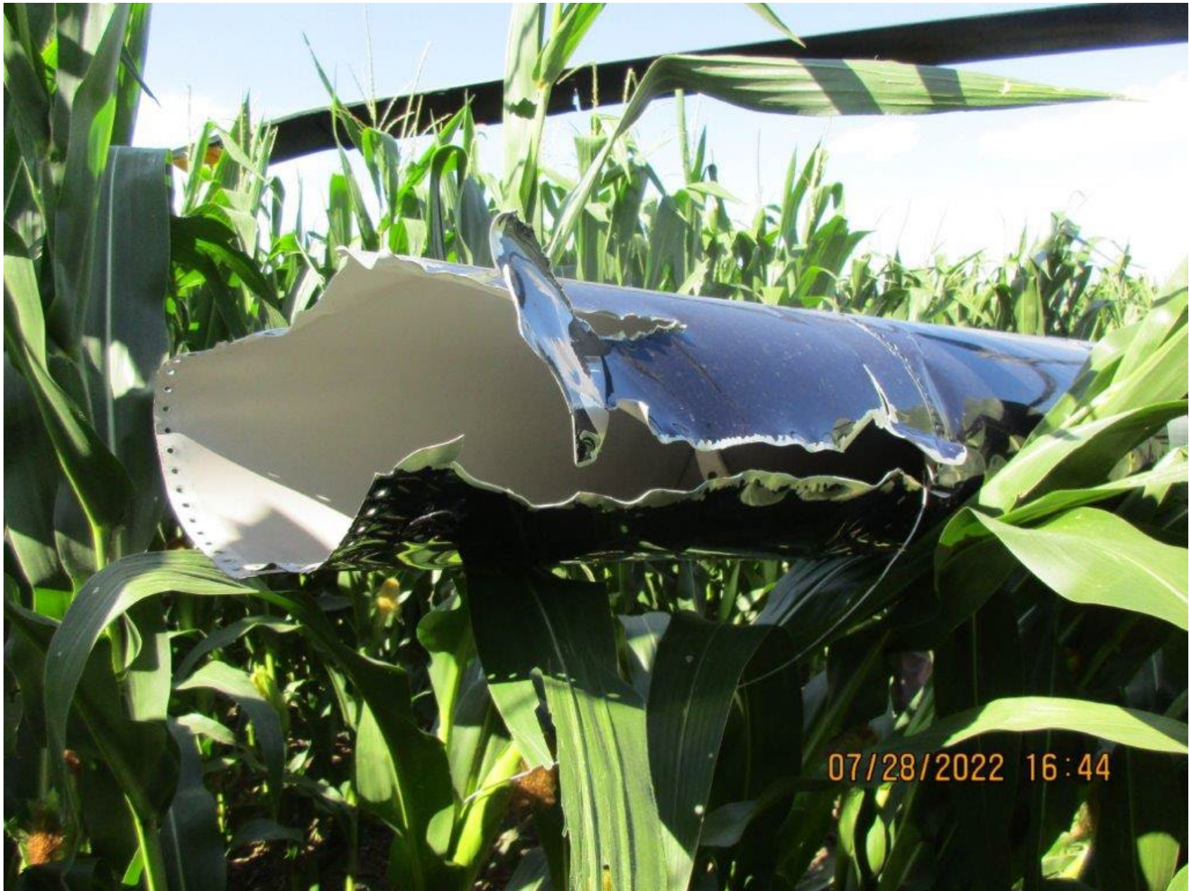
Photo 1 – Portion of Separated Tail boom Laying in Mature Corn Field (Source: FAA)
