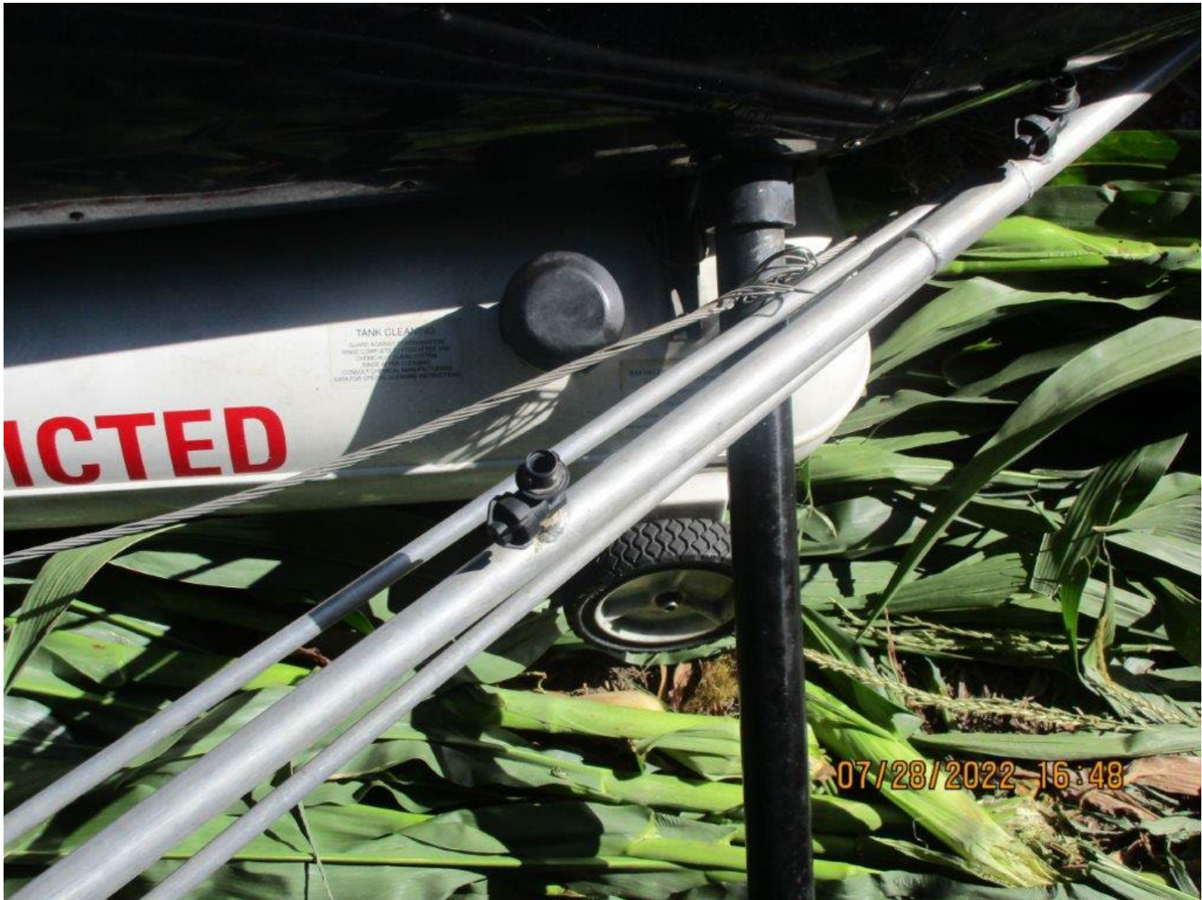
Photo 3 – Closeup of Remnants of Wire Embedded in Wreckage (Source: FAA)
