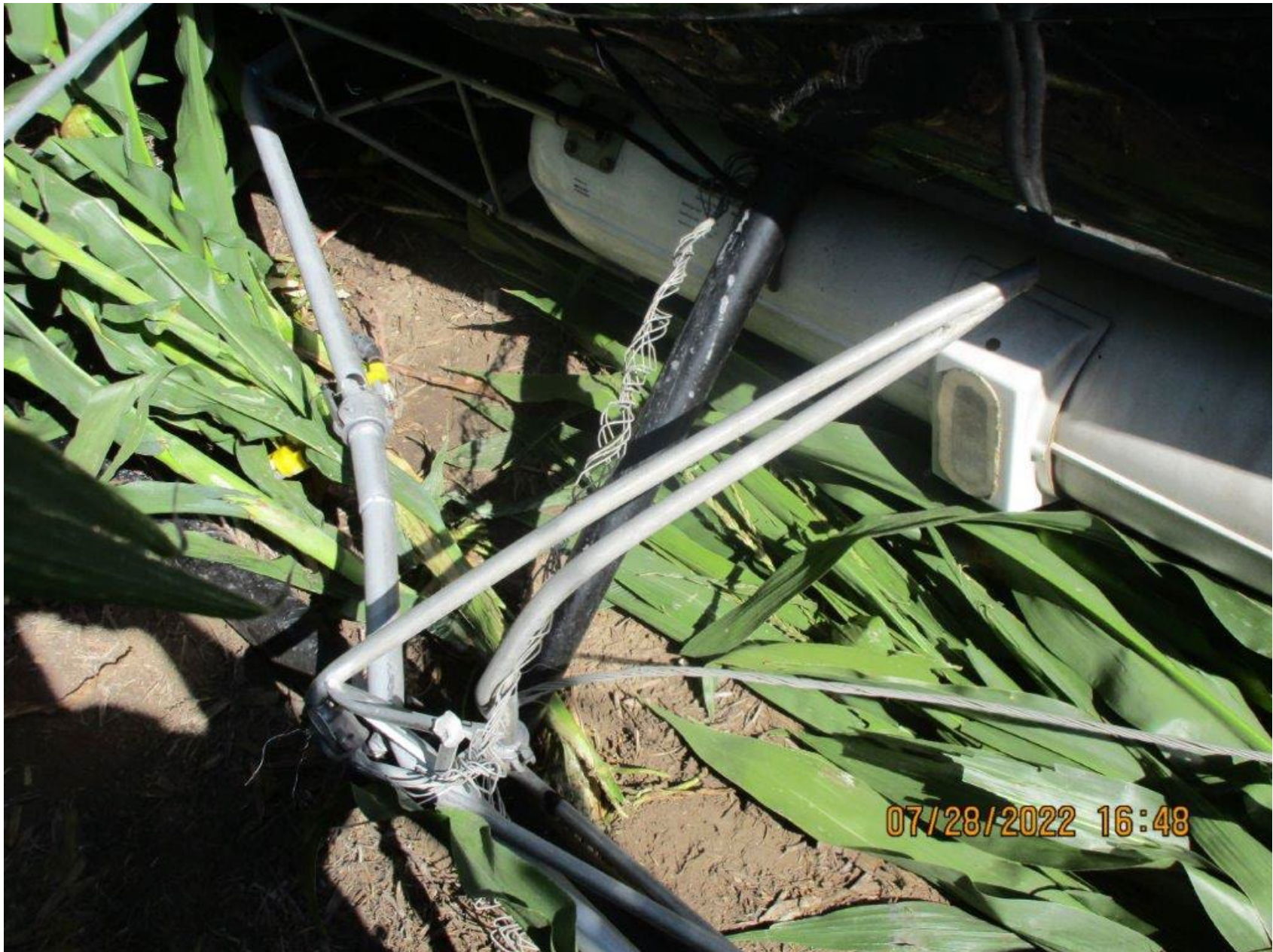
Photo 2 – Remnants of Wire Embedded in Wreckage (Source: FAA)
