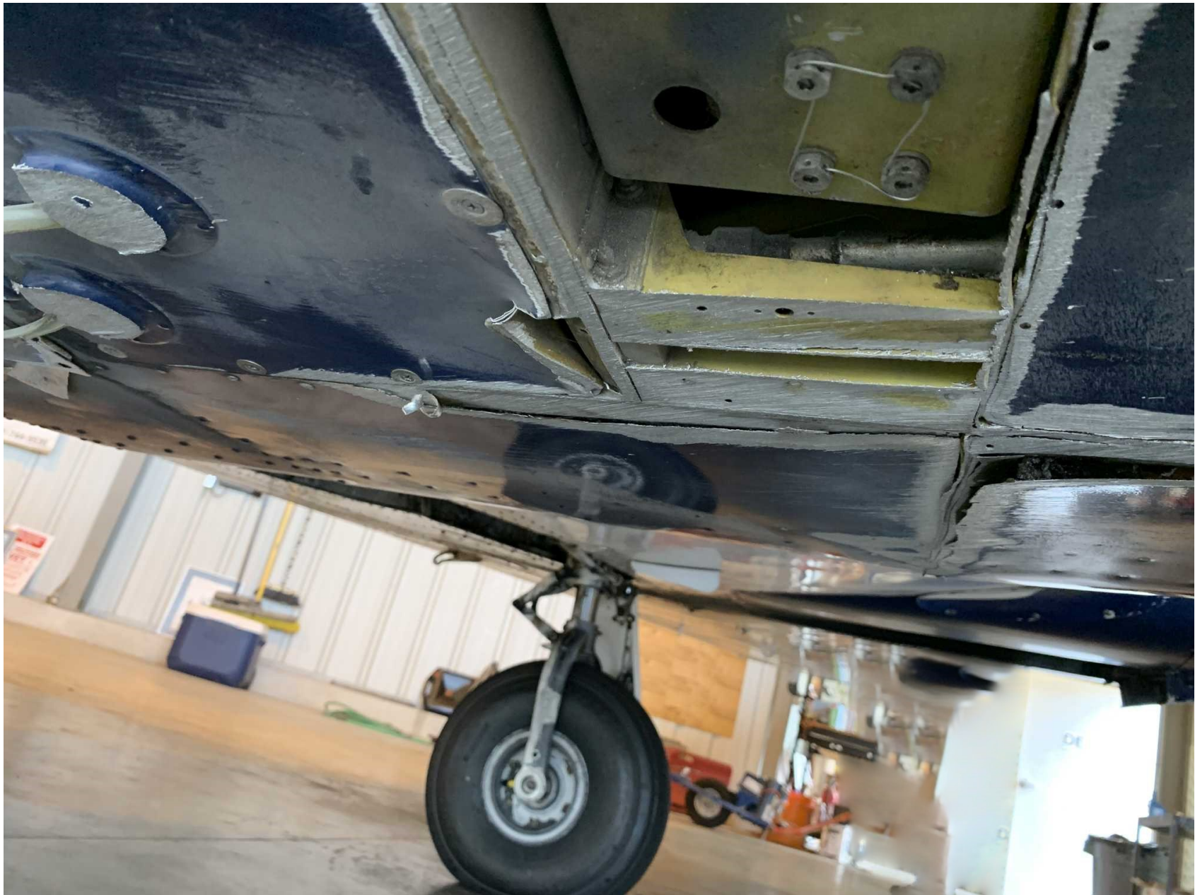
Photo 2 – Structural Damage to Underside of Fuselage (Source: FAA)
