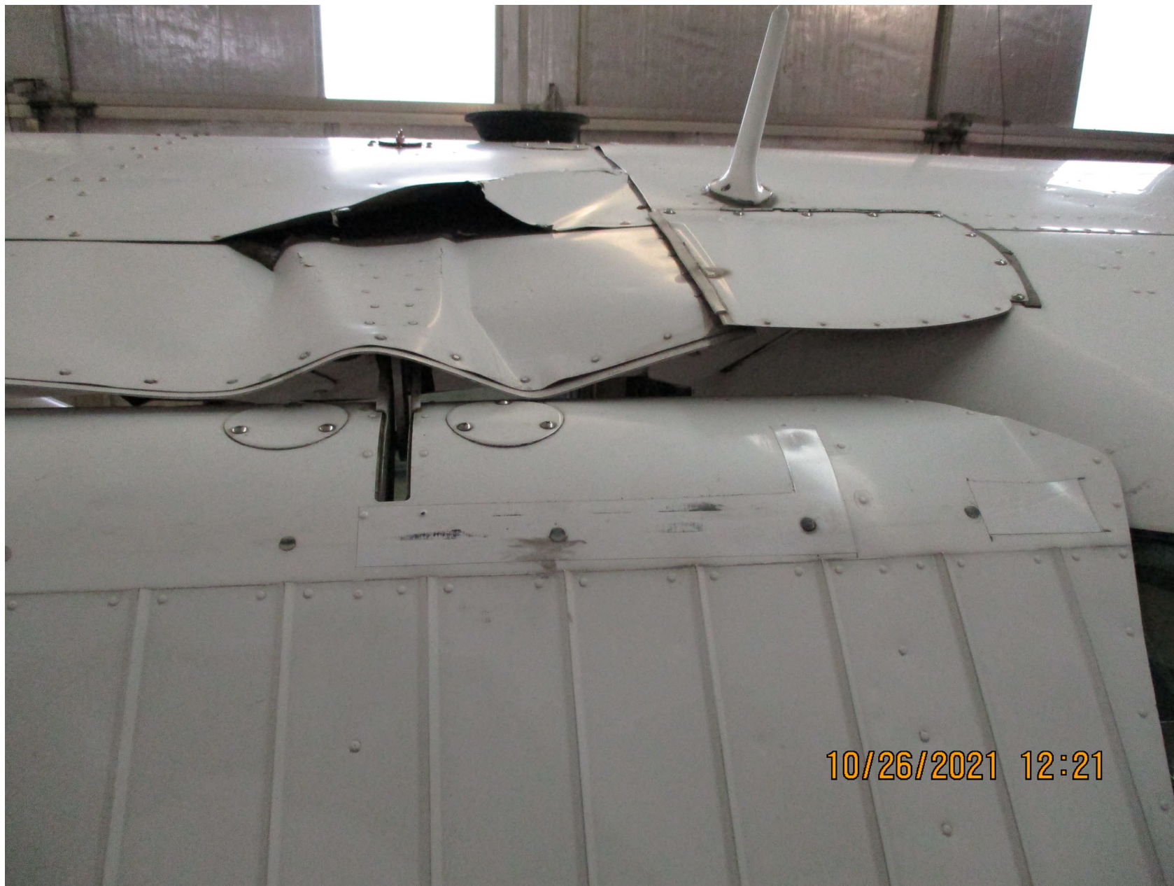
Photo 2 – Closeup of Damage to Left Wing (Source: FAA)
