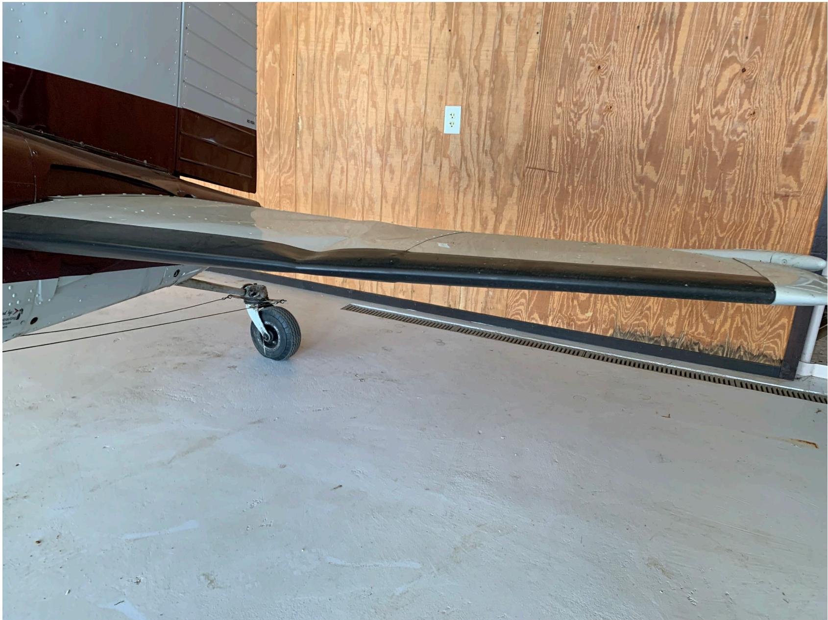
Photo 2 – Left Horizontal Stabilizer Damage (Source: FAA)
