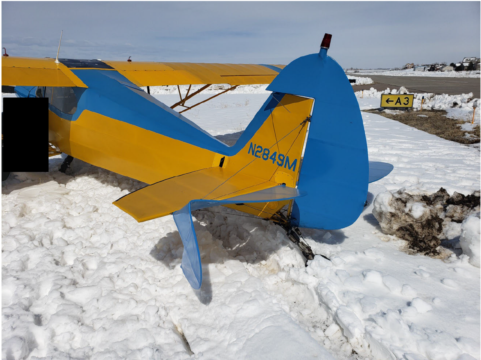
Photo 2 – Left Elevator Damage
