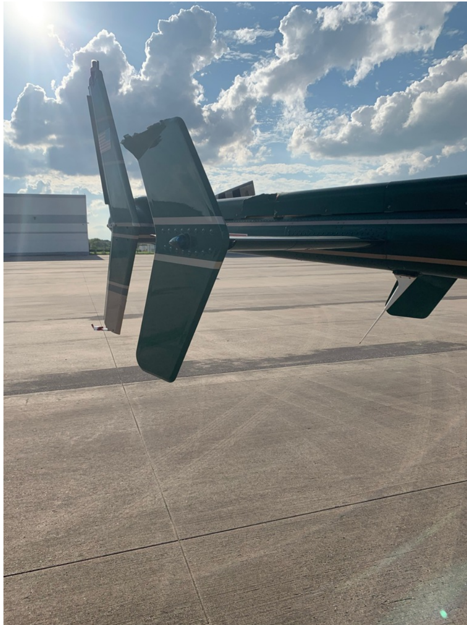
Photo 1 – Substantial Damage to Tailboom
