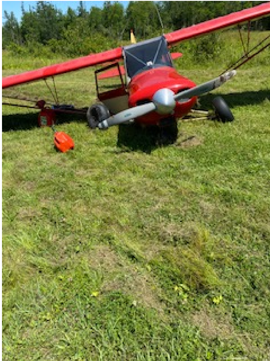
Photo 2 – View of front of airplane showing collapsed main gear
