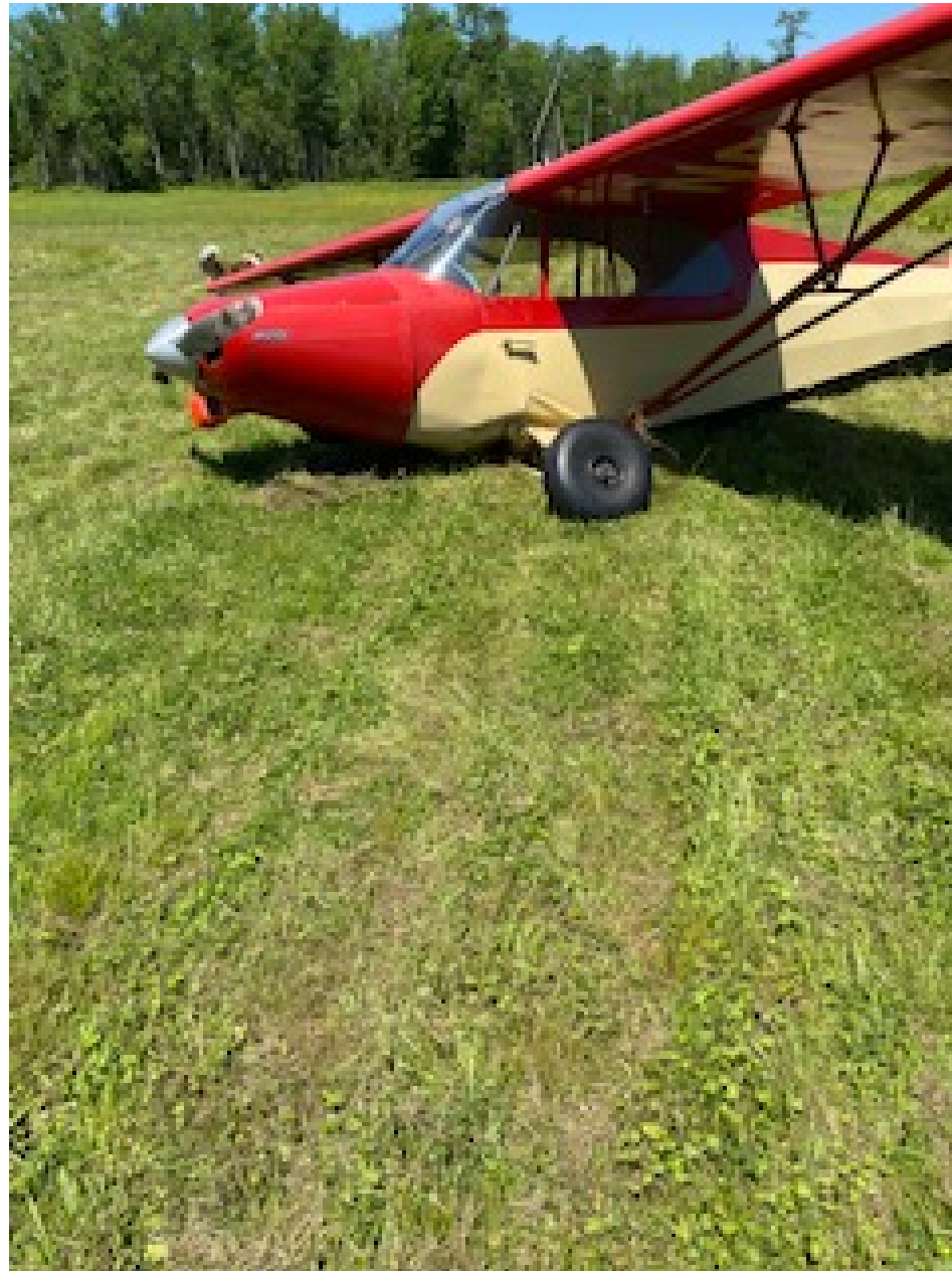
Photo 1 – View of left side showing fuselage buckling
