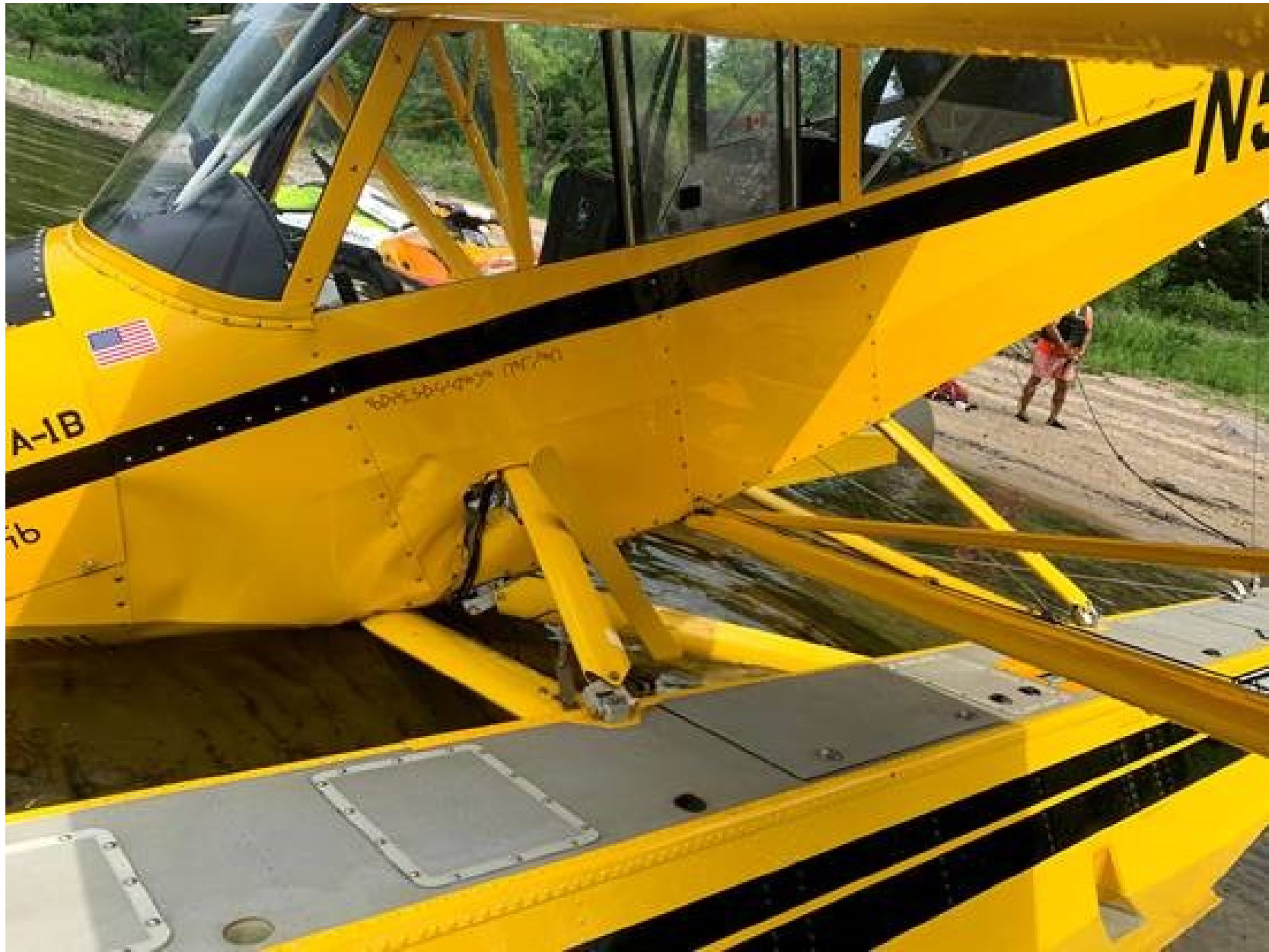
Photo 2 –View of Fuselage Skin Damage (Courtesy of Pilot)
