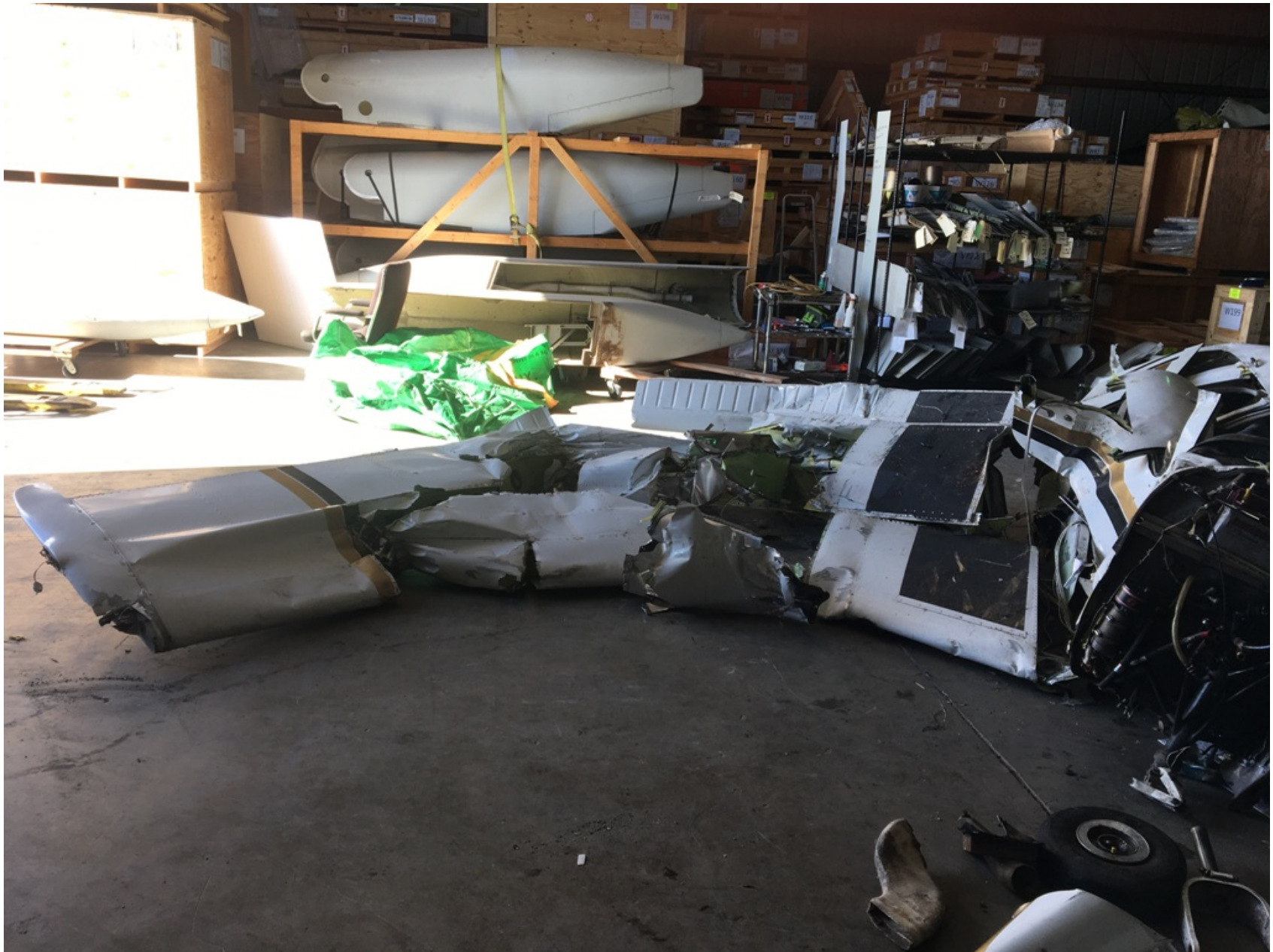
Photo 8 – Right Wing at Salvage Facility
