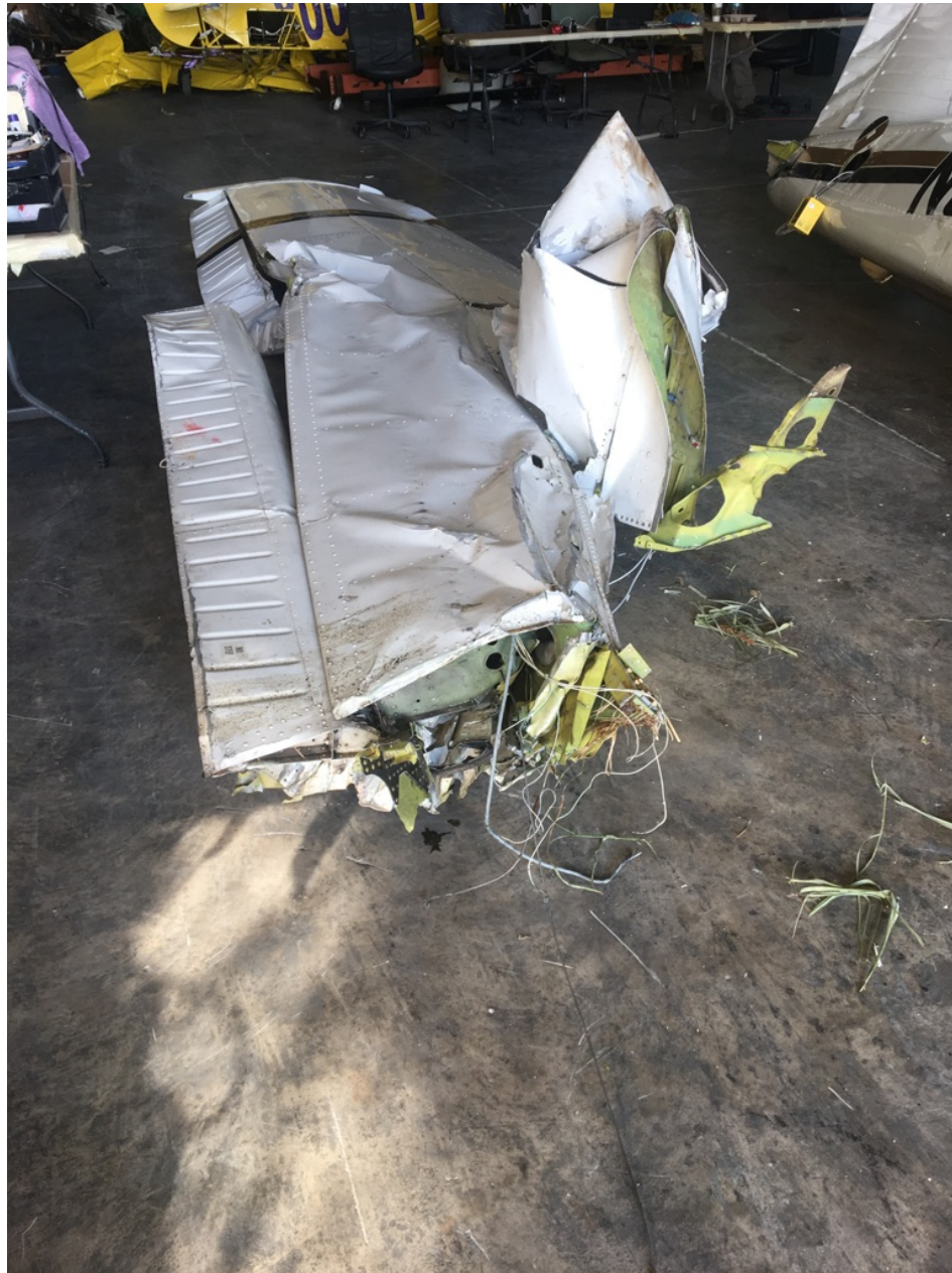
Photo 5 – Horizontal Stabilizer at Wreckage Facility
