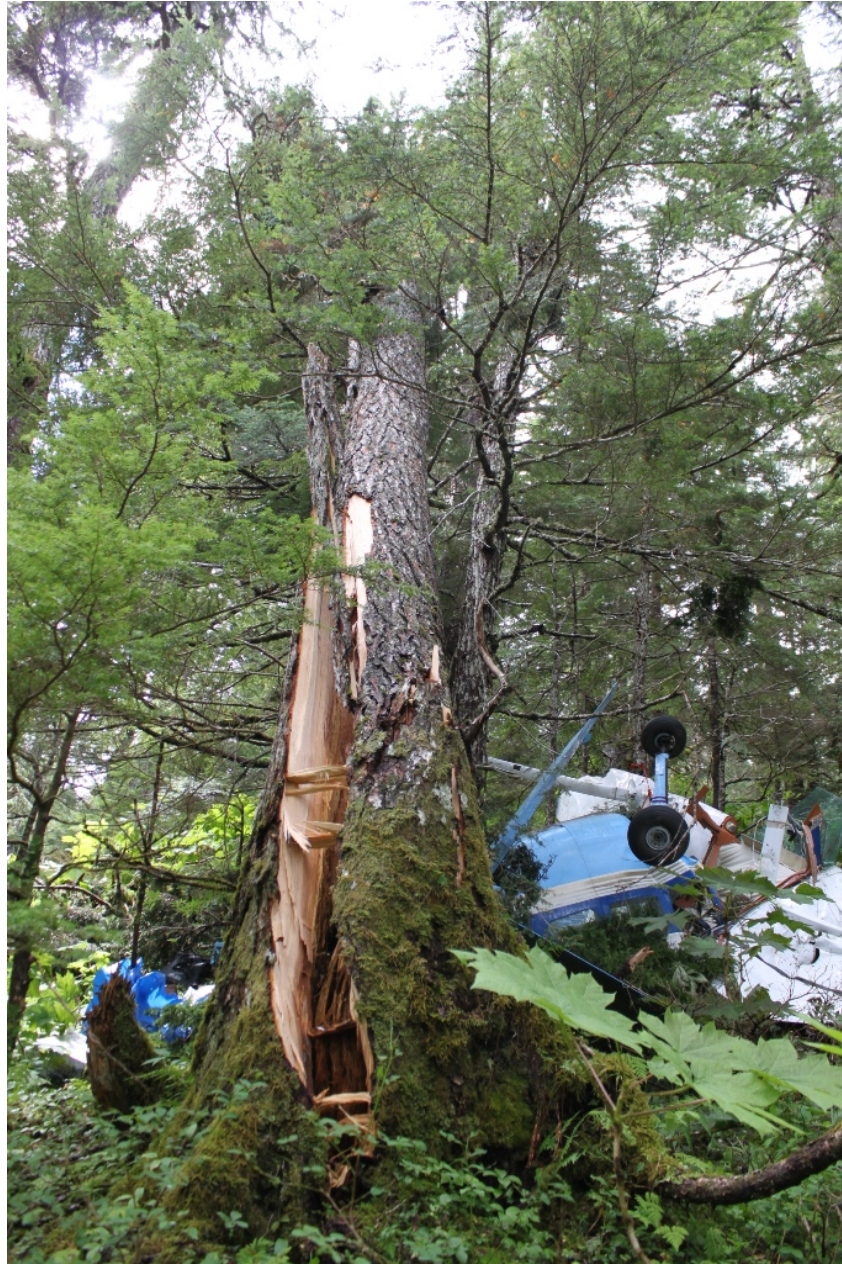
Photo 1 – Main Wreckage at base of tree (Initial Impact)
