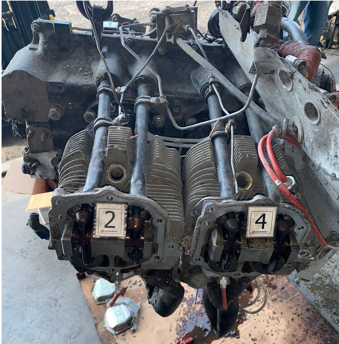
Photo 10: View of engine after removal of valve covers at exam location. (Courtesy of Lycoming)
