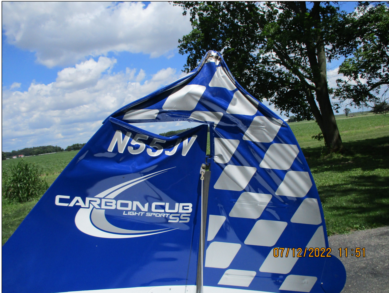
Photo 4: View of the substantial damage sustained to the vertical stabilizer and rudder (Photo Courtesy of FAA)
