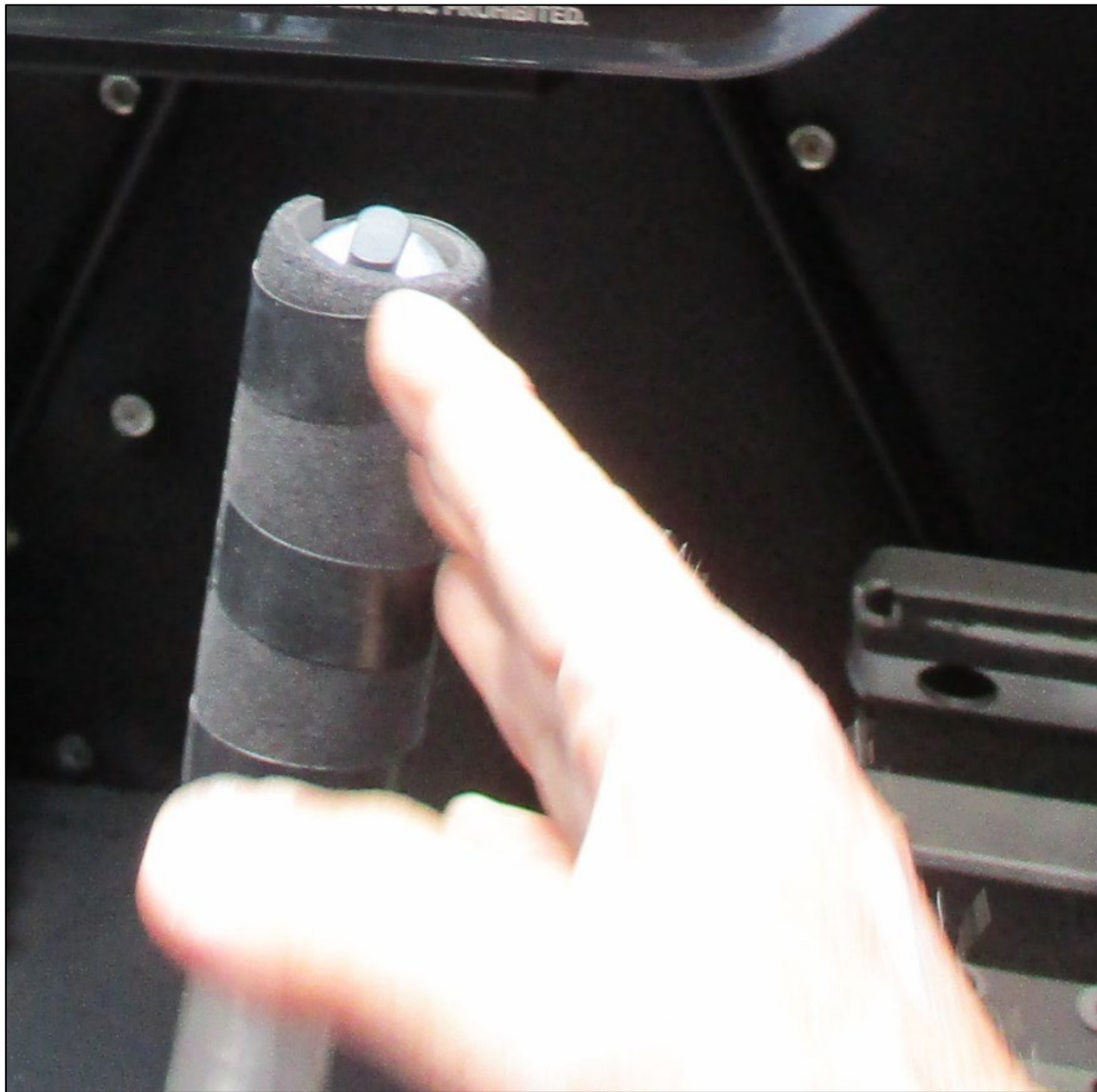
Photo 5: View of the forward seat control stick and rocker trim switch (Photo Courtesy of FAA)
