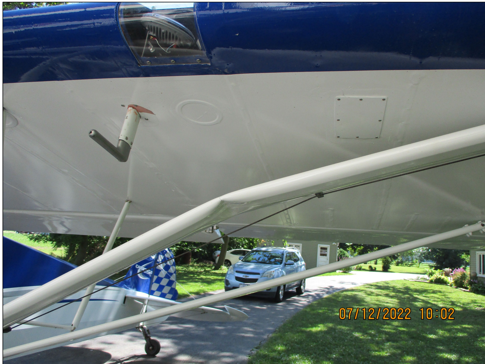
Photo 3: View of the substantial damage sustained to the left wing lift strut (Photo Courtesy of FAA)
