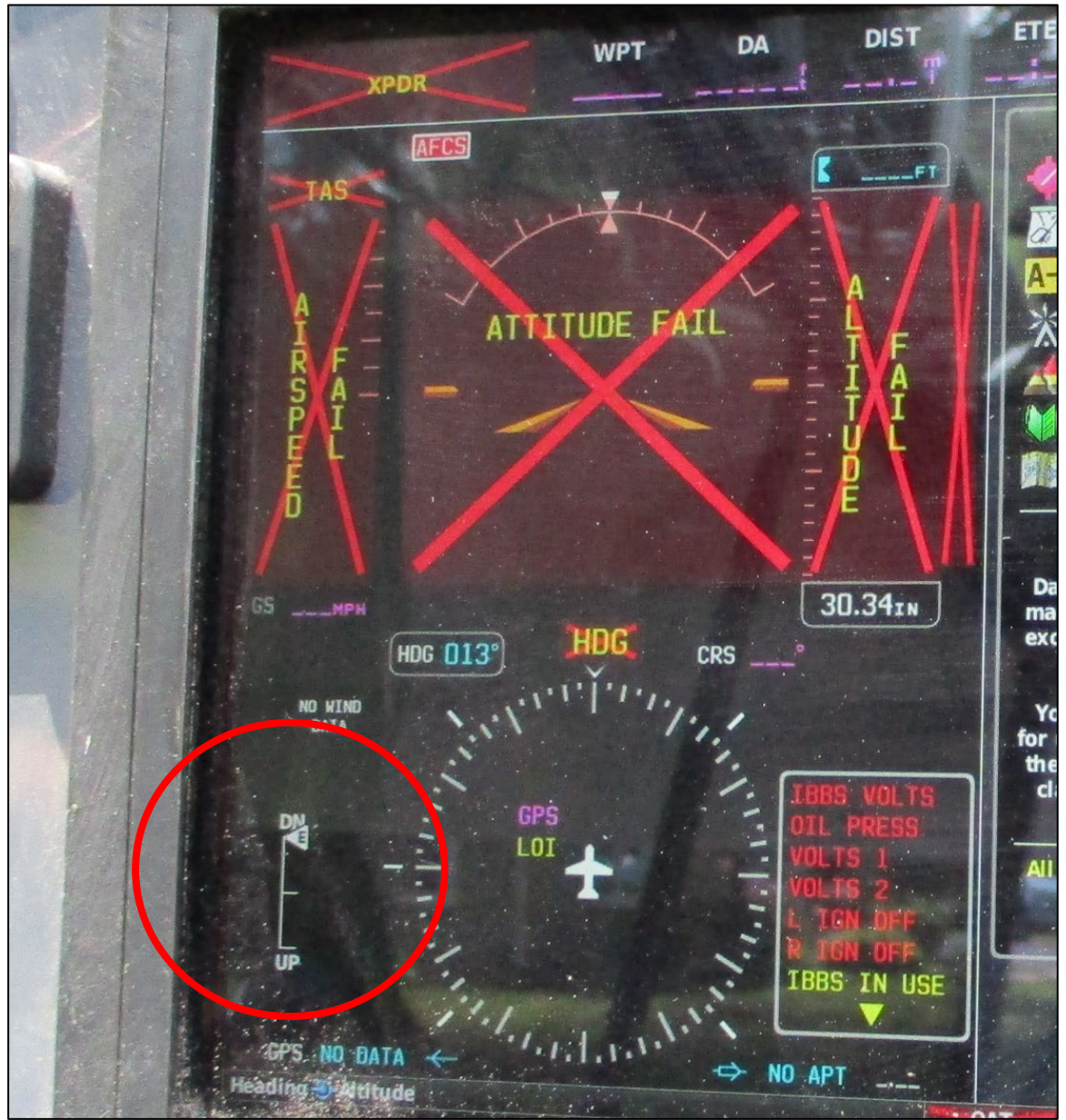
Photo 6: View of the nose UP/DOWN horizontal trim positioned to full nose down (Photo Courtesy of FAA)
