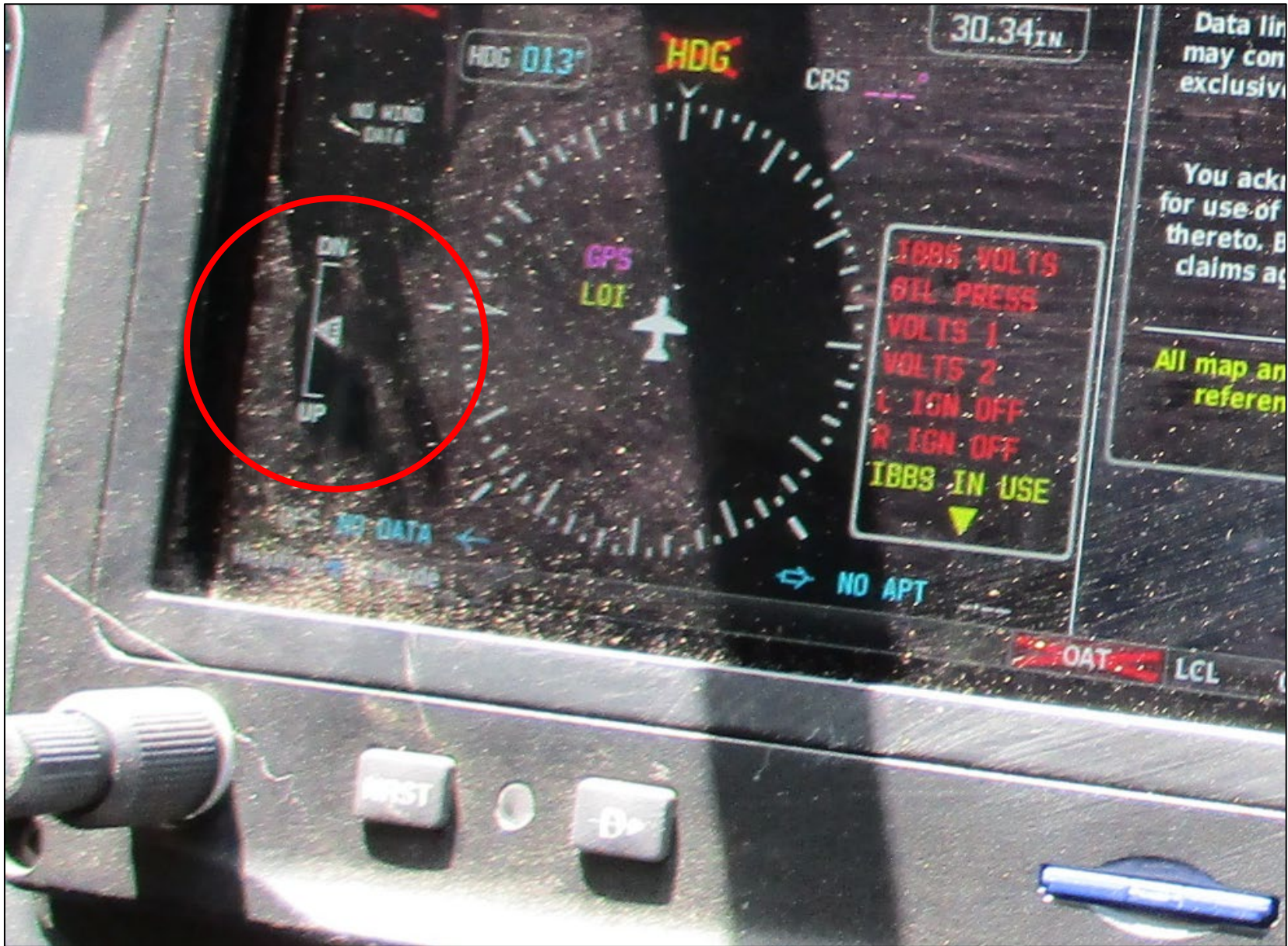
Photo 7: View of the nose UP/DOWN horizontal trim positioned to neutral (Photo Courtesy of FAA)
