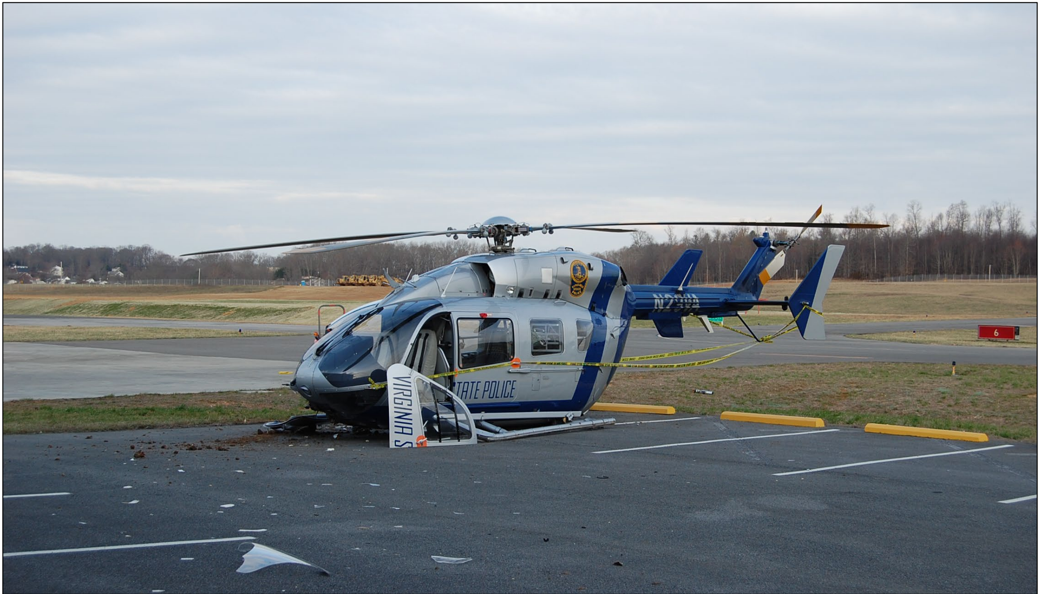
Photo 6: Overview of the helicopter's left side and damaged sustained (Photo Courtesy of Virginia State Police)
